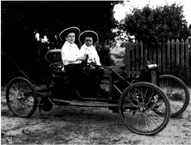
1.7 The 14–16 horsepower four-cylinder Tarrant – the Melbourne-built car that set an Australian 1000-mile (1600-km) speed record in 1905 (copyright Tuckey, B., Australians and Their Cars , Bondi Junction, NSW: Focus, 2003).
