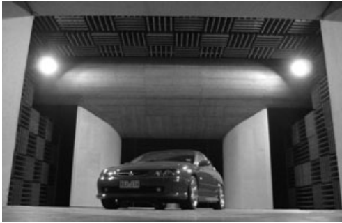
10.6 The open jet test section of an aeroacoustic wind tunnel.
