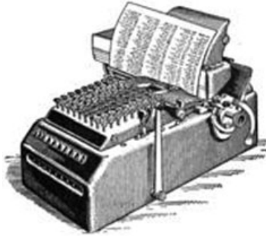
1.10 A mechanical calculator from 1914. Note the lever used to rotate the gears (copyright http://en.wikipedia.org/wiki/History_of_computing_hardware ).
