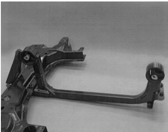
15.18 Example of cantilevered engine mount attachment design (Achram et al. , 1996).
