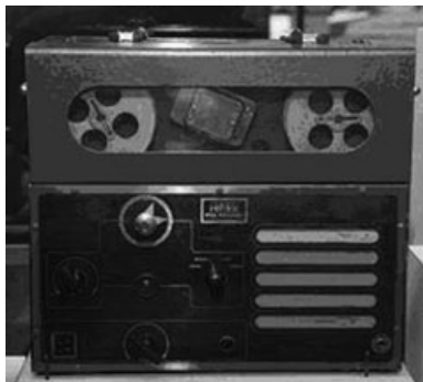
1.8 Peirce 55-B dictation wire recorder from 1945 (copyright http://en.wikipedia.org/wiki/Wire_recorder ).
