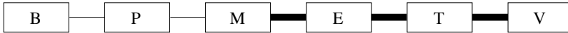
Fig. 4.3. Mild parallel hybrid configuration. B: battery, E: engine, M: motor, P: power converter, T: transmission (including clutch and gears), V: axles and vehicle. Bold lines: mechanical link, solid lines: electrical link.
