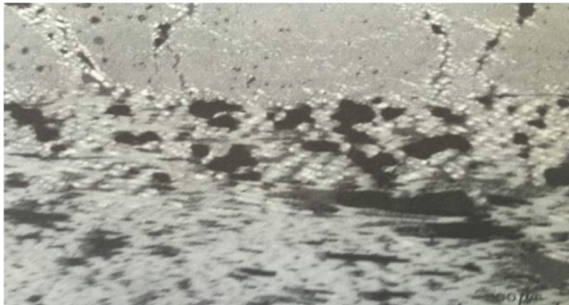
Figure 13.17 Optical micrograph showing a microstructure of C-C composites. Reproduced from Savage, G. (Ed.), 1993. Carbon-Carbon Composites, Chapman & Hall.
