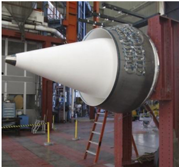
Figure 3.9 This oxide CMC exhaust ground test demonstrator consists of a 1.60-m diameter nozzle and 1.14-m diameter × 2.34-m conical centre body with a titanium end cap inspection portal.
