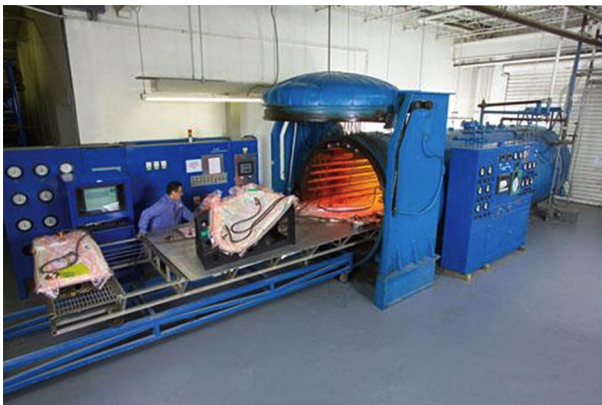
Figure 15.3 Placement of a vacuum-bagged laminated composite part into a large autoclave. Adapted from CompositesWorld. http://www.compositesworld.com/articles/fabrication-methods .
