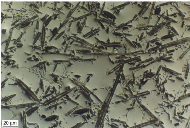
Figure 3.8 Squeeze cast aluminium matrix composite – AA383/Al 2 O 3 /20f. Alumina fibres in the pre-form present a three-dimensional (3D) distribution. Paulo Davim, J., 1997 (Ph.D. thesis).
