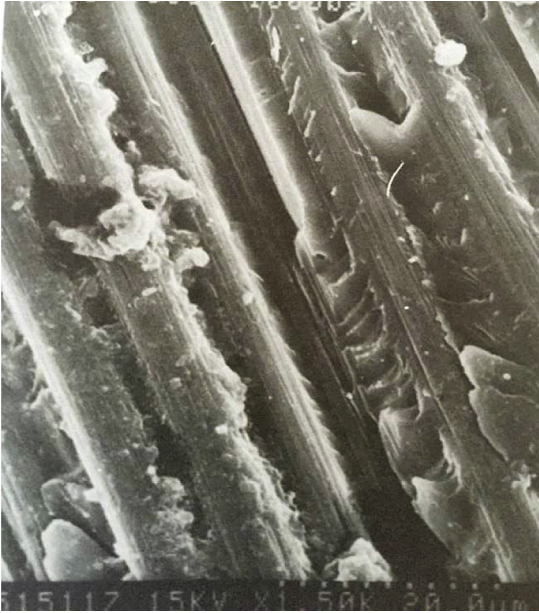
Figure 13.14 C–C composite with PEEK-derived matrix.
