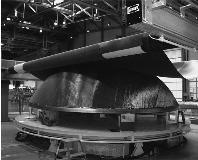
Figure 2.49 Draping of the DOS fabric in the Airbus A380 rear pressure bulkhead production. Adapted from Middendorf, P., Metzner, C., 2011. Aerospace applications of non-crimp fabric composites. In: Lomov, S.V. (Ed.), Non-crimp Fabric Composites , Woodhead, Cambridge, pp. 441–448.
