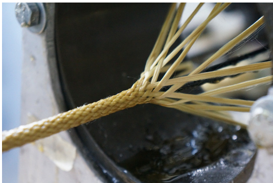
Figure 6.12 Single overlap (diamond)-type braiding pattern being produced.
