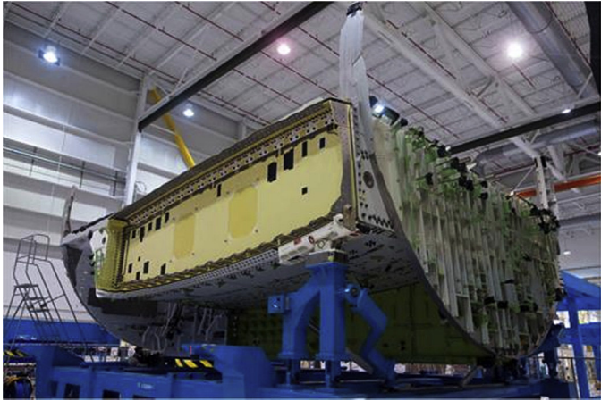
Figure 14.8 Boeing 787 Dreamliner centre wing box before assembly. Reproduced from www.compositesworld.com .
