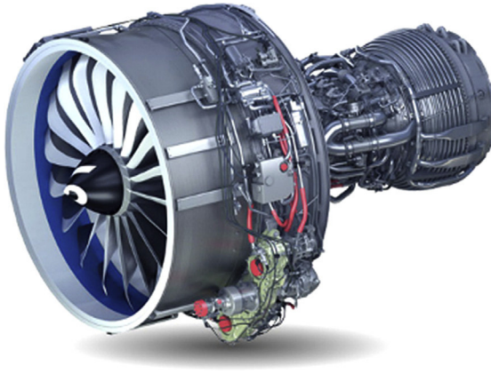
Figure 14.10 CFM Leap Engine featuring CMCs. Reproduced from http://www.cfmaeroengines.com/engines/leap .
