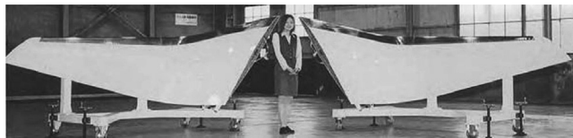
Figure 2.47 Boeing 737–300 winglet programme for Aviation Partners Boeing. Adapted from Lowe, J., 2005. Aerospace applications. In: Long, A.C. (Ed.), Design and Manufacture of Textile Composites, Woodhead, Cambridge, pp. 405–423.
