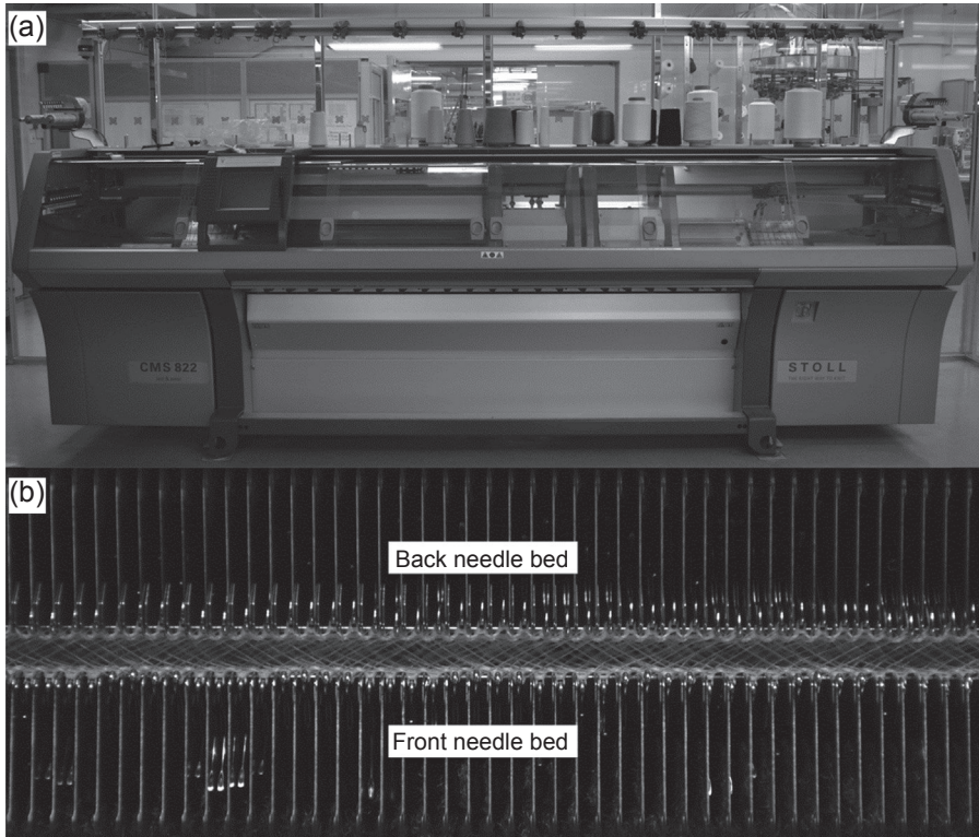
Figure 2.33 Producing a spacer fabric on a computerized flat knitting machine: (a) a Stoll computerized flat knitting machine; (b) knitting a spacer fabric on the flat machine. Adapted from Liu, Y.P., Hu, H., 2015. Three-dimensional Knitted Textiles in Advances in 3D Textiles . Woodhead, Cambridge, pp. 125–152.
