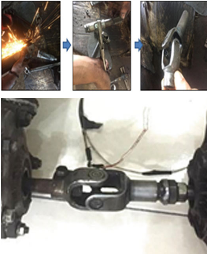
Fig. 14 Preparation of shaft coupling
