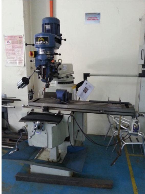
Fig. 2 Milling machine used for FSW
