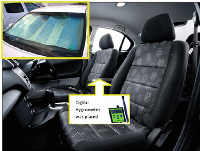
Fig. 1 Position of car sunshade and digital hygrometer inside the car interior
