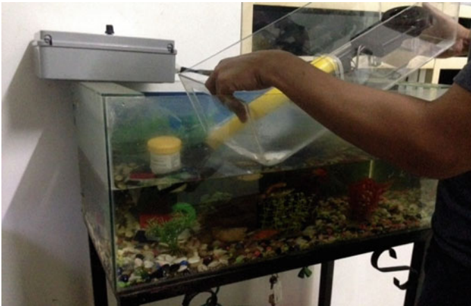
Fig. 9 Underwater 20 g load test
