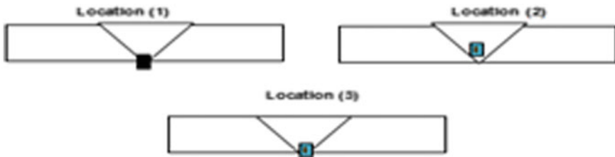
Fig. 4 The scan plan for Specimen 1 after PWHT process. Source Ultrasonic Examination Report by Kejuruteraan Escon Sdn. Bhd
