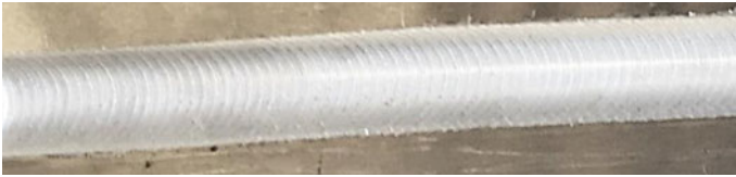
Fig. 6 Welded specimen surface of sample number 4. Smooth welded joint surface; no defects in welded joint (visual inspection); good welded penetration; no flash produced
