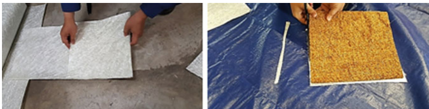
Fig. 4 Kitting process for CSM and coconut fiber
