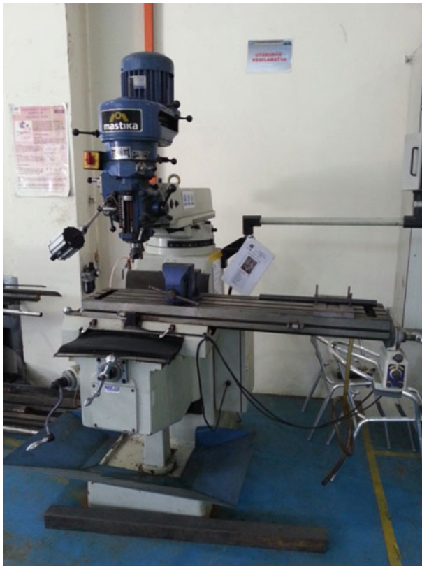
Fig. 2 Milling machine used for FSW
