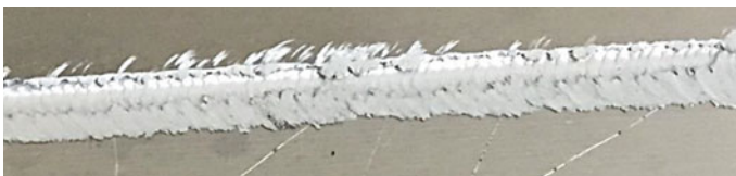
Fig. 3 Welded specimen surface of sample number 1. Poor welded joint surface; severe flash at the side of welded joint; material removal to the side of welded joint; produce wormhole defect along welded joint
