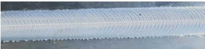
Fig. 7 Welded specimen surface of sample number 5. Smooth welded joint surface; no defects in welded joint (visual inspection); good welded penetration; no flash produced
