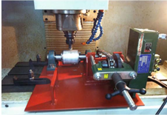
Fig. 1 The FSW jig setup on Bridgeport 2216 CNC milling machine
