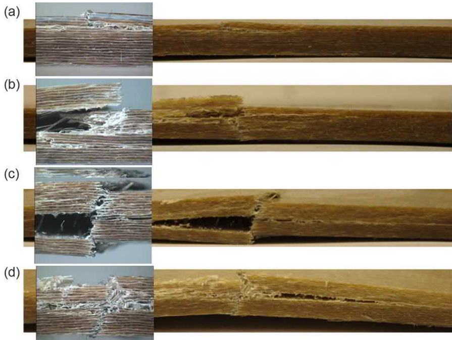
Figure 14.4 Cross-sections of 4.5 mm thick glass fiber reinforced PEI panels following air blast testing [35]. (a) Impulse = 7.9 Ns. (b) Impulse = 8.0 Ns. (c) Impulse = 9.0 Ns. (d) Impulse = 9.4 Ns.
