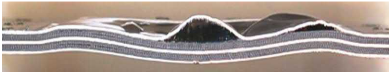
Figure 14.12 Photograph of a cross-section from a GFPP based FML panel subjected to uniformly distributed air-blast loading [76].
