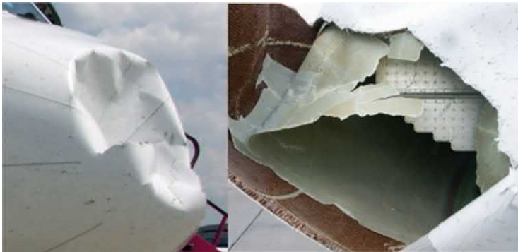
Figure 19.11 “Repaired” bonded structure failure (not considered to be the result of a bird strike) [23].
