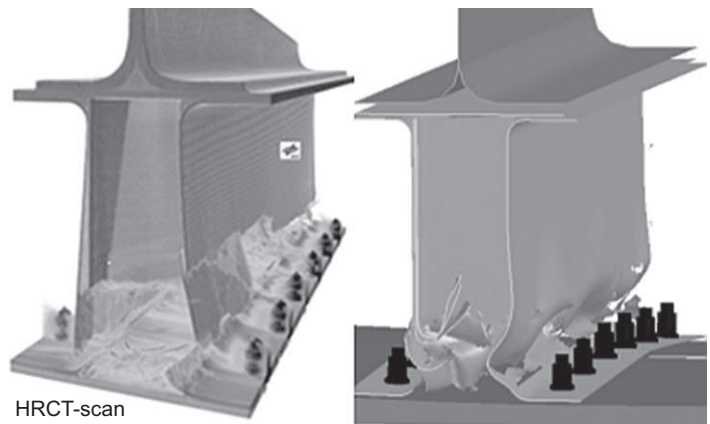
Figure 13.20 Comparison of subfloor damage from high resolution computed tomography scan and finite element simulation of Dynamic 1.
