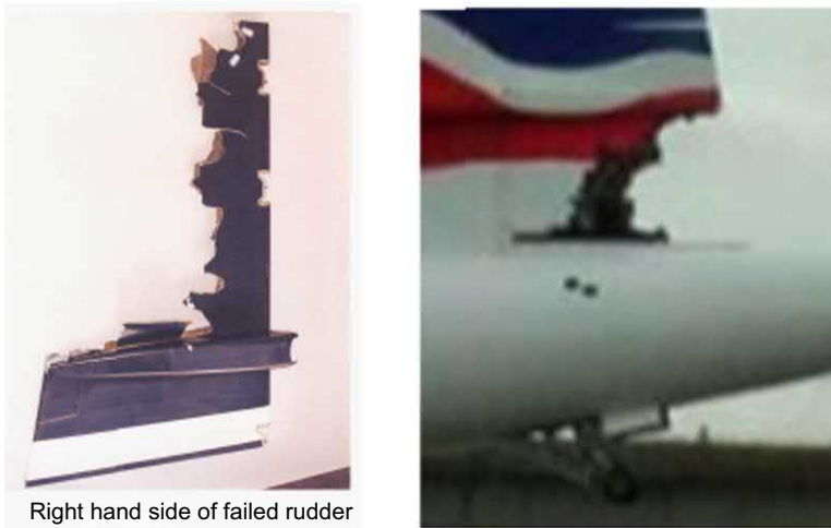
Figure 19.10 (a) Repaired original baseline rudder structure incident. (b) Later rudder structure incident (G-BOAE, 4/12/2002) [18].
