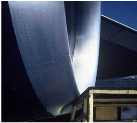
Figure 19.27 Ground crew awareness—engine lowered on to steps as wing deflected during refueling [68].
