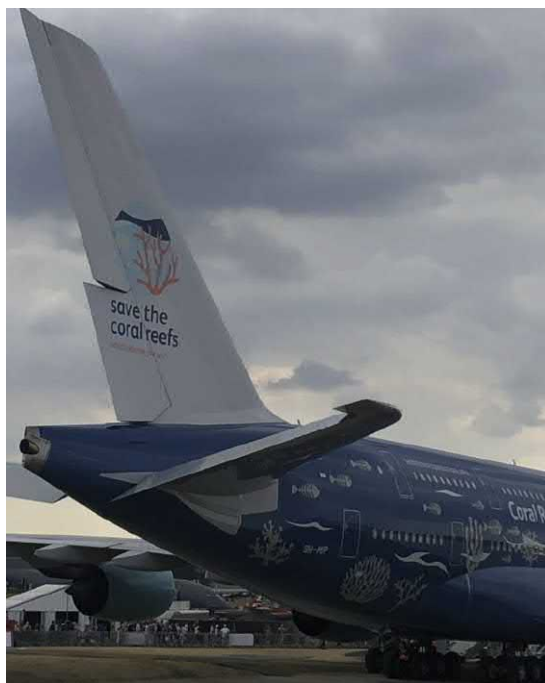
Figure 1.4 A380 all-composite tail assembly (empennage) with Glare fuselage crown. Photo by C. Soutis, Farnborough Air Show, July 2018.
