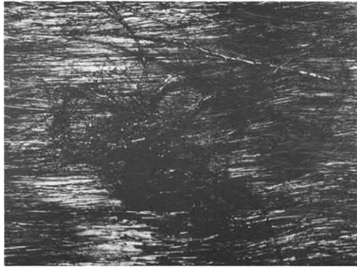
Figure 4.7 A region of entangled fibers in a carbon/epoxy prepreg.
