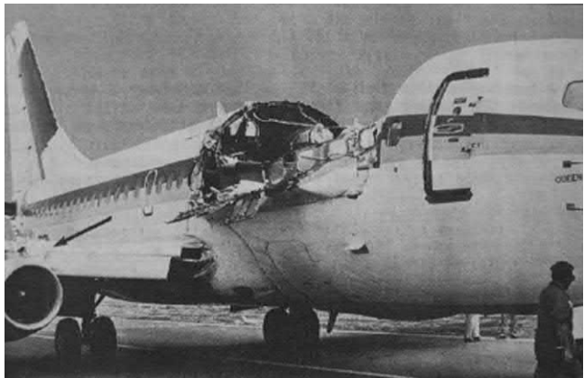
Figure 19.7 Aloha—partially initiated by cold bonded joint failure [15].
