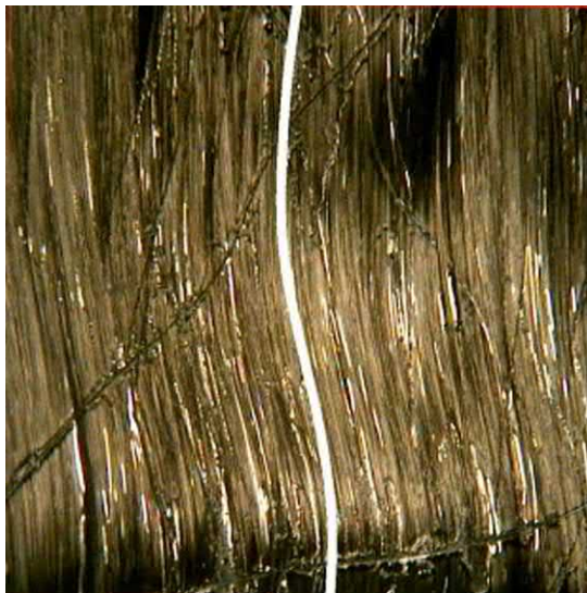
Figure 4.5 Level of fiber misalignment in a typical as-delivered unidirectional prepreg.
