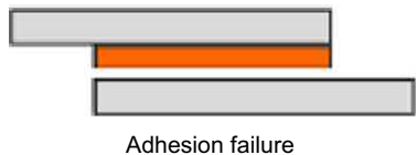
Figure 19.9 Adhesion failure - unacceptable [17].
