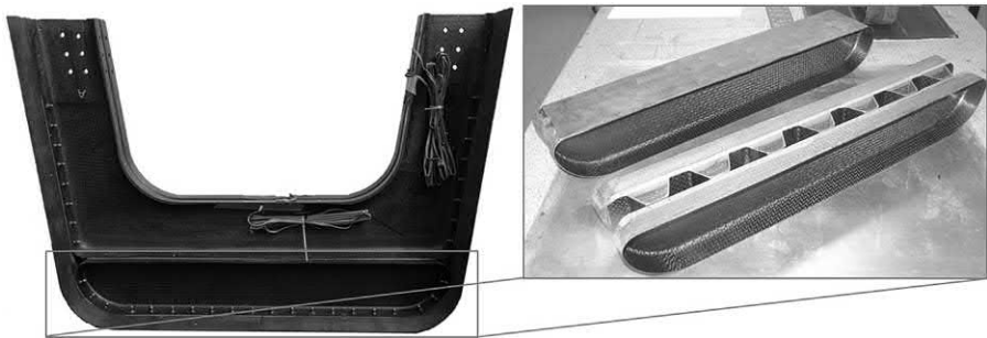
Figure 13.13 As manufactured frame structure with details of energy absorption subfloor.
