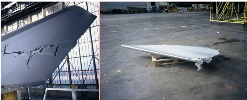
Figure 19.26 Pilot/ground crew wingspan awareness - two passing aircraft winglets collision (one severed) during taxiing (the previous model did not have winglets) ... a potential repair challenge? [68].
