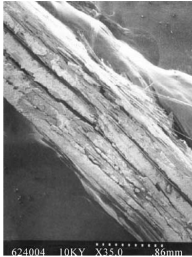
Fig. 4.25. SEM image of fracture side view for 60 wt% of pitch/BN composite annealed at 1,200 °C for 3 h
