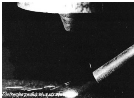
Figure 6.2 A blown powder laser clad being formed
