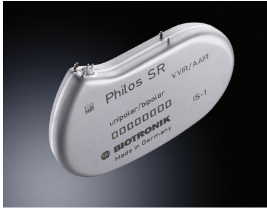
Figure 11.20 A heart pacemaker with a titanium housing that has been hermetically welded using a pulsed Nd:YAG laser. It has also had the contacts inside the housing welded and the housing marked by a pulsed Nd:YAG laser (photo: TRUMPF)
