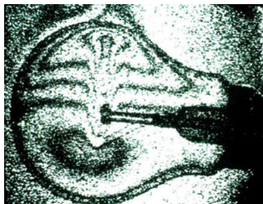
Figure 1.46 A speckle interferogram of an electric light bulb showing the convection currents inside and outside the bulb. (Photo courtesy of J.N. Butters)
