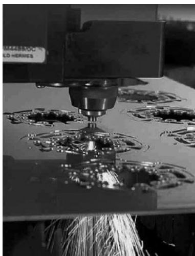
Figure 3.1 Metal cutting of 5-mm-thick stainless steel with a CO 2 slab laser of 2 kW. (Courtesy of AILU through http://www.designforlasermanufacture.com and Rofin-Baasel UK)
