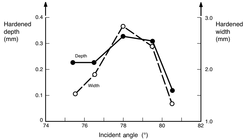
FIGURE 17.9 Variation of depth of hardening with angle of incidence of a p-polarized beam. (From ICALEO 1991 Proceedings , Vol. 74, Copyright 1992, Laser Institute of America. All rights reserved.)
