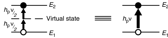
FIGURE 1.10 The two-photon absorption concept.
