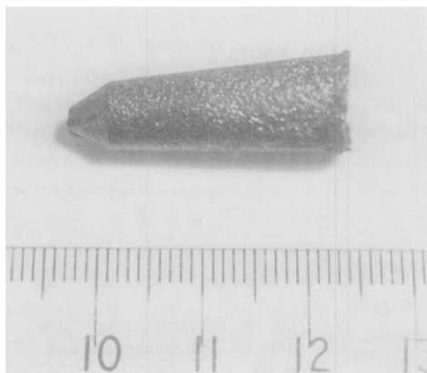
Fig 7. Boule of PrAg grown by the Bridgman technique (1 div. = 1 mm).
