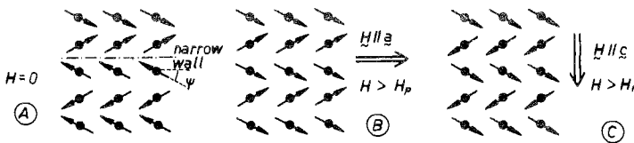
Fig. 14.123. (A): Schematic representation of the magnetic structure and domain configuration in Tb_{0.5}Y_{0.5}Ni . (B): Effect of a field applied parallel to the ferromagnetic direction a . (C): Effect of a field applied parallel to the antiferromagnetic direction c : magnetization reversal of one sublattice (Gignoux and Lemaire, 1974).
