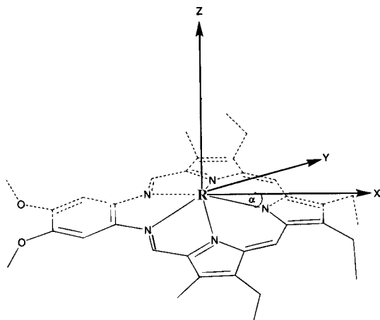
Fig. 4. Structure and reference frame for the dimethoxy tetraethyl dimethyl trivalent lanthanide texaphyrin. The \alpha angle measures the out-of-plane location of R(\text{III}) with respect to the mean macrocyclic plane (adapted from Lisowski et al. (1995a)).
