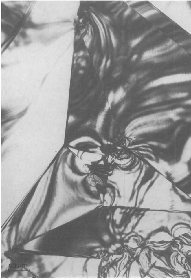
Fig. 49. Star feature of domains formed by phase transformation in B\text{-Sm}_2\text{O}_3 occurring when three domains related by a rotation of 2\pi/3 meet.
