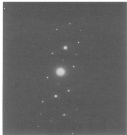
Fig. 11. Electron diffraction pattern of a GdBi film after heating at high temperature. The spot system corresponds to a fcc cell with a = 6.36 \text{ \AA} .
