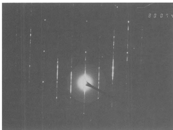
Fig. 18. Complex electron diffraction pattern corresponding to a polytypic syntactic intergrowth (the circle is the projection of the diameter of the aperture).
