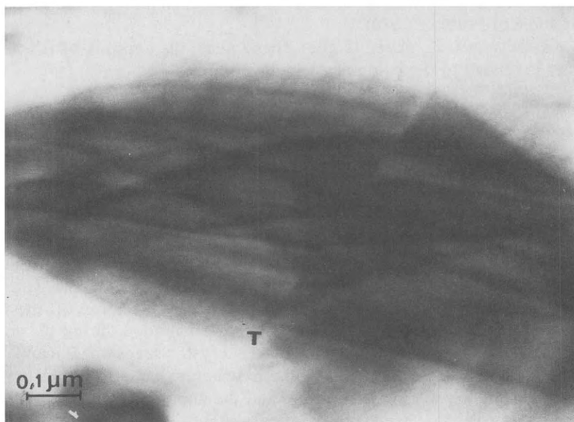
Fig. 55. High magnification image of a twin (T) of a C-Dy 2 O 3 crystal visible by using the fine structure of a \langle 111 \rangle zone axis pattern.
