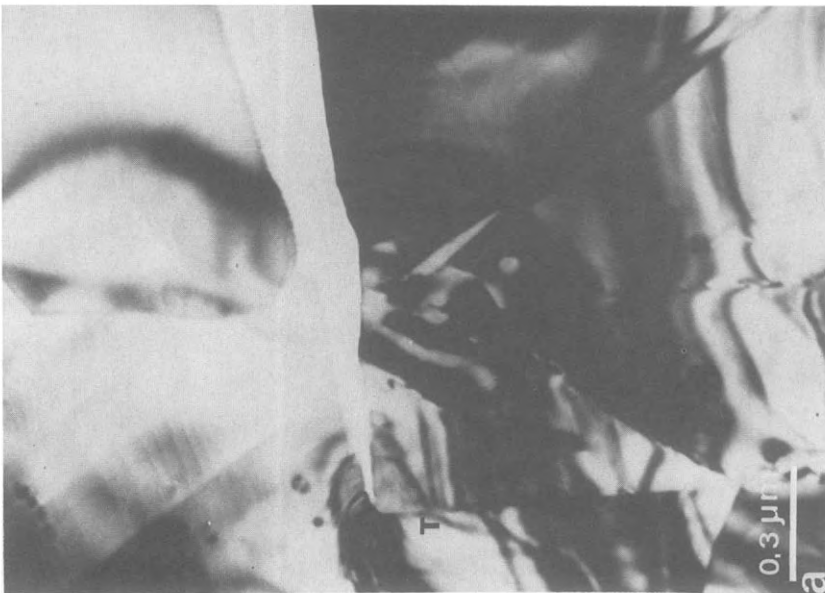
Fig. 15. (a) Mechanical twin (T) at the tip of a fracture in a B-Sm 2 O 3 crystal.
