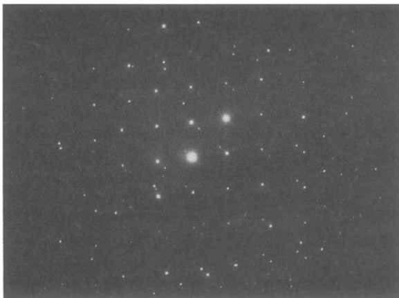
Fig. 24. Electron diffraction pattern of a large crystal obtained after annealing of a GdGa film. The two spots in the vicinity of the central spot do not correspond to the B- \text{Gd}_2\text{O}_3 structure.
