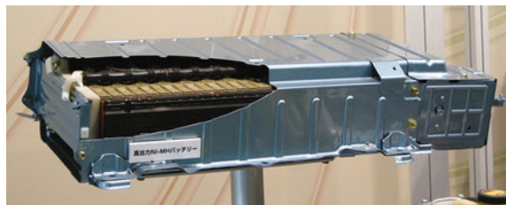
Fig. 7.6 Rechargeable NiMH battery for a Toyota Prius. Source Wikimedia commons. Original Photograph by Hatsukari715
