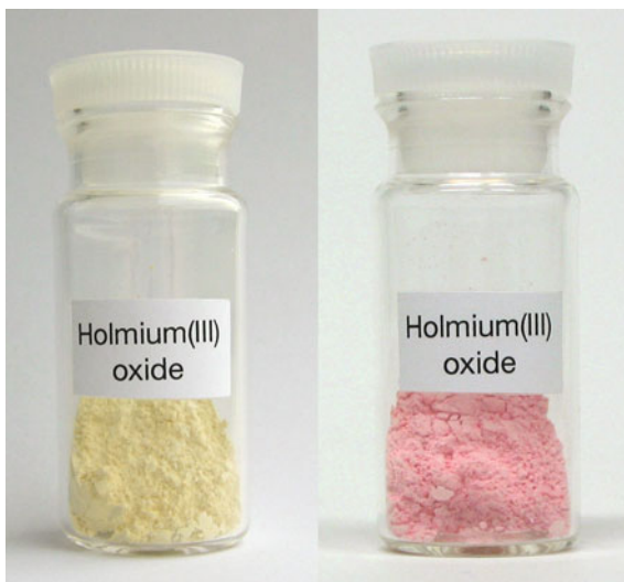
Fig. 5.7 Holmium(III) oxide. Left natural light, right fluorescent-lamp light. File from Wikimedia Commons, the free media repository. Licensed under CC BY 3.0 via Wikimedia Commons. http://commons.wikimedia.org/wiki/File:Holmium(III)_oxide.jpg . Original file uploaded by Filousoph
