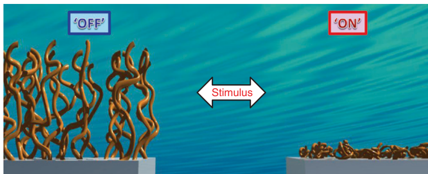
Fig. 4.1 Schematic illustration of phase transition behavior for a smart polymer-grafted surface
