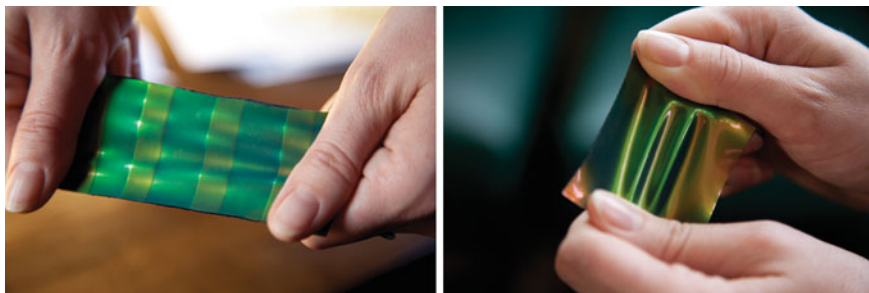
Fig. 2.26 Polymer opal gradually turns to blue when stretched and returns to its original color, in this case green . Courtesy University of Cambridge
