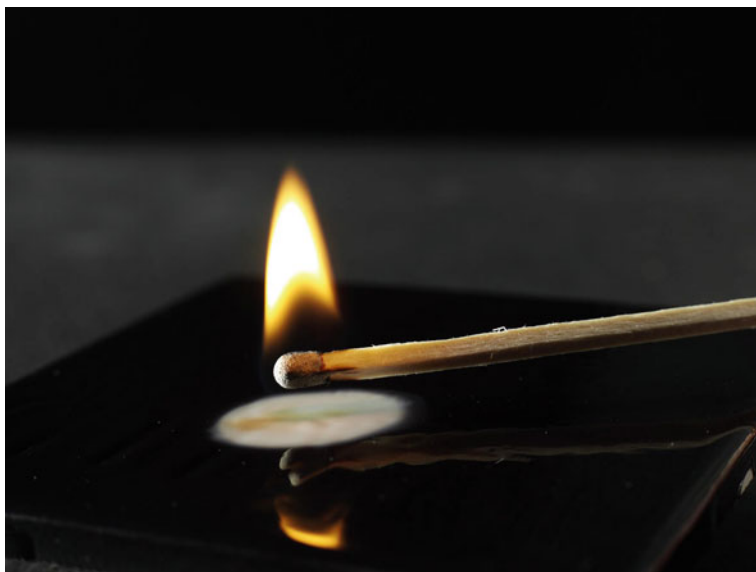
Fig. 2.3 A drop of Alsa thermochromic ink reacts to the heat generated by a match. Courtesy of Alsa Corporation
