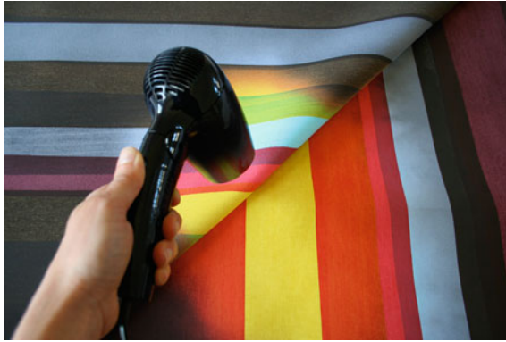
Fig. 2.11 Linda Worbin, Graffiti Cloth (picture from her PhD thesis). The textile combines three types of sensitive thermochromic pigments with conventional ones to explore the changes that occur when hot air flows. By using the overprint technique three more colors are added which become visible in the heated stage of the fabric. Some colors change from one to another while some colors stay in their initial state
