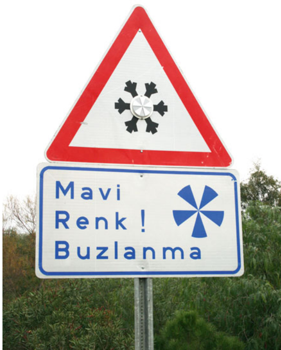
Fig. 2.13 Road sign showing risk of icing on a Turkish highway: “blue color indicates icing”—the snow flake turns to blue under -1\text{ }^{\circ}\text{C} indicating icy road surface (photo by Murat Bengisu)
