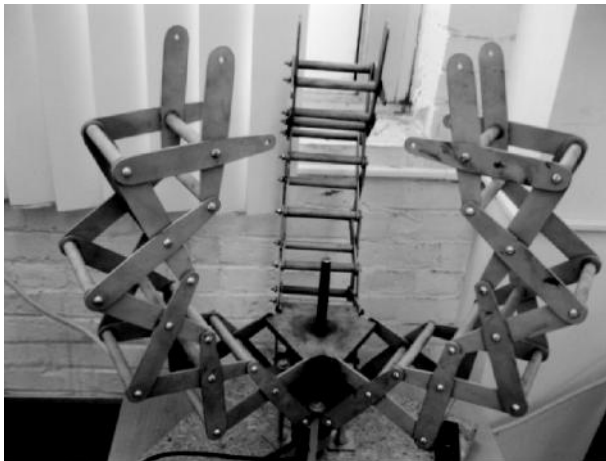
Figure 4.26 An experimental model for a three-finger robotic grabber based on an SLE in deployed mode.
