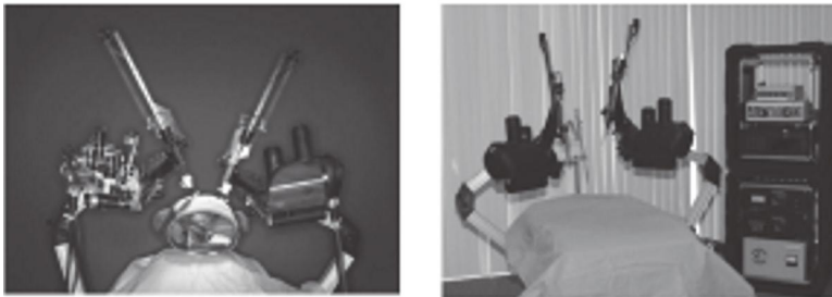
Figure 1.2 The RAVEN surgical robot. (a) SolidWorks models and (b) arms in practice.
