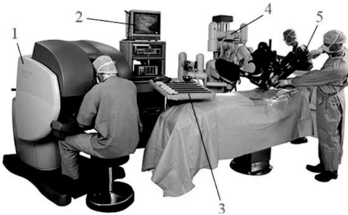
Figure 4.7 The da Vinci® robotic surgical system main units. (1) A surgeon console, (2) image-processing equipment, (3) EndoWrist® instruments, (4) a surgical arm cart, and (5) a high-resolution 3D endoscope.
