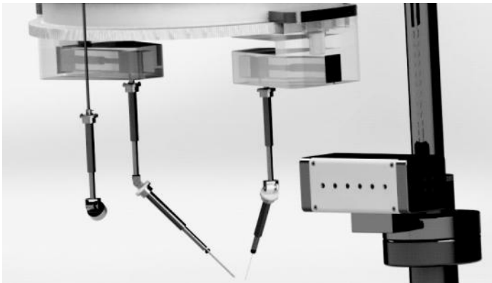
Figure 3.12 The proposed robotic surgical system; a closer view of the robotic manipulators.
