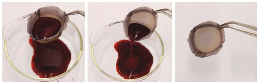
Figure 8.21 Heparinized blood was incubated for 6 h in a superamphiphobic well and removed afterwards by tilting. Macmillan Publishers Ltd., Nature Publishing Group: M. Paven, et al. , Super liquid-repellent gas membranes for carbon dioxide capture and heart-lung machines, Nat. Commun. , 2013, 4, copyright 2013.
