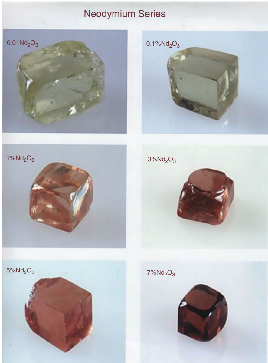
Fig. 1.1 Samples of 80\text{TeO}_2\text{-}5\text{TiO}_2\text{-(}15\text{-}x\text{)WO}_3\text{-}x\text{A}_n\text{O}_m where \text{A}_n\text{O}_m is \text{Nb}_2\text{O}_5 , \text{Nd}_2\text{O}_3 , and \text{Er}_2\text{O}_3 ; x = 0.01, 1, 3, \text{ and } 5 mol% for \text{Nb}_2\text{O}_5 ; and x = 0.01, 0.1, 1, 3, 5, \text{ and } 7 mol% for \text{Nd}_2\text{O}_3 and \text{Er}_2\text{O}_3
