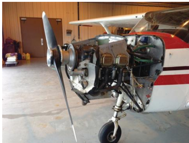
■ FIGURE 5.14 Integration of a Lycoming O-320 air-cooled engine in a Cessna 172 aircraft
