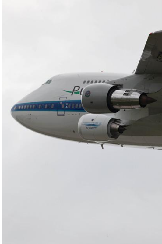
■ FIGURE 11.17 PW1133G first flight on P&W B747SP Flying Test Bed. Source: Reproduced by permission of United Technologies Corporation, Pratt & Whitney
