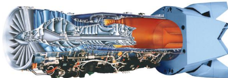
■ FIGURE 3.33 F119 engine cutaway. Source: Reproduced by permission of United Technologies Corporation, Pratt & Whitney
