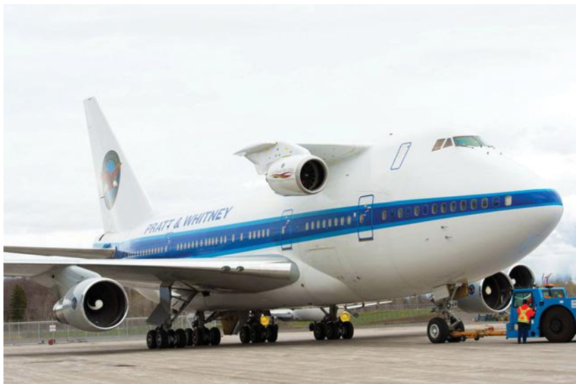
■ FIGURE 11.16 PW1217G flight testing on one of the two P&W B747SP Flying Test Beds. Source: Reproduced by permission of United Technologies Corporation, Pratt & Whitney
