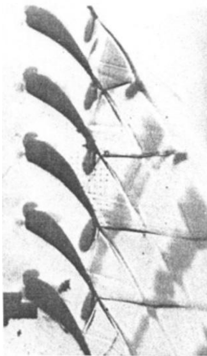
■ FIGURE 10.15 Schlieren photograph of a turbine nozzle cascade showing expansion waves and shock formations downstream of an uncooled turbine nozzle. Source: Gostelow 1984. Reproduced with permission from Elsevier
