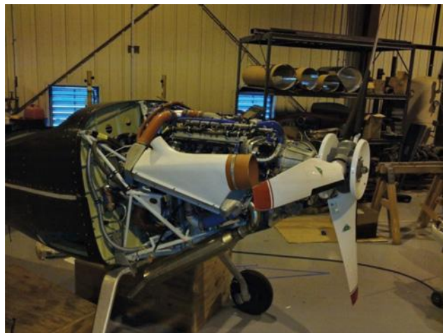
■ FIGURE 5.4 Thielert aircraft diesel engine installed on Meridian UAV
