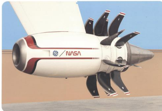
■ FIGURE 1.18 GE Unducted Fan (UDF) or GE-36. Source: Reproduced with permission from General Electric Company
