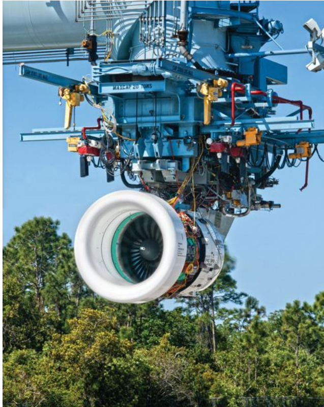
■ FIGURE 11.14 PW1524G engine in ground testing at the Pratt & Whitney West Palm Beach, FL, test facility. Source: Reproduced by permission of United Technologies Corporation, Pratt & Whitney
