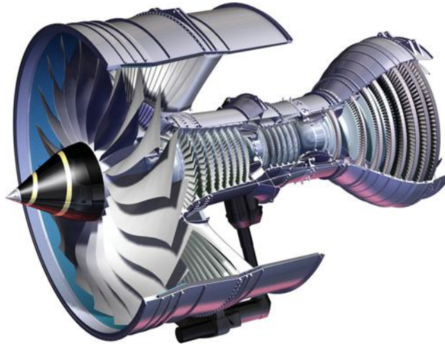
■ FIGURE 1.9 Three-spool gas turbine engine as developed by Rolls-Royce. Source: The Jet Engine , 2005. Reproduced by permission from The Jet Engine , Copyright Rolls-Royce plc 2005
