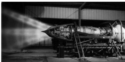
■ FIGURE 1.15 F119 engine that powers F-22 Raptor is shown in vector thrust. Source: Reproduced with permission of United Technologies Corporation, Pratt & Whitney
