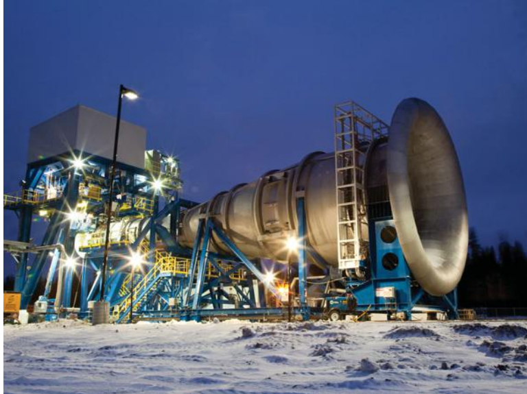
■ FIGURE 11.15 PW1524G engine conducting natural icing tests at the GLACIER facility in Thompson, Manitoba, Canada. Source: Reproduced by permission of United Technologies Corporation, Pratt & Whitney
