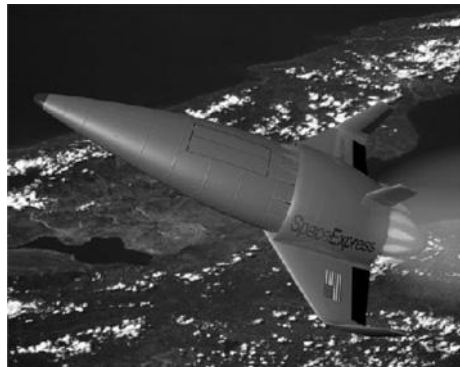
■ FIGURE 1.28 Artist's drawing of an advanced launch vehicle using RBCC propulsion. Source: Courtesy of NASA
