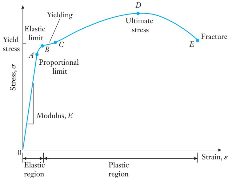
line in the stress–strain diagram. Our conclusion from such experiments is that while the stiffness depends on the rod’s dimensions, the stress–strain relationship is a property of the material alone and is independent of the test specimen’s size.
