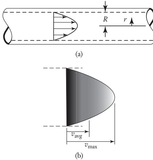
occurs at the pipe's centerline, and it depends on the pressure drop, the pipe's diameter  $d = 2R$ , the fluid's viscosity  $\mu$ , and the pipe's length  $L$ . Engineers will typically specify the diameter of a pipe, rather than its radius, because the diameter is easier to measure. The term  $\Delta p/L$  in Equation (6.8) is interpreted as the drop in pressure that occurs per unit length of the pipe.
