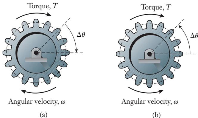
where the angle  $\Delta\theta$  again has the dimensions of radians. As is the case for the work of a force, the sign of  $W$  depends on whether the torque tends to reinforce the rotation (in which case  $W$  is positive) or oppose it (and  $W$  is negative). Those two situations are shown in Figure 8.5. Engineering units for work are summarized in Table 7.1. Two particularly useful conversion factors for calculations involving geartrains and belt drives are
