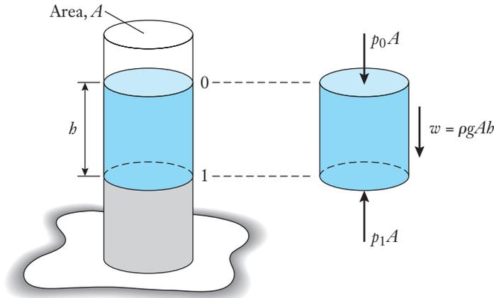
liquid or gas increases with depth. Referring to the beaker of liquid shown in Figure 6.10, the difference in pressure  $p$  between levels 0 and 1 arises because of the intervening liquid's weight. With the two levels separated by depth  $b$ , the weight of the liquid column is  $w = \rho g A b$ , where  $A b$  is the enclosed volume. By using the free body diagram of Figure 6.10, the equilibrium-force balance of the liquid column shows that the pressure at depth 1 is
