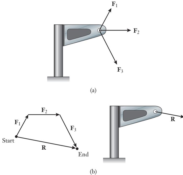
engineer first needs to determine their net effect. With  $N$  individual forces  $\mathbf{F}_i$  ( $i = 1, 2, \dots, N$ ) being present, they are summed according to
