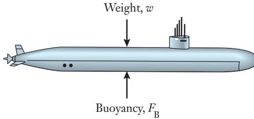
fluid. As shown in Figure 6.11, when a submarine is submerged and floating at a steady depth, the net force on it is zero since the (upward) buoyancy force balances the submarine's weight. The buoyancy force  $F_B$  equals the weight of fluid displaced by an object according to the equation
