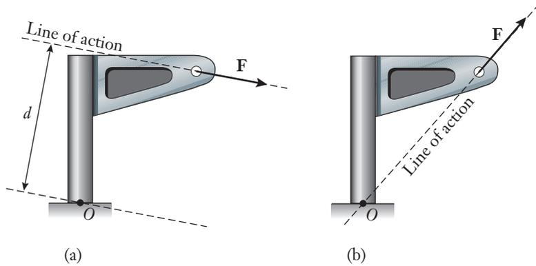
In Figure 4.10(b), the direction of the force has been changed. The force's line of action now passes exactly through point  $O$ , and so the offset distance is  $d = 0$ . No moment is produced, and the force tends to pull the post directly out of its base without rotating it. In short, the orientation of a force as well as its magnitude must be taken into account when you calculate a moment.
