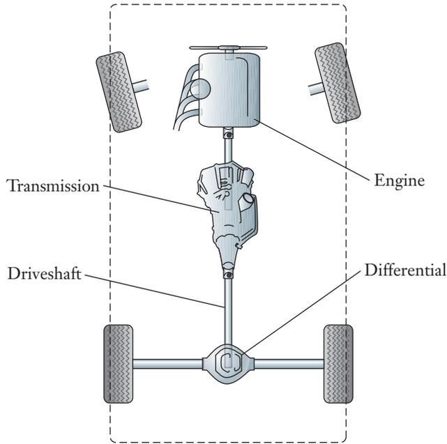
and splits it between the wheels on the driver's and passenger's sides. The differential therefore has one input (the driveshaft) and two outputs (the wheel axles). Look underneath a rear-wheel-drive automobile, and see if you can identify the transmission, driveshaft, and differential.
