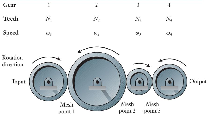
In designing a geartrain, we are more interested in the relationship between the input and output shaft speeds, than in the speeds  $\omega_2$  and  $\omega_3$  of the intermediate shafts. By combining Equations (8.13) and (8.14), we can eliminate the intermediate variable  $\omega_2$ :
