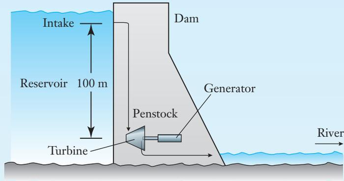
Those kinetic energy components are small when compared to the overall change in gravitational potential energy of the flowing water. Since no heat is involved, the change in gravitational potential energy balances the work output following Equation (7.10). As listed in Table 6.1, the density of fresh water is  $1000 \text{ kg/m}^3$ .
