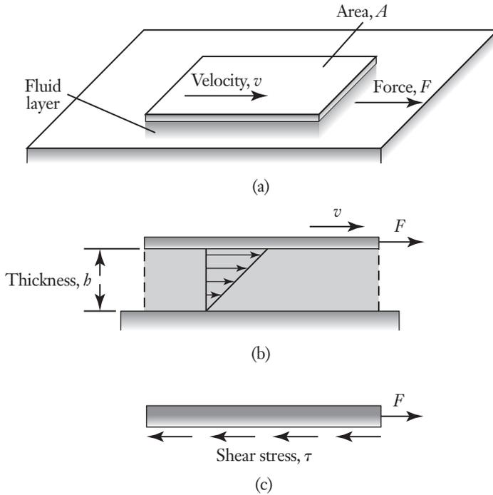
Newton’s second law of motion. The applied force  $F$  is balanced by the cumulative effect of the shear stress
