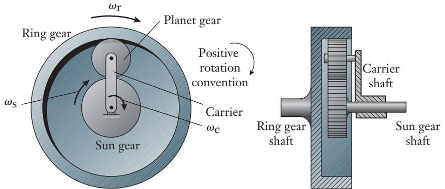
configurations such as these are exploited in the operation of automotive automatic transmissions. By the proper sizing of the sun, planet, and ring gears and by selecting the input and output connections, engineers can obtain either very small or very large velocity ratios in a geartrain of compact size.
