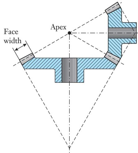
**Figure 8.14** Two bevel gears in mesh.
