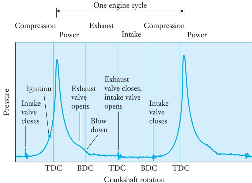
The peak pressure reached in this engine was about 450 psi. For each pulse of pressure in the cylinder, a portion of that rise was associated with the upward compressing motion of the piston in the cylinder, but the dominant factor was combustion following the instant labeled “ignition” in Figure 7.17.
