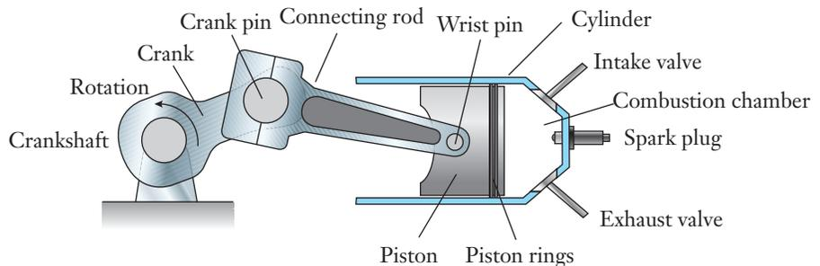
convert the back-and-forth motion of the piston into the crankshaft's rotation. As fuel burns, the high pressure that develops in the cylinder pushes the piston, moves the connecting rod, and rotates the crankshaft. The engine also contains a means for fuel and fresh air to be drawn into the cylinder, and for the exhaust gases to be vented away. We will discuss those processes separately in the context of four-stroke and two-stroke engines.
