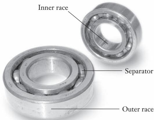
called the *cage* or *retainer*) keeps the balls evenly spaced around the bearing's perimeter and prevents them from contacting one another. Otherwise, if the bearing was used at high speed or subjected to large forces, friction could cause it to overheat and become damaged. In some cases, the gap between the inner and outer races is sealed by a rubber or plastic ring to keep grease in the bearing and dirt out of it.
