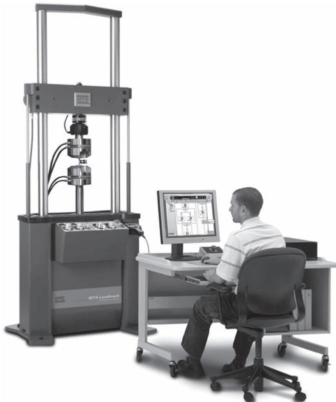
are then converted to stress and strain by using Equations (5.2) and (5.3). When the stress–strain data is drawn on a graph, the slope in the low-strain region is measured to determine  $E$ , and the value of the stress  $S_y$  at the yield point is read off the curve.
