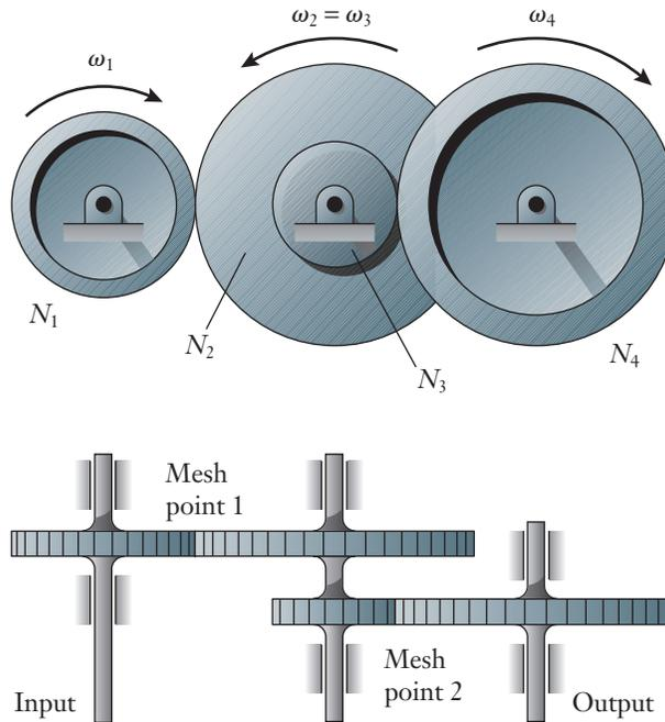
meshing gears. Beginning with the first pair in mesh,
