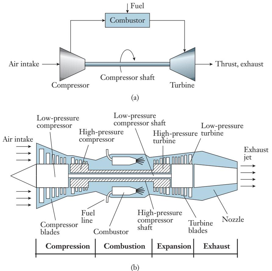
of the turbine. As shown in Figure 7.4, each stage of the turbine is similar in appearance to a fan and comprises many short, specially shaped, blades. The shafts that provide power to the compressor extend forward from the turbine along the length of the engine. The turbine produces just enough power to drive the compressor, and the energy remaining in the combustion gas provides the plane with its forward thrust.
