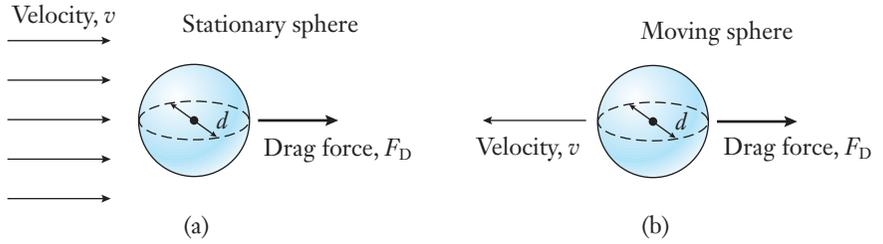
When it is combined with Figure 6.22, Equation (6.14) can be used to calculate the drag force acting on a sphere. When  $Re$  is very low, so that the flow is smooth and laminar, the drag coefficient is given approximately by
