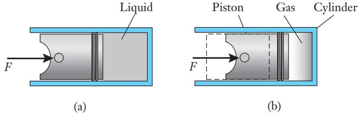
pistons and other actuators. Gases, the second category of fluids, have molecules that separate from one another widely in order to expand and fill an enclosure. A gas can be easily compressed, and, when it is compressed, its density and pressure increase accordingly.
