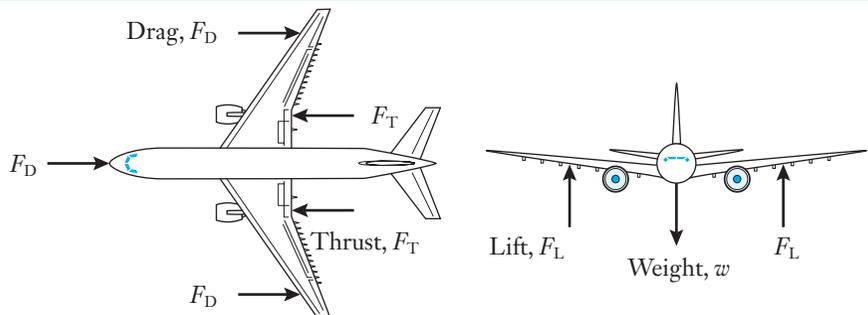
equilibrium: the engines' output overcomes wind resistance, and the wings' lift supports the weight of the aircraft. Lift force is important not only for aircraft wings and other flight control surfaces, but also for the design of propeller, compressor, and turbine blades; ship hydrofoils; and the body contours of commercial and racing automobiles.
