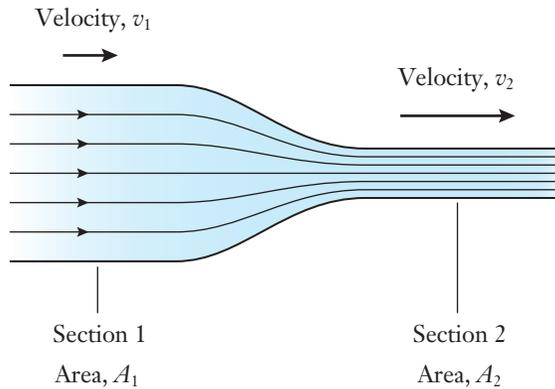
concentrated at some point in the pipe, the amount of fluid that flows into the pipe must also flow out of it. In Figure 6.19, the cross-sectional area of the pipe decreases between sections 1 and 2. For the same volume of fluid to flow out of the constriction per unit time as flows into it, the fluid's velocity in section 2 must be higher. By applying Equation (6.10), the average speed of the flowing fluid changes according to the equation
