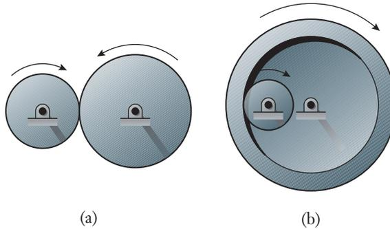
simply called the gear. The pinion and gear mesh at the point where the teeth approach, contact one another, and then separate.
