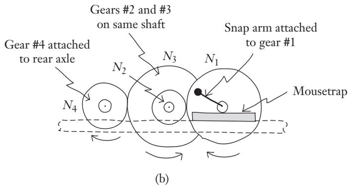
incorporates a two-stage geartrain, and its velocity ratio is set by the numbers of teeth on the four gears. The team's illustration of a two-stage geartrain is arbitrary; a system with only one stage or more than two stages might be preferable. However, the students accept such ambiguity, and they realize that a decision for the geartrain's velocity ratio is not yet necessary.
