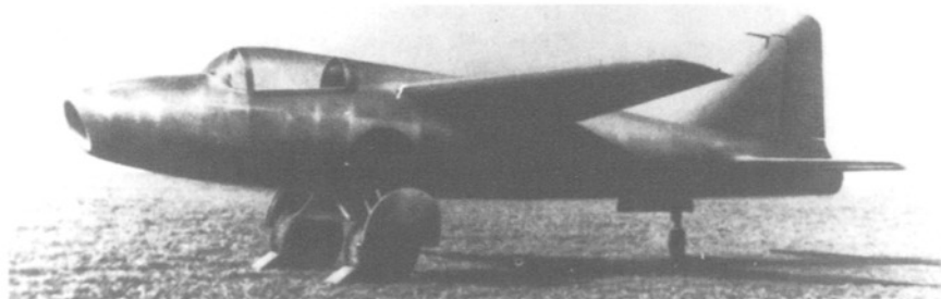
Fig. 13 The world's first jet-powered aircraft, the Heinkel He-178, was powered by the von Ohain-designed He.S3B turbojet engine. (National Air and Space Museum.)
