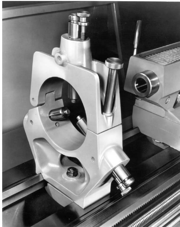
Figure 10.26 The fixed steady (photograph reproduced courtesy of Colchester Lathe Co.)
