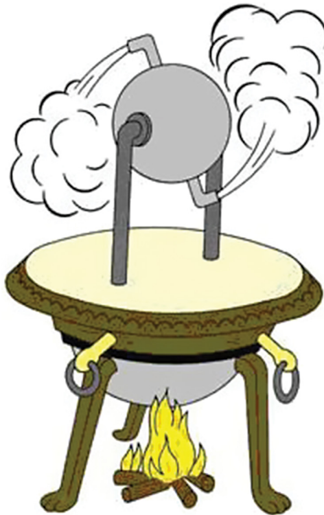
FIGURE 1.1 Schematic of the aeropile by Hero. (From Treager, I.E., Aircraft Gas Turbine Engine Technology , 3rd edn., McGraw-Hill Inc., New York, 1995.)
