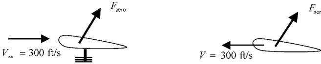
**Fig. 1.16** Airfoil on a test stand and an airfoil in flight.
