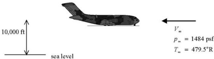
Fig. 1.13 Aircraft at specified flight conditions.
