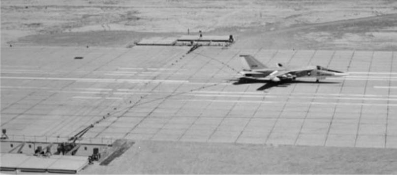
**Fig. 3.42** FB-111 test aircraft engaging Dual BAK-12 system.
