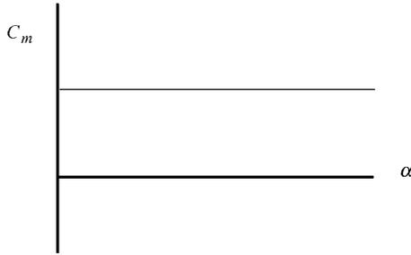
**Fig. 5.17**  $C_m$  vs alpha characteristics for a neutral longitudinal stability.
