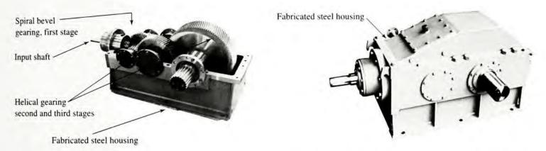
FIGURE 10-15 Spiral bevel, right-angle reducer (Sumitomo Machinery Corporation of America, Teterboro, NJ)
