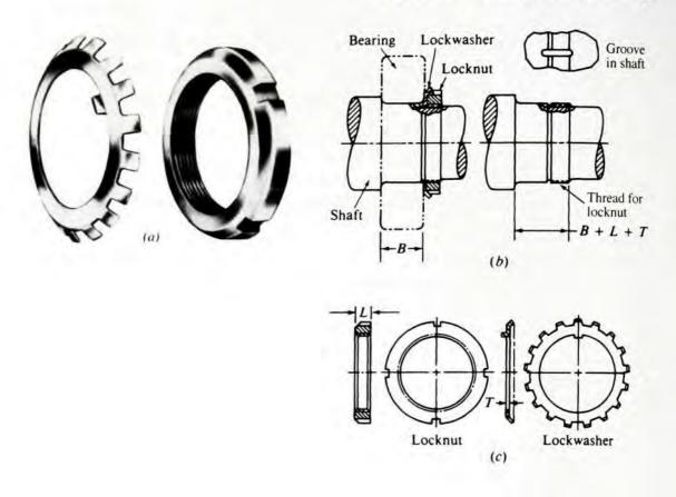
on the bearings. It is desirable to give one bearing complete location while allowing the other bearing to float axially.
