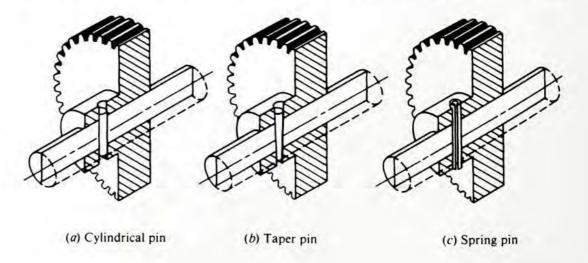
the assembly in position. But, of course, the presence of any of the pin-type connections produces stress concentrations in the shaft. (See Internet site 1.)
