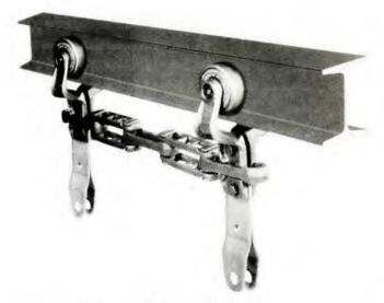
(b) Chain and roller system supported on an I-beam
