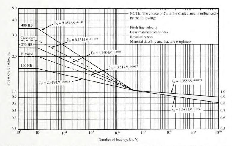
**FIGURE 9–22** Bending strength stress cycle factor,  $Y_N$  (Extracted from AGMA Standard 2001-C95, Fundamental Rating Factors and Calculation Methods for Involute Spur and Helical Gear Teeth, with permission of the publisher, American Gear Manufacturers Association, 1500 King Street, Suite 201, Alexandria, VA 22314)
