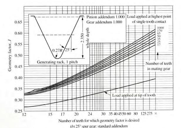
the tooth form actually used, including the form of the fillet, are included in the stress analysis.
