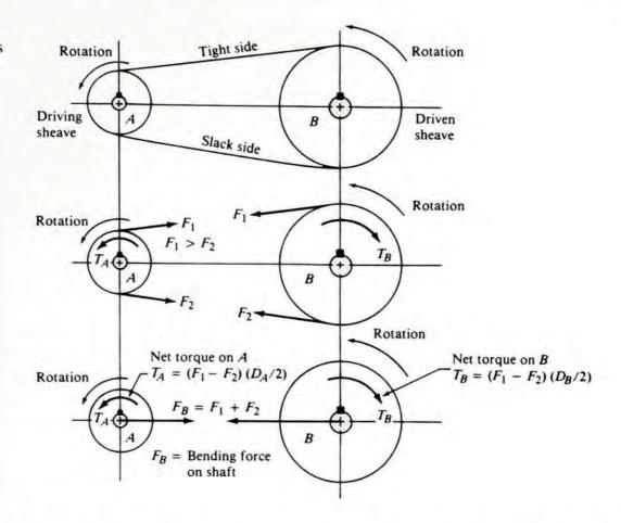
But notice that the bending force on the shaft carrying the sheave is dependent on the *sum*,  $F_1 + F_2 = F_B$ . To be more precise, the components of  $F_1$  and  $F_2$  parallel to the line of centers of the two sprockets should be used. But unless the two sprockets are radically different in diameter, little error will result from  $F_B = F_1 + F_2$ .
