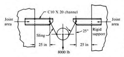
Load shared equally by four brackets (only two shown)
