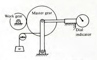
(a) Schematic diagram of a typical gear rolling fixture
