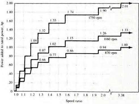
The maximum power added, for ratios of above 3.38, was used to draw the dashed curves in Figures 7–10, 7–11, and 7–12. In most cases, a rough interpolation between the two curves is satisfactory.
