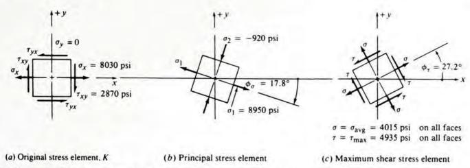
FIGURE 4-11 Relation of maximum shear stress element to the original stress element and the principal stress element
