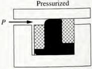
(c) Pressure causes T-ring to move backup ring into gap. Harder backup ring does not extrude.
