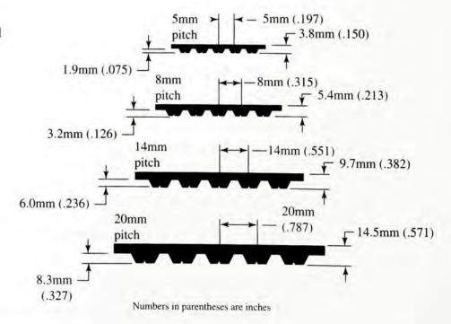
the four common tooth pitches and sizes for commercially available synchronous belts. The pitch is the distance from the center of one tooth to the center of the next adjacent tooth. Standard pitches are 5 mm, 8 mm, 14 mm, and 20 mm.
