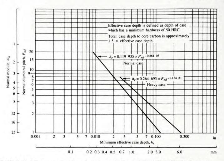
**FIGURE 9–12** Effective case depth for carburized gears,  $h_e$  (Extracted from AGMA 2001-C95 Standard, Fundamental Rating Factors and Calculation Methods for Involute Spur and Helical Gear Teeth, with permission of the publisher, American Gear Manufacturers Association, 1500 King Street, Suite 201, Alexandria, VA 22314)
