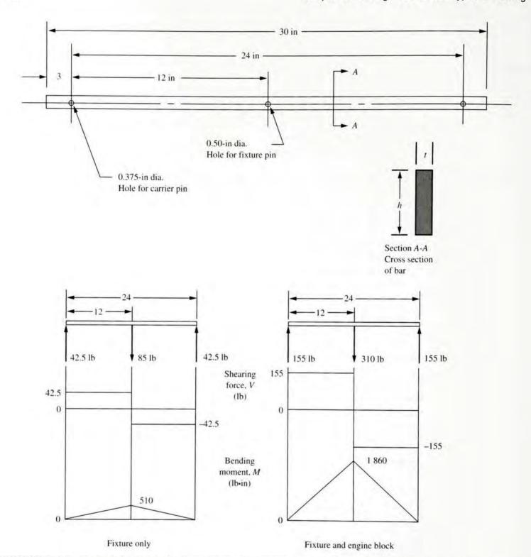
FIGURE 5-19 Basic design of the horizontal bar and the load, shearing force, and bending moment diagrams
