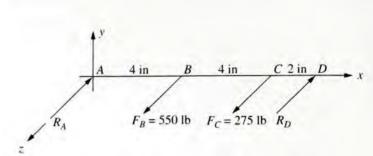
(b) Forces acting on shaft at B and C caused by belt drives
