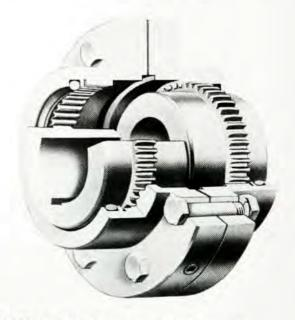
FIGURE 11-19 Gear coupling. Torque is transmitted between crown-hobbed teeth from the coupling half to the sleeve. The crown shape on the gear teeth permits misalignment. (Emerson Power Transmission Corporation, Ithaca, NY)
