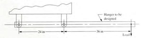
FIGURE P5-80 Hanger for the conveyor system for Problem 80
