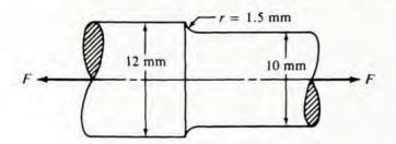
graph of Figure A15-1 to determine the stress concentration factor. That value is used in Equation (3-27) to determine the maximum stress.
