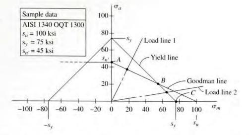
diction, sketched in Figure 5–14, has been shown to provide a good correlation with experimental data, falling just slightly below the scatter of data points.
