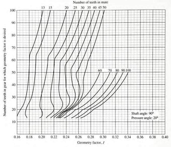
**FIGURE 10–13** Geometry factor, J, for straight bevel gears with  $20^{\circ}$  pressure angle and  $0.120/P_d$  tool edge radius (Extracted from AGMA 6010-F97, Standard for Spur, Helical, Herringbone and Bevel Enclosed Drives, with permission of the publisher, American Gear Manufacturers Association, 1500 King Street, Suite 201, Alexandria, VA 22314)
