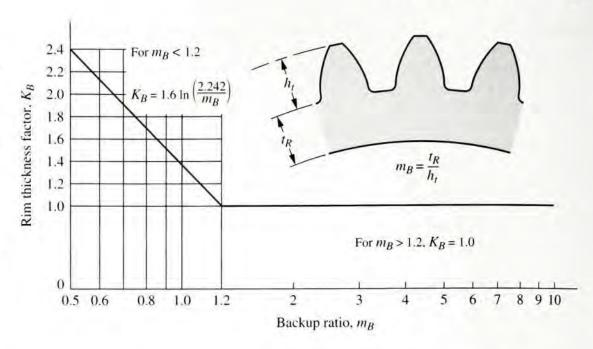
For  $m_B > 1.2$ , the rim is sufficiently strong and stiff to support the tooth, and  $K_B = 1.0$ . The  $K_B$  factor can also be used in the vicinity of a keyseat where a small thickness of metal occurs between the top of the keyseat and the bottom of the tooth space.
