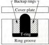
(a) Initial installation of T-ring and backup rings.
