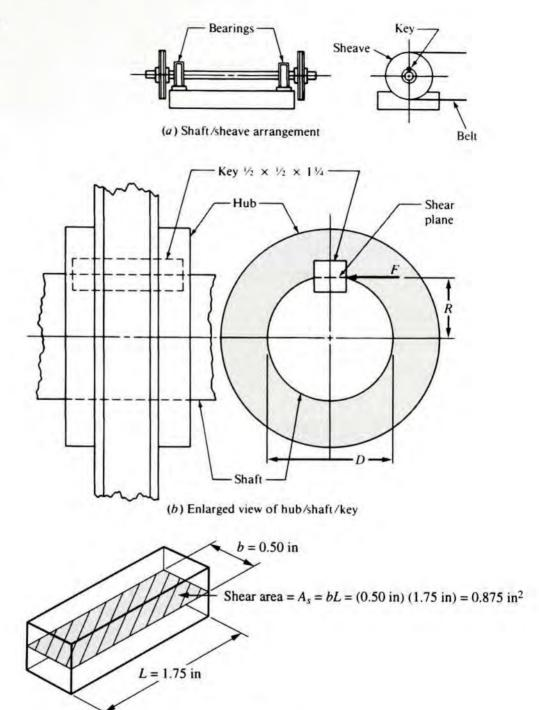
This stress is more properly called the *average shearing* stress, but we will make the simplifying assumption that the stress is uniformly distributed across the shear area.
