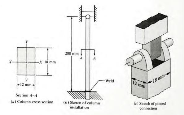
**Step 2.** Compute the transition slenderness ratio. For the AISI 1040 hot-rolled steel, E = 207 GPa and  $s_v = 290$  MPa. Then, from Equation (6–4),
