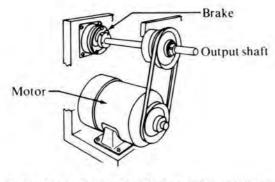
(c) Brake: Stops (brakes) load when coil is energized. Panel shows clutch imparting rotary motion to the output (load) shaft while brake is de-energized. Conversely, de-energizing clutch coil and energizing brake coil causes load to stop.
