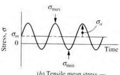
(b) Tensile mean stress —  $\sigma_{\text{max}}$  tensile  $\sigma_{\text{min}}$  compressive -1.0 < R < 0
