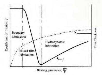
of lubricant and its temperature), the variables affecting the production of the film include the quantity of lubricant supplied, the adhesion of the lubricant to the surfaces, the materials of the journal and the bearing, the structural rigidity of the journal and the bearing, and the surface roughness of the journal and the bearing. After completing the design process presented later in this chapter, you are advised to test the design.
