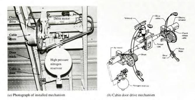
FIGURE 1-9 Aircraft door drive mechanism (The Boeing Company, Seattle, WA)
