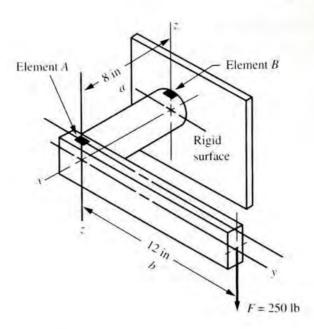
FIGURE 5–21 Freebody diagram of bar
