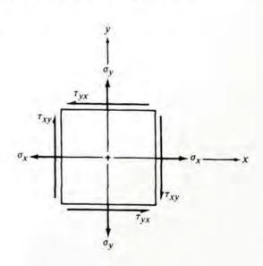
With the stress element defined, the objectives of the remaining analysis are to determine the maximum normal stress, the maximum shear stress, and the planes on which these stresses occur. The governing formulas follow. (See Reference 1 for the derivations.)
