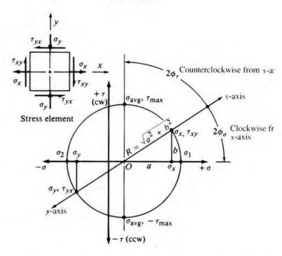
11. The coordinates of the top of the circle give the maximum shear stress and the average normal stress that act on the element having the maximum shear stress. Note that  $\tau_{\text{max}} = R$ .
