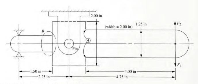
FIGURE P5-75 Beam for Problems 75 and 76
