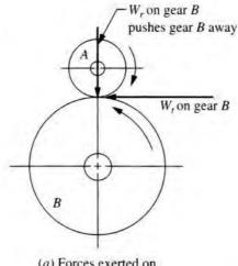
(a) Forces exerted on gear B by gear A.Action forces—gear A drives gear B.
