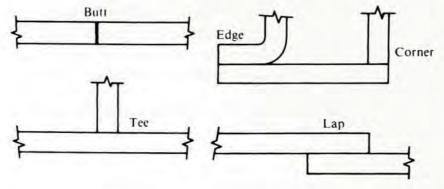
FIGURE 20–7 Some types of welds showing edge preparation
