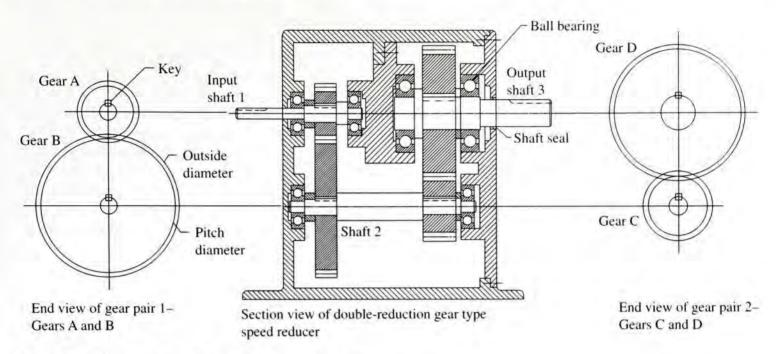
FIGURE 1-12 Conceptual design for a speed reducer
