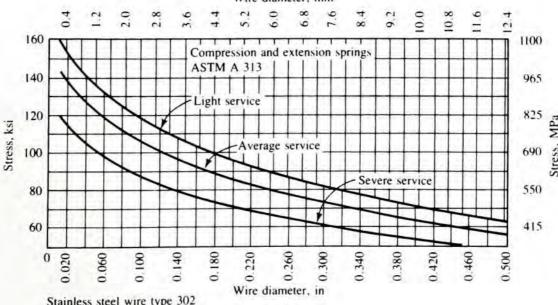
Stainless steel wire type 302 For type 304 multiply by 0.95 For type 316 multiply by 0.85
