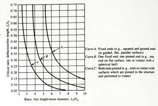
Then, from Figure 19-15, the critical deflection ratio is 0.20. From this we can compute the critical deflection:
