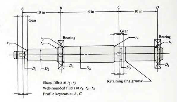
the gear hub and the shaft. The power is then transmitted down the shaft to point C, where it passes through another key into gear C. Gear C then transmits the power to gear Q and thus to the output shaft. The locations of the gears and bearings are dictated by the overall configuration of the reducer.
