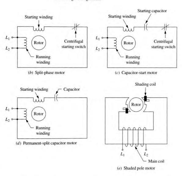
These characteristics make the split-phase motor one of the most popular types, used in business machines, machine tools, centrifugal pumps, electric lawn mowers, and similar applications.
