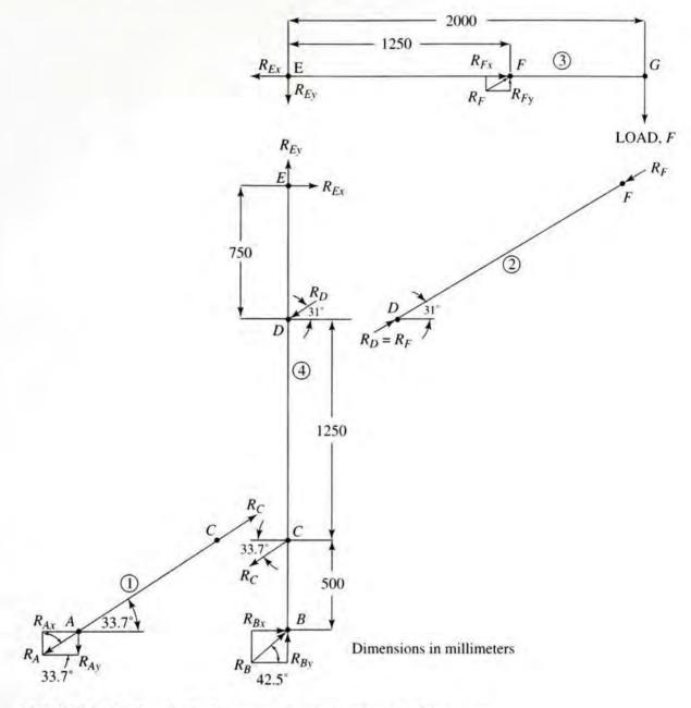
FIGURE 3-3 Free-body diagrams of each component of the crane
