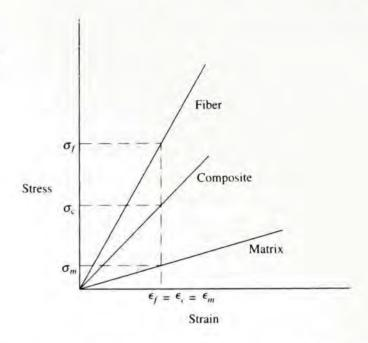
The ultimate strength of the composite,  $s_{uc}$ , is at some intermediate value between  $s_{uf}$  and  $\sigma'_m$ , depending on the volume fraction of fiber and matrix in the composite. That is,
