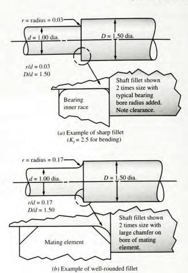
shaft must be smaller yet in order for the bearing to be seated properly against the shoulder. When an element with a large chamfer on its bore is located against the shoulder, or when nothing at all seats against the shoulder, the fillet radius can be much larger (well-rounded), and the corresponding stress concentration factor is smaller. We will use the following values for design for bending:
