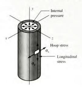
where p = internal pressure in the cylinder
