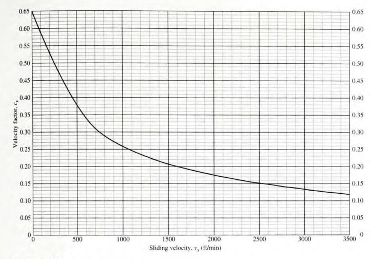
**FIGURE 10–22** Velocity factor,  $C_v$ , vs. sliding velocity.
