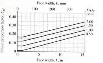
$D_P$  = Pinion diameter For  $F/D_P < 0.50$ , use curve for  $F/D_P = 0.50$ When  $F \le 1.0$  in.  $(F \le 25 \text{ mm})$   $C_{pf} = \frac{F}{10D_P} - 0.025$ When  $1.0 \le F < 15$ ,  $C_{pf} = \frac{F}{10D_P} - 0.0375 + 0.0125F$
