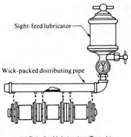
(a) Drip feed lubrication (Type A)
