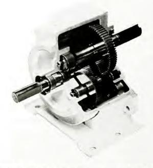
FIGURE 9-35 Double-reduction gear reducer. First stage, helical gears; second stage, spur gears, (Bison Gear & Engineering Corporation, Downers Grove, IL)
