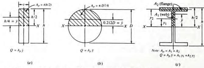
FIGURE 3-13 Illustrations of  $A_p$  and  $\bar{y}$  used to compute Q for three shapes
