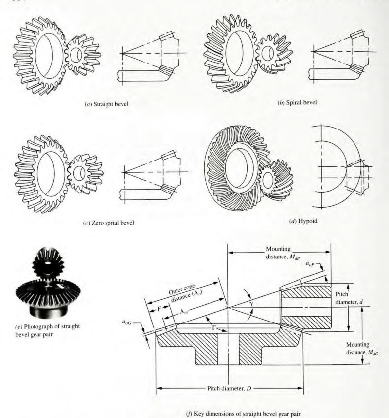
**FIGURE 8–22** Types of bevel gears [Parts (a) through (d) extracted from ANSI/AGMA 2005-C96, *Design Manual for Bevel Gears*, with the permission of the publisher, the American Gear Manufacturers Association, 1500 King Street, Suite 201, Alexandria, VA 22314. Photograph in (e) courtesy of Emerson Power Transmission Corporation, Browning Division, Maysville, KY
