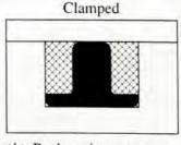
(b) Backup rings squeeze bottom and sides of T-rings.
