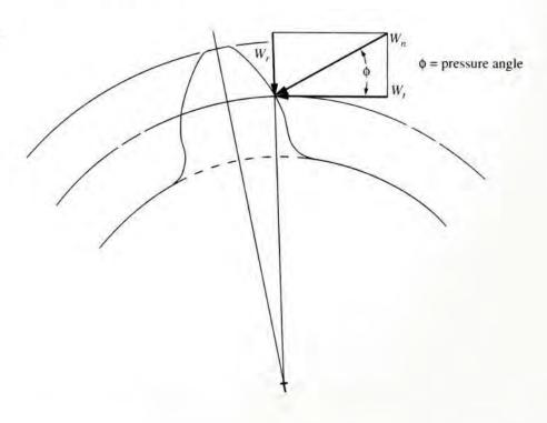
The torque exerted on a gear is the product of the transmitted load,  $W_t$ , and the pitch radius of the gear. The torque is also equal to the power transmitted divided by the rotational speed. Then
