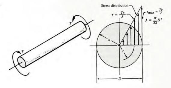
**Example Problem 3–6** Compute the maximum torsional shear stress in a shaft having a diameter of 10 mm when it carries a torque of 4.10 N·m.
