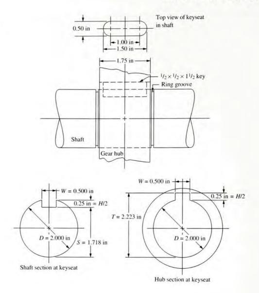
chord of that segment times the thickness of the key. The following equations describe the geometry:
