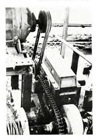
(b) Photograph of an actual drive installation. Note that guards have been removed from the belt and chain drives to show detail.
