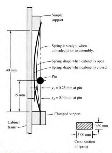
**FIGURE P5–9** Cabinet latch spring (Problems 9 and 22)
