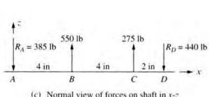
(c) Normal view of forces on shaft in x-z plane with reactions at bearings
