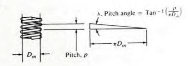
You can see the logic of this formula by taking one coil of a spring and unwrapping it onto a flat surface, as illustrated in Figure 19–7. The horizontal line is the mean circumference of the spring, and the vertical line is the pitch, p.
