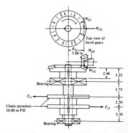
FIGURE P12-37 Bevel gears shown in section for Problem 37. See Chapter 10.
