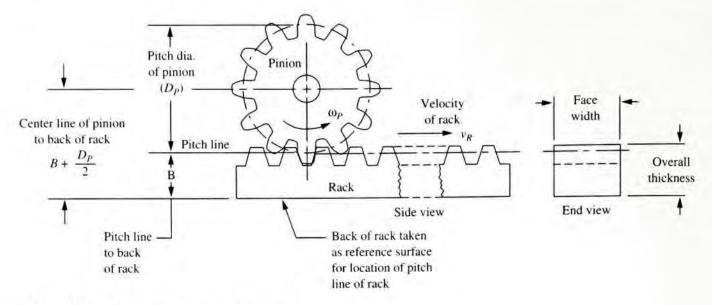
FIGURE 8-19 Rack driven by a pinion
