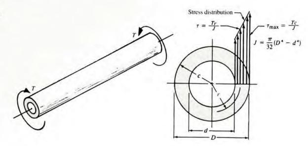
For design, it is convenient to define the polar section modulus, Z<sub>n</sub>:
