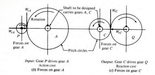
Forces on the Shaft: The next step is to show these forces on the shaft in their proper planes of action and in the proper direction. The reactions at the bearings are computed, and the shearing force and bending moment diagrams are prepared. The results are shown in Figure 12–12.
