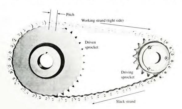
FIGURE 7–21 Some roller chain styles (Rexnord, Inc., Milwaukee, WI)
