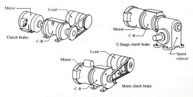
(e) Three types of mountings for clutch-brake modules: Clutch brake combines functions of clutch and brake in a complete preassembled package with input and output shafts. C-flange clutch brake performs same function but for use between NEMA "C" flange motor and speed reducer. Motor clutch brake is a preassembled module for mounting to a NEMA "C" flange motor and presenting an output shaft for connection to load.
