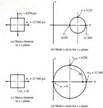
free face of the element. Likewise, there are no shear stresses on this face. The Mohr's circle for this plane is shown in Part (d) of the figure. The maximum shear stress is equal to the radius of the circle, 6250 psi, or *twice* as much as would be predicted from the x-y plane. This approach should be used any time the two principal stresses in a biaxial stress problem have the same sign.
