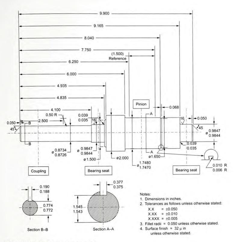
FIGURE 15-4 Final design of the input shaft
