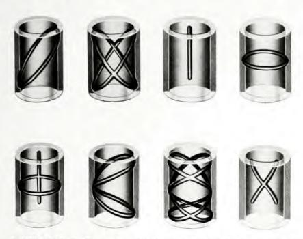
**FIGURE 16–9** Examples of styles of grooving for plain bearings (Bunting Bearings Corp., Holland, OH)
