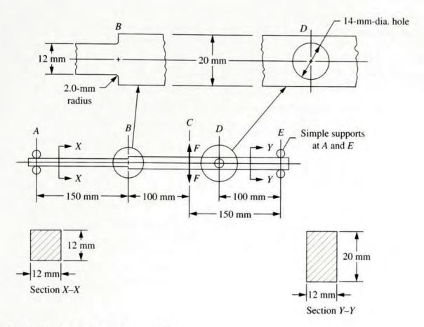
FIGURE P5-67 Beam for Problems 67 and 68
