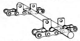
(c) Attachments used as spacers to convey and position long objects
