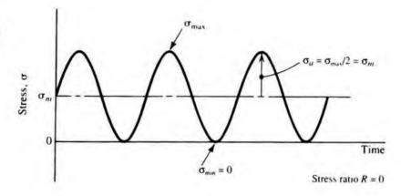
nonzero mean is considered a fluctuating stress. Figure 5–4 also shows the possible ranges of values for the stress ratio R for the given loading patterns.
