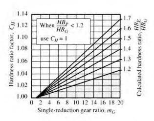
FIGURE 9-25 Hardness ratio facator,  $C_H$  (throughhardenced gears) (Extract from AGMA Standard 2001-C95, Fundamental Rating Factors and Calculation Methods for Involute Spur and Helical Gear Teeth, with the permission of the publisher, American Gear Manufacturers Association, 1500 King Street, Suite 201, Alexandria, VA 22314)
