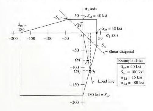
ultimate tensile strength lines are extended from the first quadrant into the second and fourth quadrants to the point where each intersects the *shear diagonal*, drawn at 45 degrees through the origin. Then the failure line proceeds at an angle to the ultimate compressive strength.
