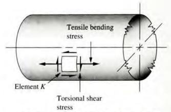
(d) Enlarged view of element K on front of shaft
