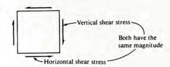
Note that the vertical shearing stress is equal to the *horizontal shearing stress* because any element of material subjected to a shear stress on one face must have a shear stress of the same magnitude on the adjacent face for the element to be in equilibrium. Figure 3–15 shows this phenomenon.
