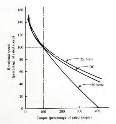
load is similar, regardless of the nature of the input power. Note also that these motors have poor speed regulation; that is, the speed varies greatly with load.
