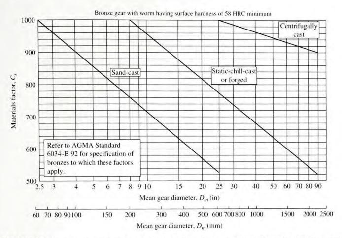
**FIGURE 10–20** Materials factor,  $C_s$ , for center distance > 3.0 in (76 mm) (Extracted from AGMA Standard 6034-B92, *Practice for Enclosed Cylindrical Wormgear Speed Reducers and Gearmotors*, with the permission of the publisher, American Gear Manufacturers Association, 1500 King Street, Suite 201, Alexandria, VA 22314)
