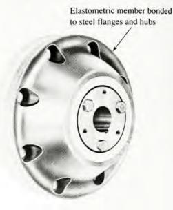
FIGURE 11–17 Ever-Flex coupling. The features of this coupling are that it (1) generally minimizes torsional vibration; (2) cushions shock loads; (3) compensates for parallel misalignment up to 1/32 in; (4) accommodates angular misalignment of ±3°; and (5) provides adequate end float, ±1/32 in. (Emerson Power Transmission Corporation, Ithaca, NY)
