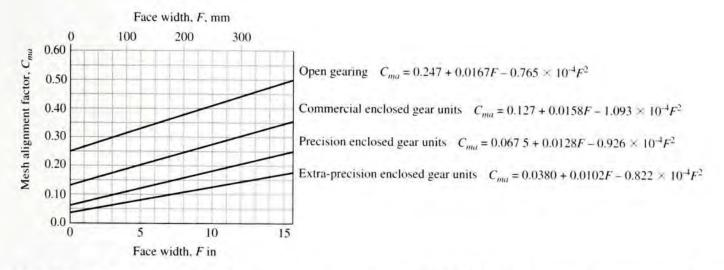
**FIGURE 9–19** Mesh alignment factor,  $C_{ma}$  (Extracted from AGMA 2001-C95 Standard, Fundamental Rating Factors and Calculation Methods for Involute Spur and Helical Gear Teeth, with permission of the publisher, American Gear Manufacturers Association, 1500 King Street, Suite 201, Alexandria, VA 22314)
