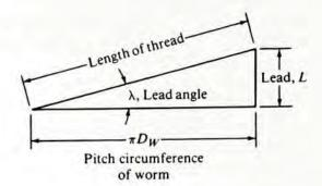
were unwrapped from the pitch cylinder and laid flat on the paper. The length of the hypotenuse is the length of the thread itself. The vertical side is the lead, L. The horizontal side is the circumference of the pitch cylinder,  $\pi D_W$ , where  $D_W$  is the pitch diameter of the worm. Then
