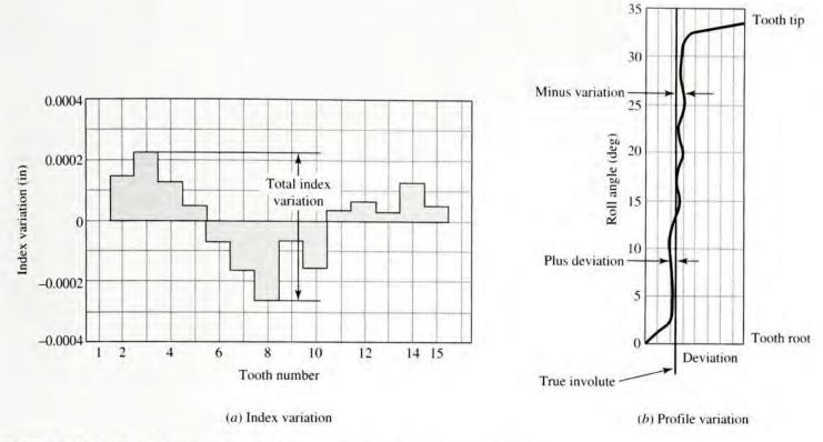
FIGURE 9-9 Typical output charts from an analytical measurement system (Process Equipment Company, Tipp City, Ohio)
