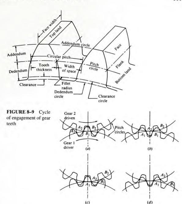
made from Figure 8–9 is that throughout the engagement cycle there are two circles, one from each gear, that remain tangent. These are called the *pitch circles*. The diameter of the pitch circle of a gear is its *pitch diameter*; the point of tangency is the *pitch point*.
