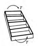
(a) Conventional cross bracing  $\theta = 10.8^{\circ}$
