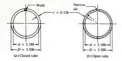
gle of twist for a hollow circular tube is inversely proportional to the polar moment of inertia J. All other terms in the two equations are the same for each design. Therefore, the ratio of  $\theta_{\text{open}}$  to  $\theta_{\text{closed}}$  is equal to the ratio J/K. From Appendix 1, we find
