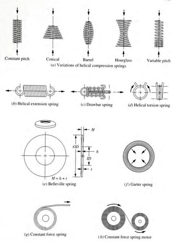
The *drawbar spring* incorporates a standard helical compression spring with two looped wire devices inserted through the inside of the spring. With such a design, a tensile force can be exerted by pulling on the loops while still placing the spring in compression. It also provides a definite stop as the compression spring is compressed to its solid height.
