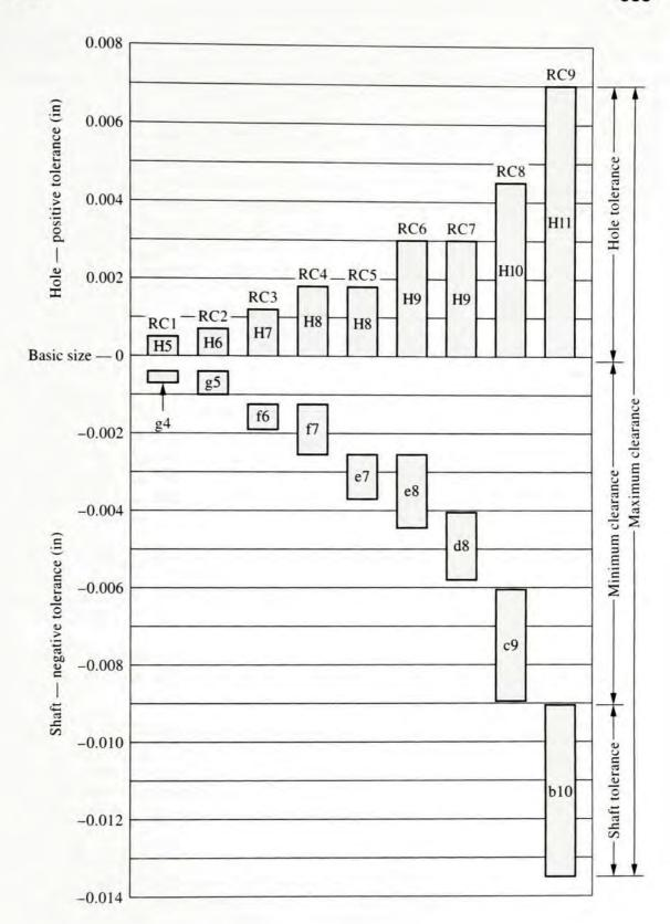
The codes within the tolerance bars in Figure 13–4 refer to the tolerance grades mentioned earlier. The capital H combined with a tolerance grade number is used for the hole in the basic hole system for which there is no fundamental deviation from the basic size. The lowercase letters in the shaft tolerance bars indicate some fundamental deviation of the shaft size from the basic size. Then the tolerance is added to the fundamental deviation. The size of the tolerance is indicated by the number.
