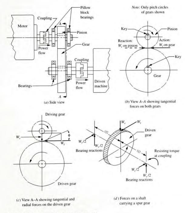
FIGURE 9-1 Power flow through a gear pair
