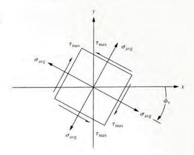
The angle of inclination of the element on which the maximum shear stress occurs is computed as follows:
