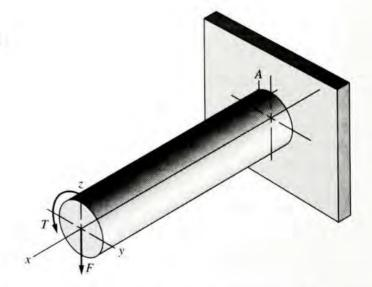
A convenient and useful concept called *equivalent torque* can be developed from Equation (4–7) for the special case of a body subjected to only bending and torsion.
