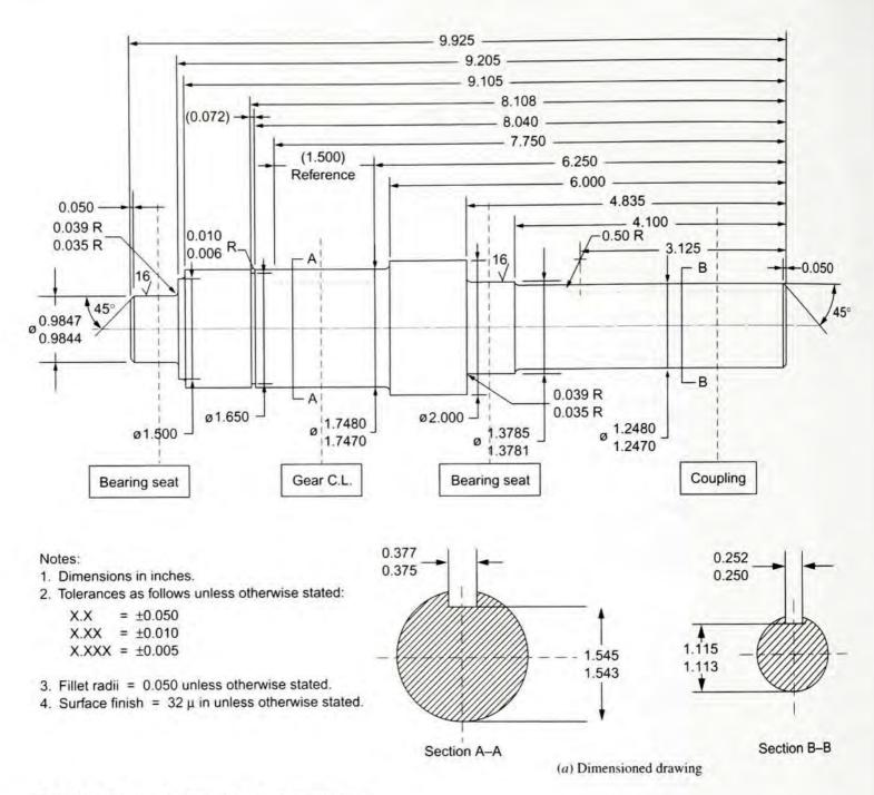
FIGURE 15-5 Final design of the output shaft
