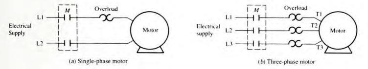
**FIGURE 21–20** Manual starters. M = normally open contactors. All actuate together.
