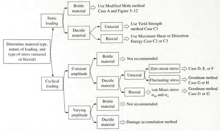
FIGURE 5-17 Logic diagram for visualizing methods of design analysis
