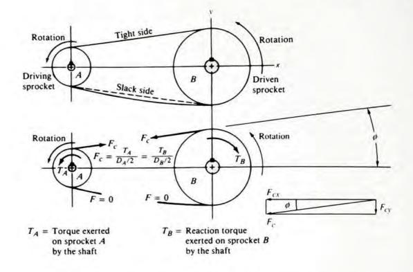
Notice that the force,  $F_c$ , acts along the direction of the tight side of the belt. Because of the size difference between the two sprockets, that direction is at some angle from the centerline between the shaft centers. A precise analysis would call for the force,  $F_c$ , to be resolved into components parallel to the centerline and perpendicular to it. That is,
