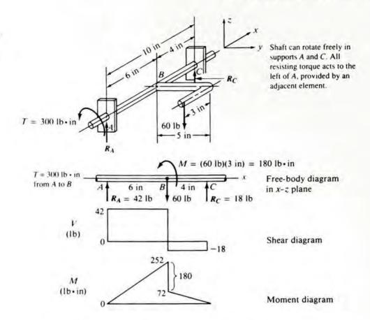
When a concentrated bending moment acts on a beam in a counterclockwise direction, the moment diagram drops; when a clockwise concentrated moment acts, the moment diagram rises.
