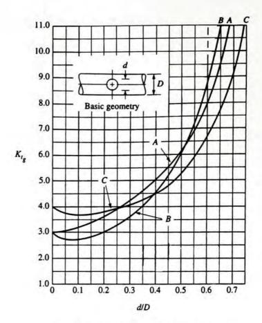
Note:  $K_{lg}$  is based on the nominal stress in a round bar without a hole (gross section).
