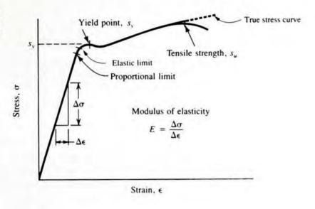
FIGURE 2-2 Typical stress-strain diagram for aluminum and other metals having no yield point
