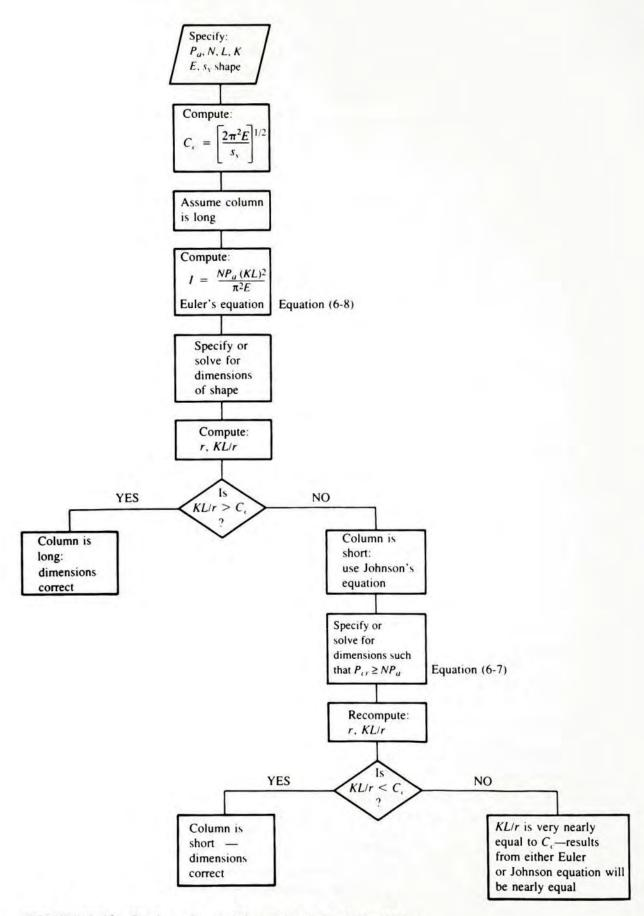
FIGURE 6-13 Design of a straight, centrally loaded column
