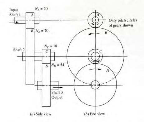
This is the input speed divided by the output speed, the basic definition of the train value. This process can be expanded to any number of stages of reduction in a gear train.
