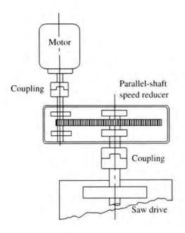
Parallel-shaft speed reducer
