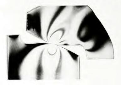
us to determine the stress concentration factor,  $K_i$ , for the fillet area. Placing this into equation (9–12) gives
