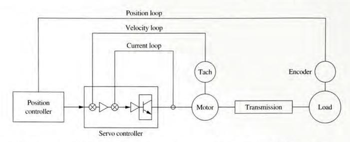
FIGURE 21-33 Servomotor controller system (Rockwell Automation/Allen-Bradley, Milwaukee, WI)
