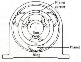
(b) Schematic arrangement of planetary gearing
