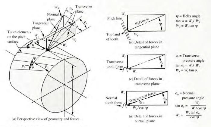
FIGURE 8-21 Helical gear geometry and forces
