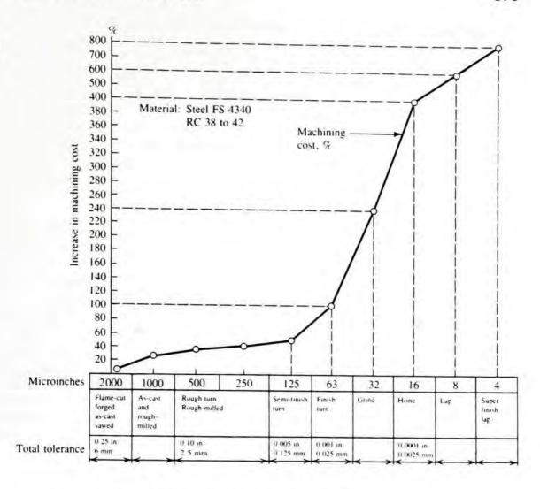
several passes, ending with a fine finish cut. Cutting tool changes must be more frequent, also, as wear of the tool takes the part out of tolerance.
