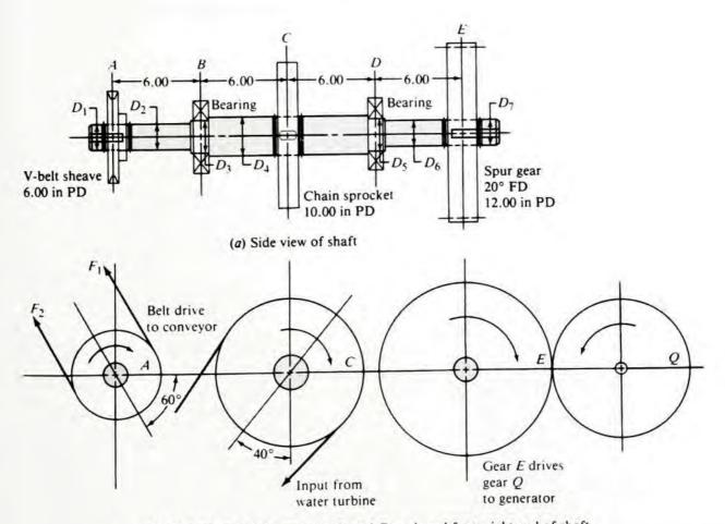
(b) Orientation of elements A, C, and E as viewed from right end of shaft
