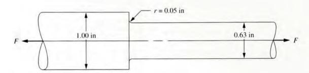
FIGURE P5-73 Rod for Problems 73 and 74
