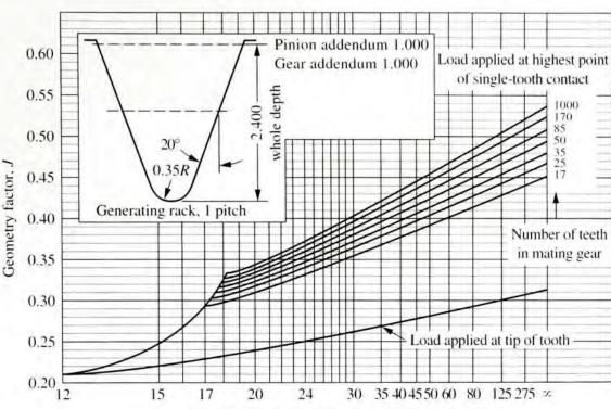
Number of teeth for which geometry factor is desired (a) 20° spur gear: standard addendum
