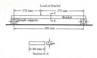
FIGURE P5-8 Seat bracket (Problems 8, 19, and 20)
