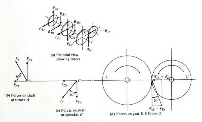
**FIGURE 12–15** Forces resolved into x- and y-components
