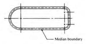
The shear stress computed by this approach is the *average stress* in the tube wall. However, if the wall thickness *t* is small (a thin wall), the stress is nearly uniform throughout the wall, and this approach will yield a close approximation of the maximum stress. For the analysis of tubular sections having nonuniform wall thickness, see References 2, 4, and 7.
