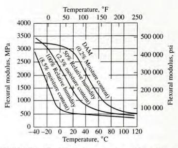
FIGURE 2–18 Effect of temperature and humidity on the flexural modulus of nylon 66 (DuPont Polymers, Wilmington, DE)
