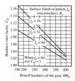
FIGURE 9–26 Hardness ratio factor,  $C_H$  (surface-hardened pinions) (Extracted from AGMA Standard 2001-C95, Fundamental Rating Factors and Calculation Methods for Involute Spur and Helical Gear Teeth, with permission of the publisher, American Gear Manufacturers Association, 1500 King Street, Suite 201, Alexandria, VA 22314)
