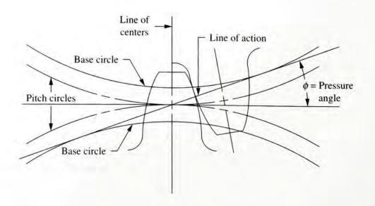
FIGURE 8-13 Fulldepth, involute-tooth form for varying pressure angles
