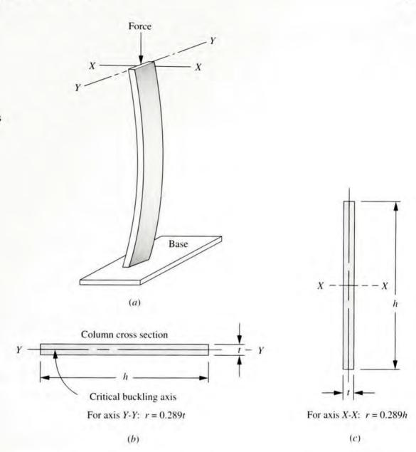
prohibits any tendency for the fixed end of the column to rotate. A column end securely welded to a rigid base plate is also a good approximation of a fixed-end column.
