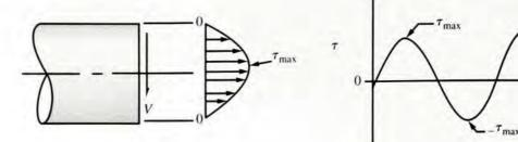
(a) Distribution of shearing stress on a circular cross section of a shaft
