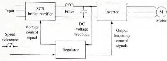
(a) Schematic diagram of variable voltage inverter
