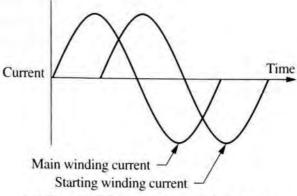
(a) Phase shift between main winding current and starting winding current
