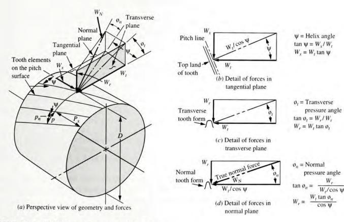
FIGURE 10-4 Helical gear geometry and forces
