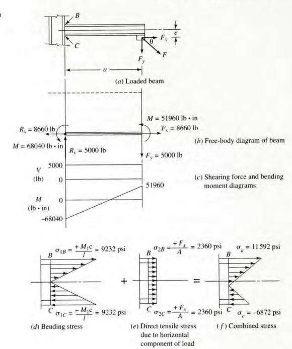
Section modulus =  $S = 7.37 \text{ in}^3$ ; area =  $A = 3.67 \text{ in}^2$  (Table A16–4). Eccentricity of the load = e = 6.0 in from the neutral axis of the beam to the line of action of the horizontal component of the applied load.
