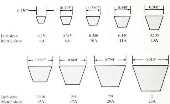
7–3(d). The following standards of the Society of Automotive Engineers (SAE) give dimensions and performance standards for automotive belts.
