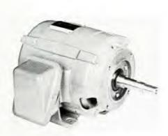
**D-Flange Mounting.** A machined flange is provided on the shaft end of the motor with a standard pattern of through clearance holes for bolts for attaching the motor to the driven equipment. The flange design is controlled by NEMA.
