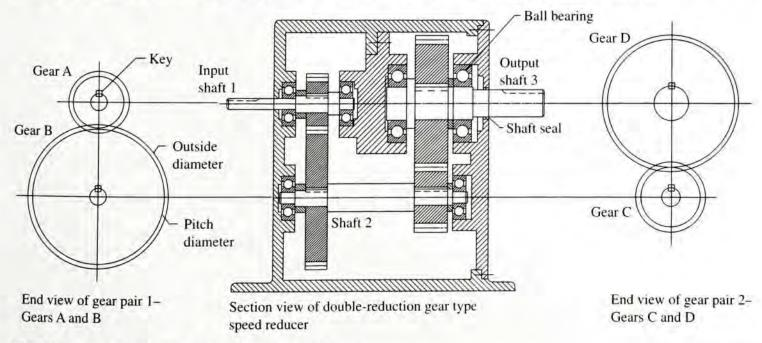
FIGURE 8-3 Conceptual design for a speed reducer
