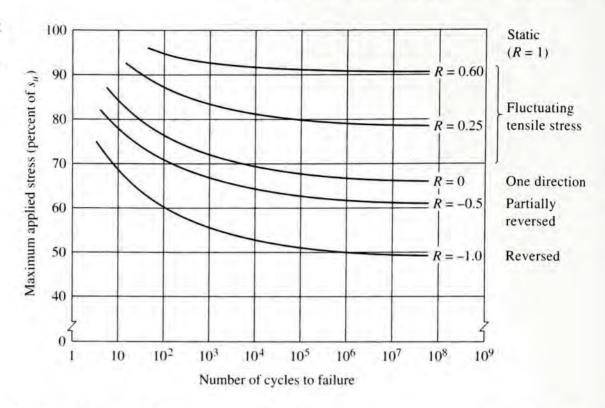
**Effect of Stress Ratio on Endurance Strength.** Figure 5–11 shows the general variation of endurance-strength data for a given material when the stress ratio R varies from -1.0 to +1.0, covering the range of cases including the following:
