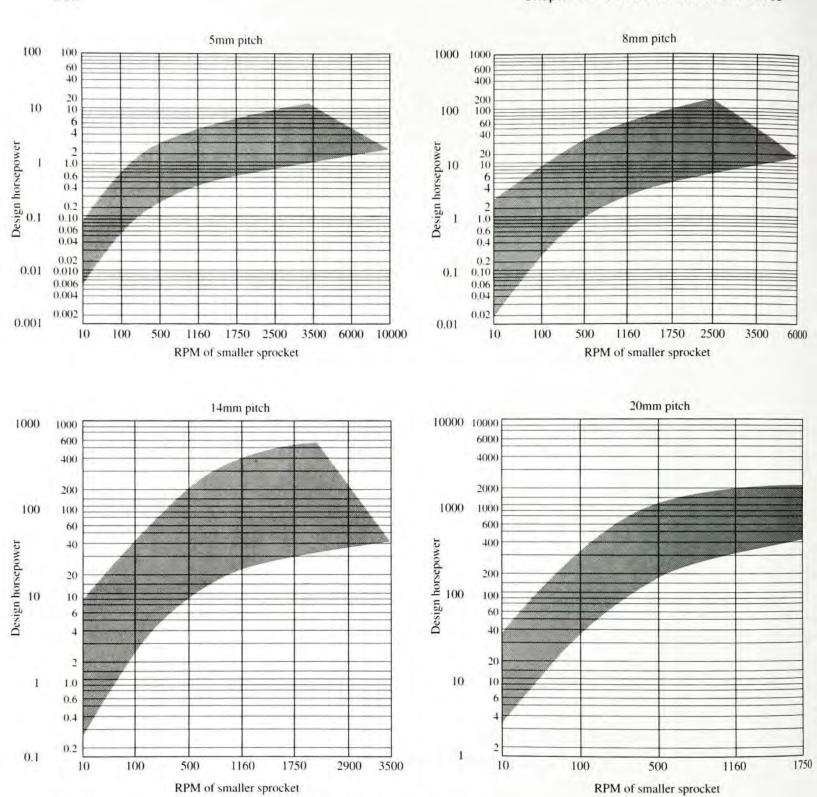
FIGURE 7-19 Belt pitch selection guide for synchronous belts
