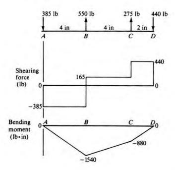
Results Element K is subjected to bending that produces a tensile stress acting in the x-direction. Also, there is a torsional shear stress acting at K. Figure 4–8 shows the shearing force and bending moment diagrams for the shaft and indicates that the bending moment at K is 1540 lb·in. The bending stress is therefore
