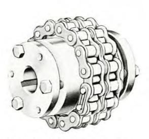
FIGURE 11–16 Chain coupling. Torque is transmitted through a double roller chain. Clearances between the chain and the sprocket teeth on the two coupling halves accommodate misalignment. (Emerson Power Transmission Corporation, Ithaca, NY)
