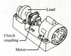
(b) Clutch coupling: Transmits rotary motion to an in-line shaft only when coil is energized. Split shaft applications.
