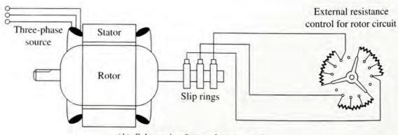
(b) Schematic of wound rotor motor with external resistance control The wound-rotor design is used in such applications as printing presses, crushing equipment, conveyors, and hoists.
