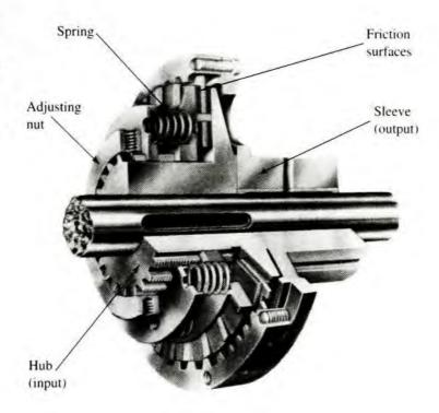
**Spring-applied.** Sometimes called a *fail-safe* design when applied to a brake, the brake is applied automatically by springs unless there is some opposing force present. Thus, if power fails, or if air pressure or hydraulic pressure is lost, or if the operator is unable to perform the function, the springs apply the brake and stop the load. The concept may also be used to engage or to disengage a clutch.
