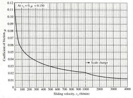
choice of formula depends on the sliding velocity. *Note:*  $v_s$  must be in ft/min in the formulas; 1.0 ft/min = 0.0051 m/s.
