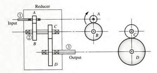
FIGURE P12-38 Gear reducer for Problems 38 and 39
