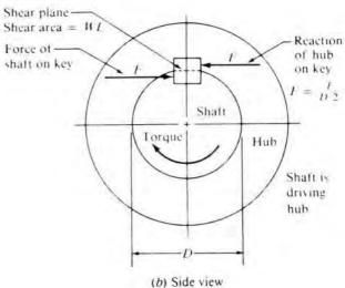
The failure in bearing is related to the compressive stress on the side of the key, the side of the shaft keyseat, or the side of the hub keyseat. The area in compression is the same for either of these zones,  $L \times (H/2)$ . Thus, the failure occurs on the surface with the lowest compressive yield strength. Let's define a design stress for compression as
