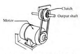
(a) Clutch: Transmits rotary motion to a parallel shaft only when coil is energized, by using sheaves, sprockets, gears, or timing pulleys.
