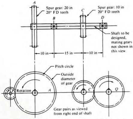
Input: Gear P drives gear A
