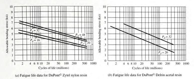
**FIGURE 9–39** Fatigue life data for two types of plastic materials used for gears (DuPont Polymers, Wilmington, DE)
