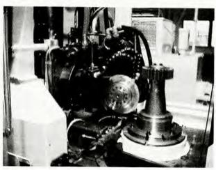
(a) Gear grinding machine
