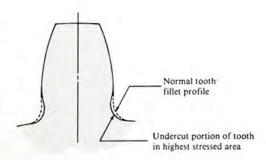
To alleviate the problem of interference, increase the addendum of the pinion while decreasing the addendum of the gear. The center distance can remain the same as its theoretical value for the number of teeth in the pair. But the resulting gears are, of course, nonstandard. (See Reference 10.) It is possible to make the pinion of a gear pair larger than standard while keeping the gear standard if the center distance for the pair is enlarged. (See Reference 9.)
