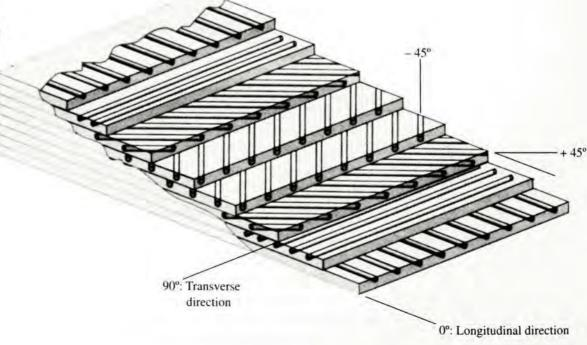
structure (through the thickness) are still quite low because fibers do not extend in that direction. Also, the strength and the stiffness in the primary directions are somewhat lower than if the plies were aligned in the same direction. Table 2–11 also shows sample data for a quasi-isotropic laminate compared with one having unidirectional fibers in the same matrix.
