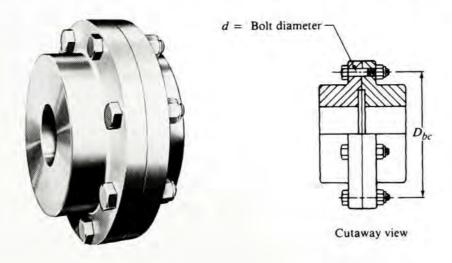
occur, parts of the coupling move with little or no resistance. Thus, no significant axial or bending stresses are developed in the shaft.
