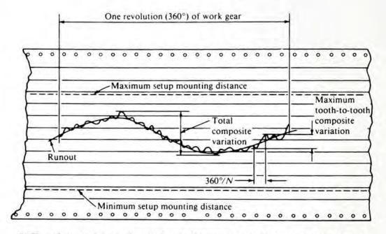
(b) Chart of gear-tooth errors of a typical gear when run with a specified gear in a rolling fixture
