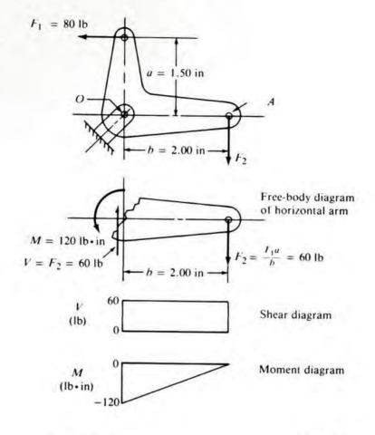
FIGURE 3–22 Bending moment on a print head
