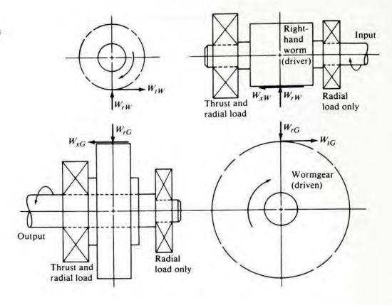
and wormgear with the forces acting on each. Note that because of the 90° orientation of the two shafts,
