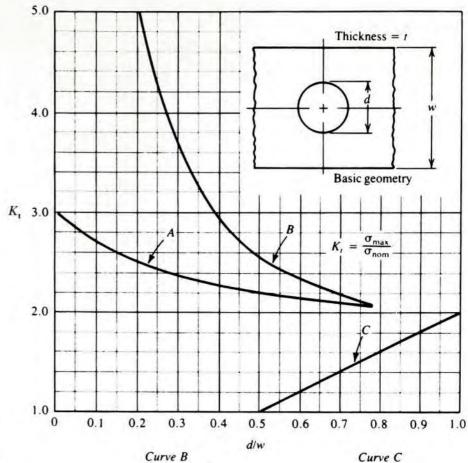
Curve A Direct tension on plate
