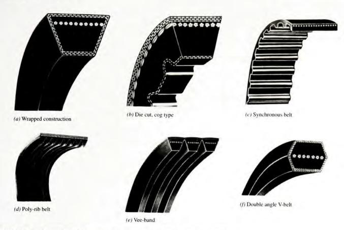
FIGURE 7-3 Examples of belt construction (Dayco Corp., Dayton, OH)
