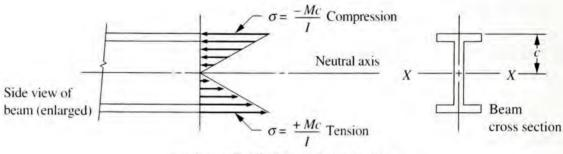
(c) Stress distribution on beam section
