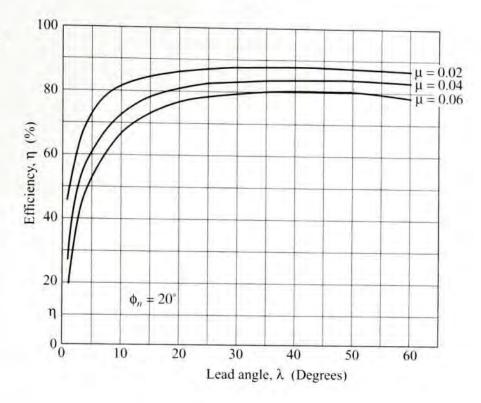
Efficiency for a wormgear drive with the usual case of the input coming through the worm can also be computed directly from the following equation.
