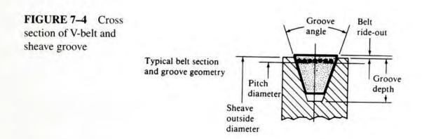
vide the flexibility needed to allow the belt to pass around the sheave. Often an outer fabric cover is added to give the belt good durability.
