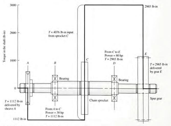
FIGURE 12-14 Torque distribution in the shaft
