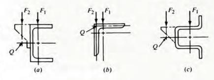
action of the loads on such sections passes through the axis of symmetry, then there is no tendency for the section to twist, and the flexure formula applies.
