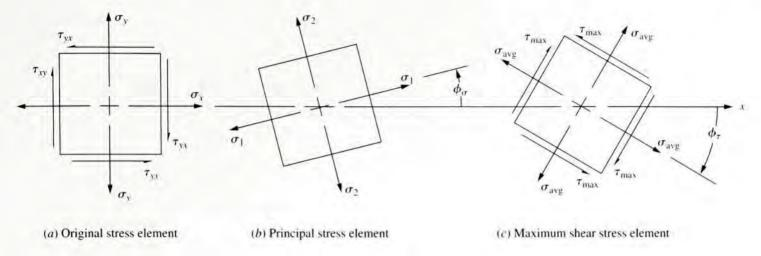
FIGURE 4-6 Relationships among original stress element, principal stress element, and maximum shear stress element for a given loading
