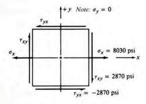
FIGURE 4–16 Partially completed Mohr's circle
