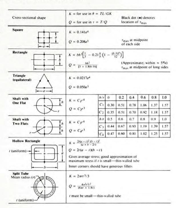
$$\tau_{\text{max}} = \frac{T}{Q} = \frac{15\,000\,\text{lb}\cdot\text{in}}{(1.115\,\text{in}^3)} = 13\,460\,\text{psi}$$
