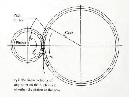
This set of equations says that the pitch line speeds of the pinion and the gear are the same. Equating these two and solving for  $\omega_P/\omega_G$  gives our definition for the velocity ratio, VR:
