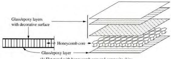
(b) Flat panel with honeycomb core and composite skins
