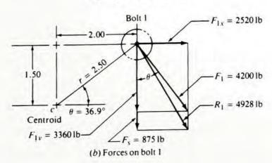
Step 4. Compute the radial distance from the centroid of the bolt pattern to the center of each bolt. In this problem, each bolt has a radial distance of
