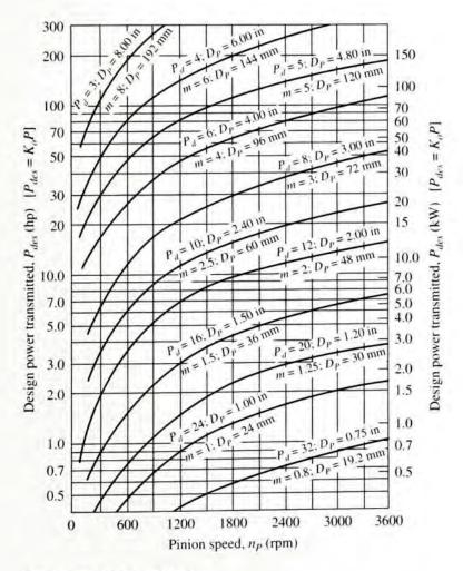
For all curves: 20° full depth teeth:  $N_P = 24$ ;  $N_G = 96$ ;  $m_G = 4.00$ ;  $F = 12/P_d$ ;  $Q_v = 6$ Steel gears, HB 300;  $s_{at} = 36\,000$  psi;  $s_{ac} = 126\,000$  psi
