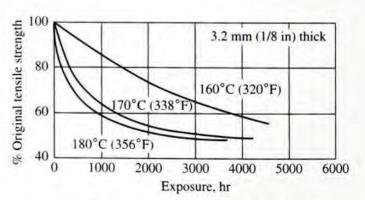
FIGURE 2-20 Effect of exposure to elevated temperature on a thermoplastic polyester resin (PET) (DuPont Polymers, Wilmington, DE)
