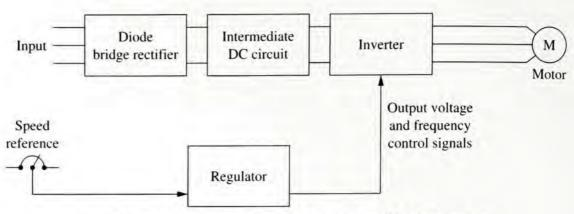
(a) Schematic diagram of pulse-width modulation (PWM) controller
