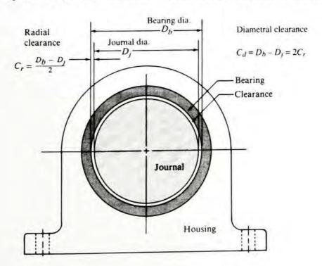
The stationary member that mates with the journal is called simply the *bearing*. Other names used for plain surface bearings are *journal bearings* and *sleeve bearings*.
