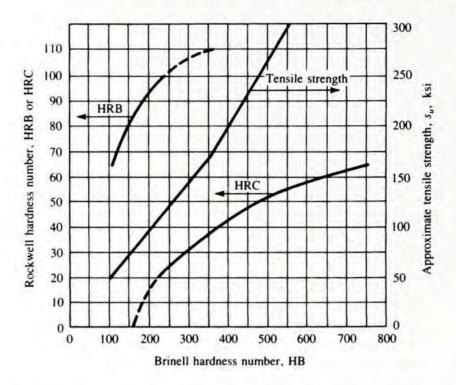
TABLE 2-1 Comparison of hardness scales with tensile strength
