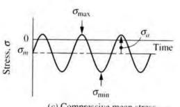
(c) Compressive mean stress —  $\sigma_{\text{max}}$  tensile  $\sigma_{\text{min}}$  compressive —  $\infty < R < -1.0$
