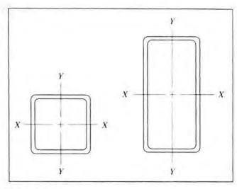
TABLE A16-5 Properties of steel structural tubing, square and rectangular\*
