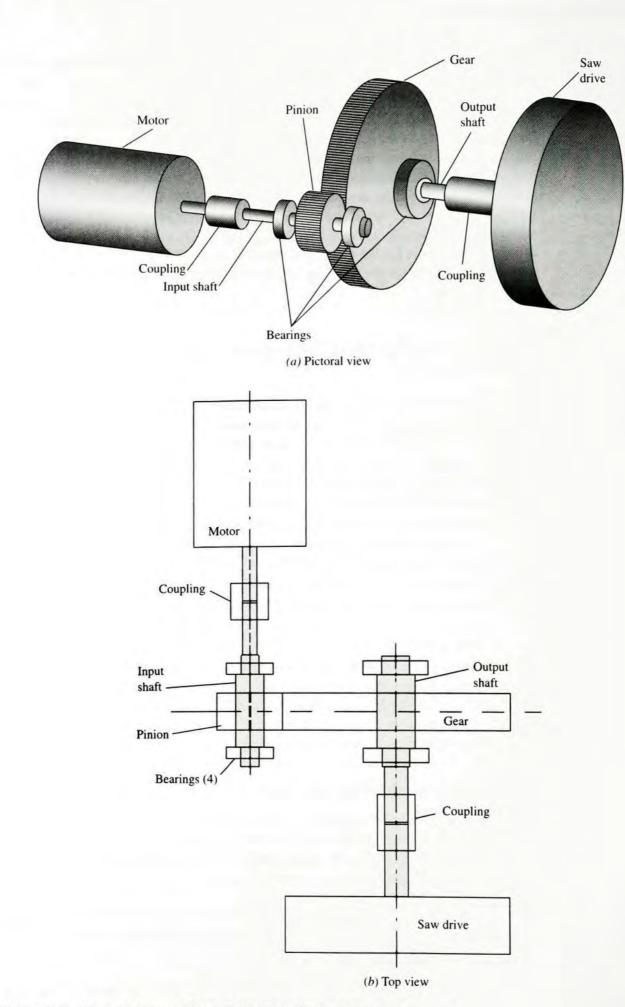
FIGURE 15-2 General layout of saw drive with single-stage gear reducer
