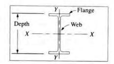
TABLE A16-3 Properties of steel wide-flange shapes, W-shapes\*
