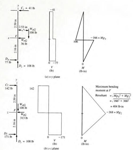
Bearing Reactions, Gear Shaft: Bearings C and D Using similar methods, we can find the forces in Figure 10–12.
