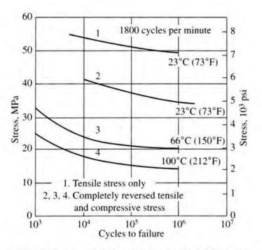
FIGURE 2-19 Fatigue stress vs. number of cycles to failure for an acetal resin plastic (DuPont Polymers, Wilmington, DE)
