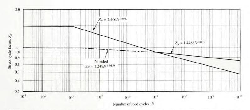
**FIGURE 9–24** Pitting resistance stress cycle factor,  $Z_N$  (Extracted from AGMA Standard 2001-C95, Fundamental Rating Factors and Calculation Methods for Involute Spur and Helical Gear Teeth, with permission of the publisher, American Gear Manufacturers Association, 1500 King Street, Suite 201, Alexandria, VA 22314)
