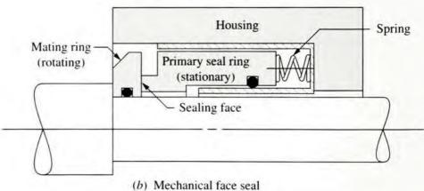
FIGURE 11–38 Seal for ball bearing
