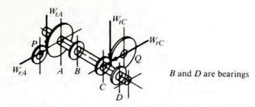
(a) Pictorial view of forces on gears A and C
