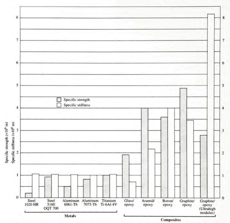
FIGURE 2-21 Comparison of specific strength and specific stiffness for selected metals and composites
