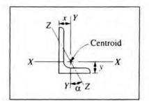
TABLE A16-1 Properties of steel angles, equal legs and unequal legs, L-shapes\*
