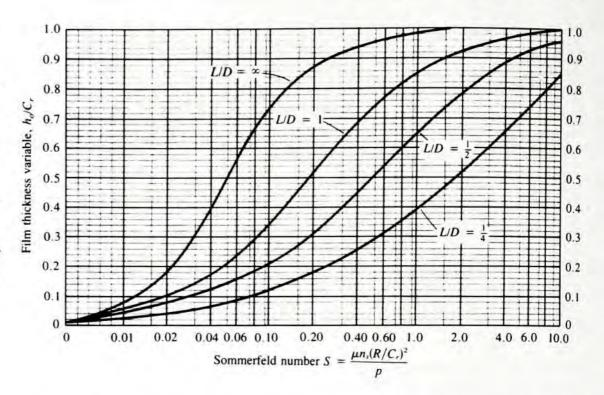
Note that S is similar to the bearing parameter,  $\mu n/p$ , discussed in Section 16–3, in that it involves the combined effect of viscosity, rotational speed, and bearing pressure. In order for S to be dimensionless, the following units should be used for the factors:
