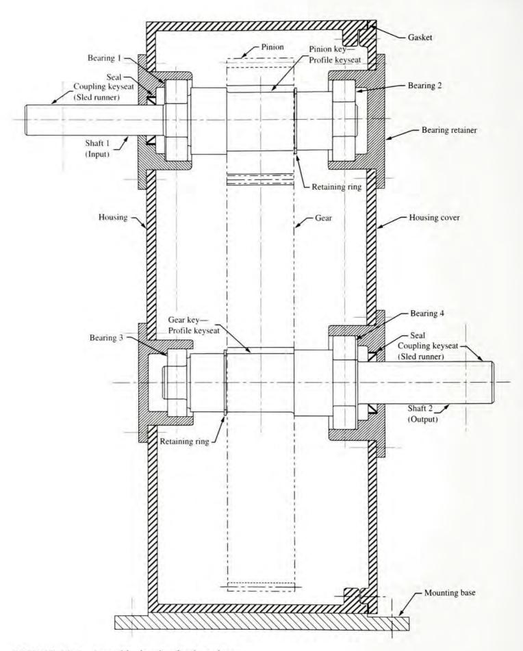
FIGURE 15-6 Assembly drawing for the reducer
