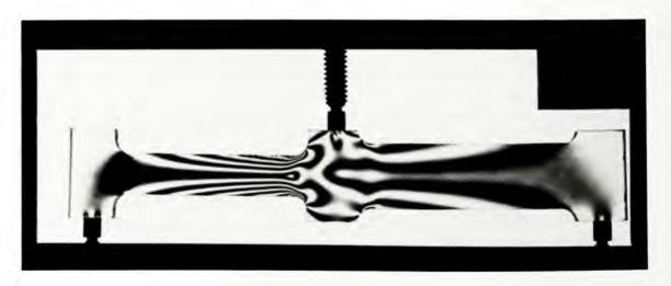
that the highest stress occurs in the fillet. Figure A15–2 gives data for the values of the stress concentration factor,  $K_t$ . The nominal stress,  $\sigma_{\text{nom}}$ , is computed from the classic flexure formula, and the section modulus is based on the smaller cross section near the fillet. These formulas are listed near the stress concentration chart.
