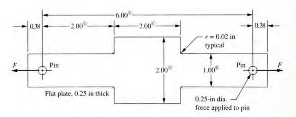
FIGURE P5-64 Beam for Problems 64 and 65
