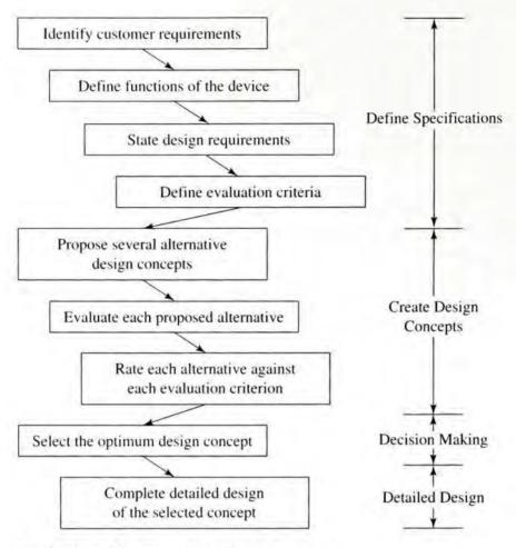
FIGURE 1-11 Steps in the design process
