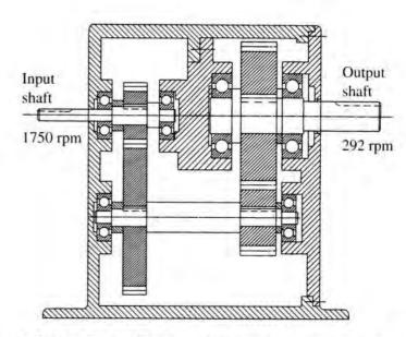
FIGURE 13-1 Conceptual design for a speed reducer
