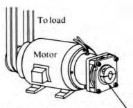
(d) Fail-safe brake: Stops load by de-energization of coil; power off – brake on.
