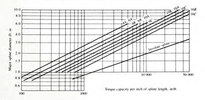
FIGURE 11-7 Torque capacity per inch of spline length, lb in
