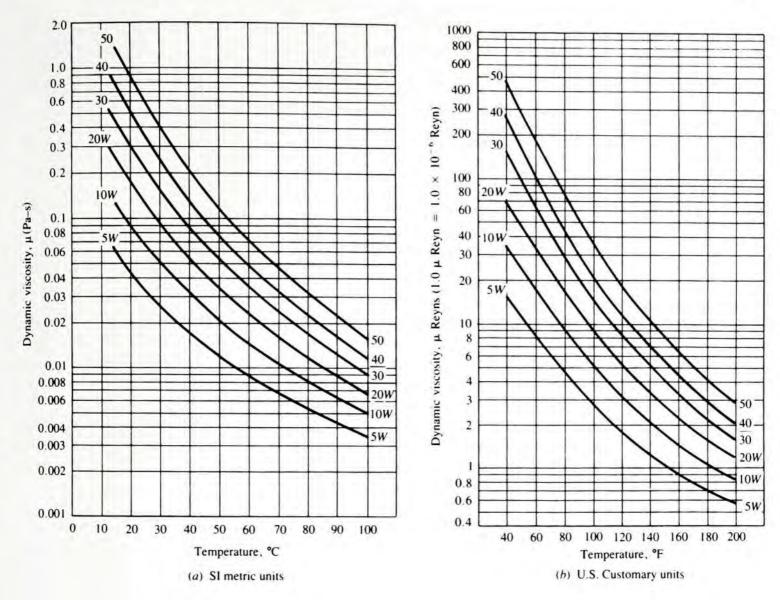
**FIGURE 16–6** Viscosity vs. temperature for SAE oils
