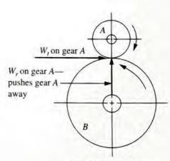
(b) Forces exerted on gear A by gear B. Reaction forces. Action: Driver pushes on driven gear Reaction: Driven gear pushes back on driver
