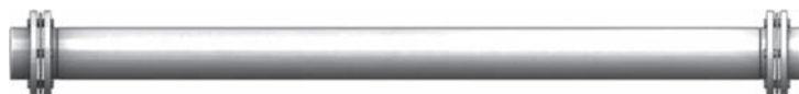
(d) General design of the coupling for each segment of the driveline
