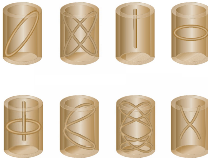
FIGURE 16–10 Examples of styles of grooving for plain bearings
