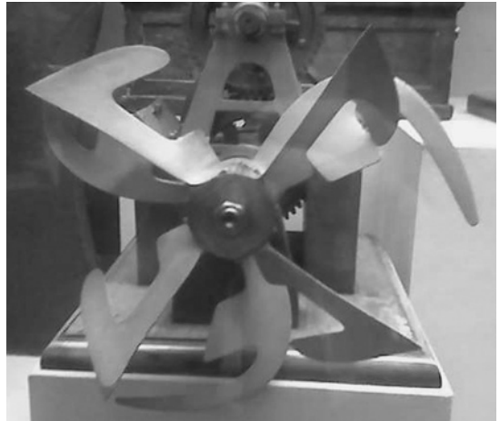
Figure 1.11 de Bay's contra-rotating propeller design
