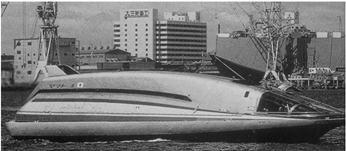
Figure 2.19 Yamato 1 : Experimental magnetohydrodynamic propulsion craft
