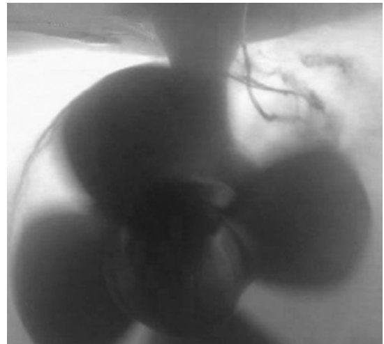
Figure 9.14 Example of a propeller–hull vortex emanating from a podded propulsion unit
