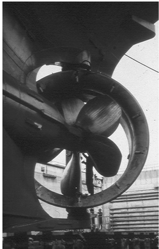
Figure 2.5 Steerable ducted propeller
