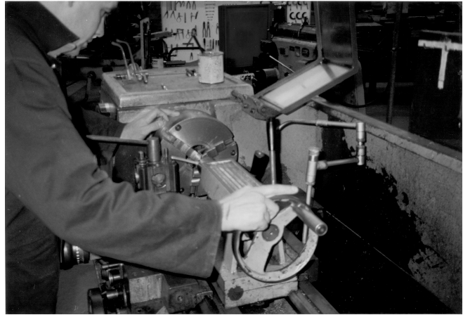
The set-up for hand tapping on a centre lathe
