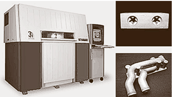
Fig. 7.327 Sinterstation HiQ System of 3-D Systems. Technical characteristics: materials: steels ST100, ST200 and A6; no full melting, infiltration required; layer thickness 70 \mu\text{m} ; accuracy 0.05–0.1 mm; build volume 330 \times 380 \times 457 mm; speed 50–80 \text{cm}^3/\text{h}
