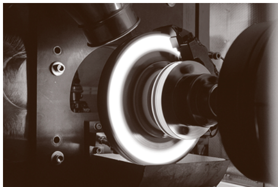
Fig. 13.50 Brake test on a testing machine (courtesy of Mercedes Car Group)
