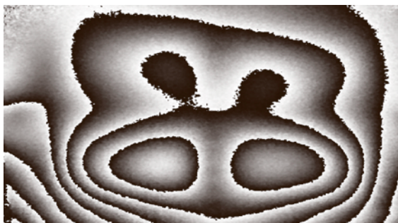
Fig. 3.99 Speckle fringes caused by discontinuities of off-plane surface displacements
