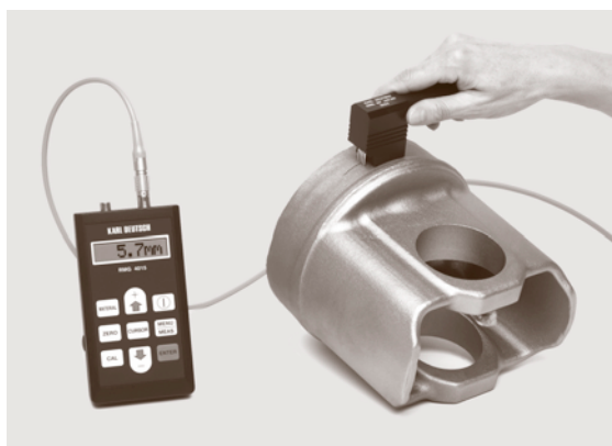
Fig. 3.85 Potential probes are able to measure crack depth and inclination
