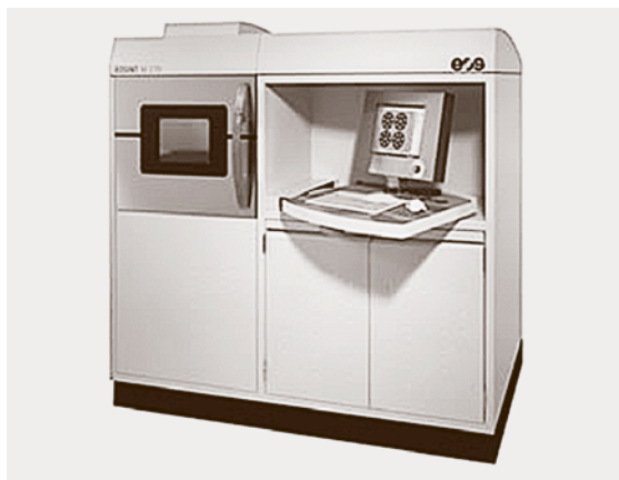
Fig. 7.334 EOSINT M270 – EOS device. Technical characteristics: materials: tool steel H20, steel DS20, Ti6AL4V, stainless steel EOS 17-4 PH, bronze DM20; full melting; layer thickness 20–100 \mu\text{m} ; accuracy 0.05–0.1 mm; build volume 250 \times 250 \times 215\text{ mm} ; speed 5–70 \text{cm}^3/\text{h}
