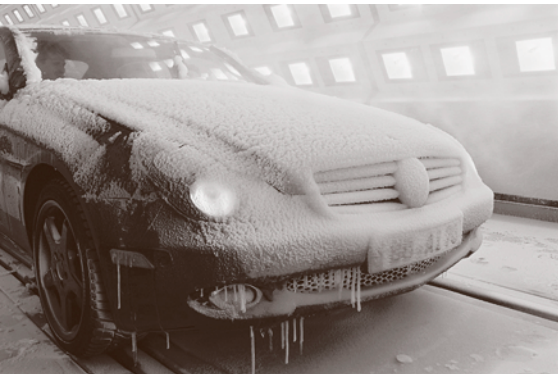
Fig. 13.85 Car test in climate chamber (courtesy of Mercedes Car Group)
