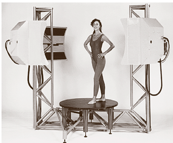
Fig. 7.349 Use of a three-dimensional scanner for clothing design (after [7.449])
