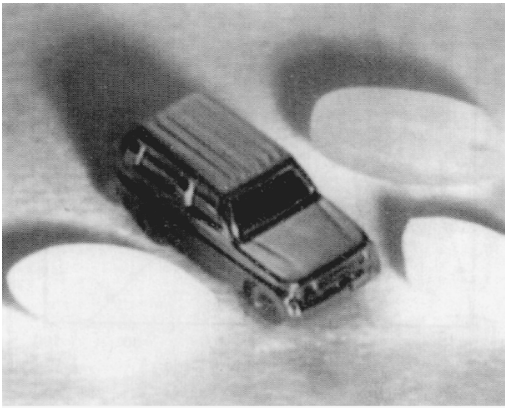
FIGURE 15.3.12 Micro car and rice grains ( left ) and micro-car on sandpaper (grain size = 200 mm) ( right ). The car is 7 mm long, 2.3 mm wide, and 3 mm high. (Source: A. Teshigahara, M. Watanabe, N. Kawahara, Y. Ohtsuka, and T. Hattori, J. Microelectromech. Syst. , 4, 76–80, 1995. With permission.)
