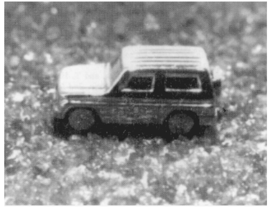
FIGURE 15.3.12 Micro car and rice grains ( left ) and micro-car on sandpaper (grain size = 200 mm) ( right ). The car is 7 mm long, 2.3 mm wide, and 3 mm high. (Source: A. Teshigahara, M. Watanabe, N. Kawahara, Y. Ohtsuka, and T. Hattori, J. Microelectromech. Syst. , 4, 76–80, 1995. With permission.)
