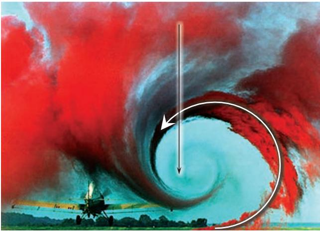
**FIGURE 9.122** Red smoke pulled into the low-pressure zone created on the back side of an airplane wing. (From NASA photograph, Washington, DC.)
