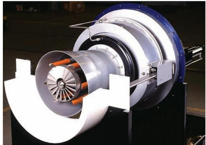
FIGURE 11.6 Cutaway view of the burner to be installed on the prototype.
