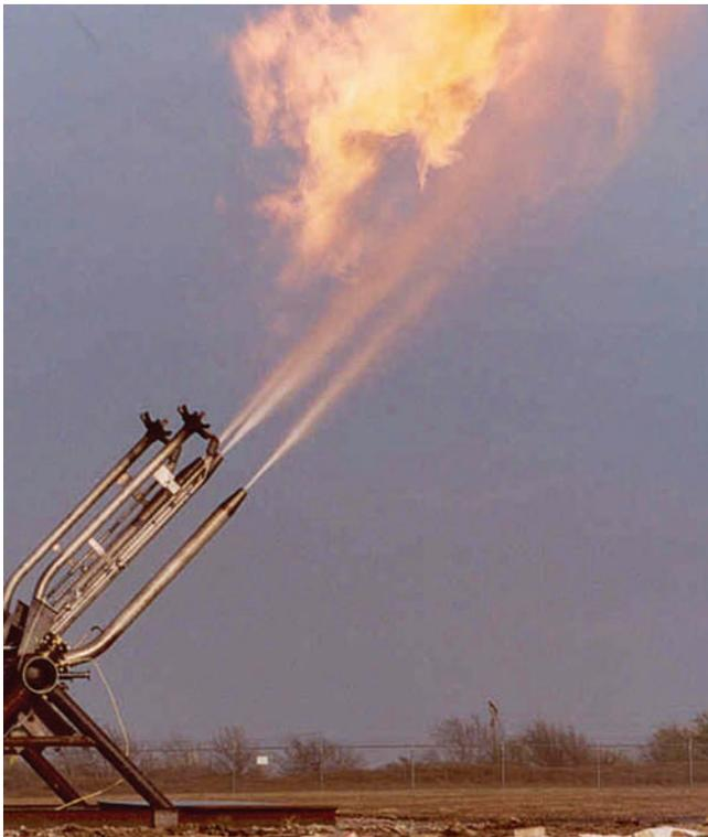
**FIGURE 16.36** Water injected into a high-pressure flare.
