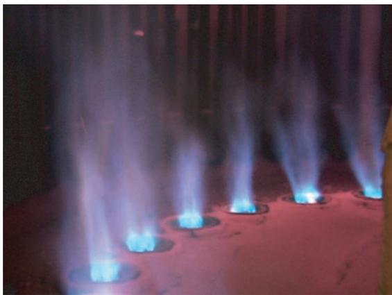
**FIGURE 9.119** Burners firing in a vertical-cylindrical (VC) heater showing no signs of flame–flame interactions.
