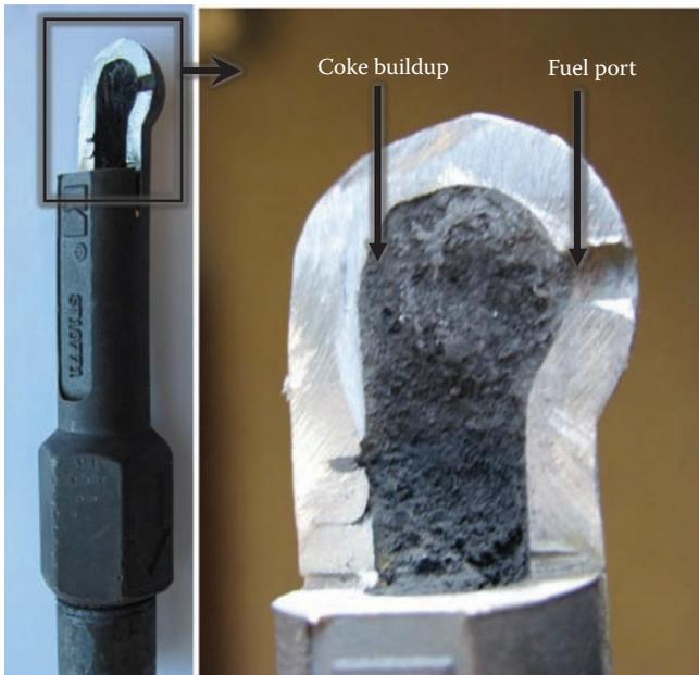
**FIGURE 9.96** Burner tip with coking on the inside.
