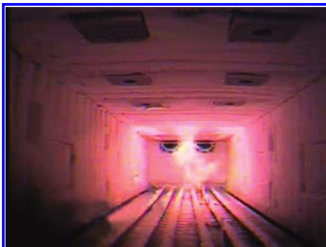
FIGURE 6.17 Example of flame rollover in a pilot-scale cracking furnace.
