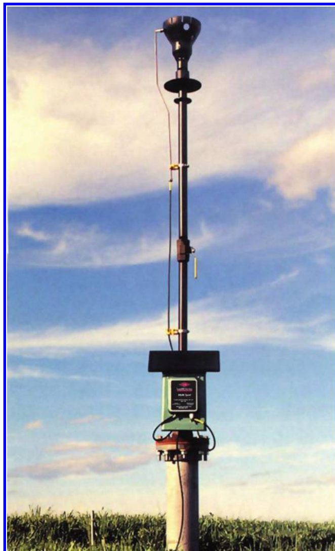
FIGURE 13.1 Solar powered passive flare. (Courtesy of Solar-Spark by LSC Environmental Products, LLC.)
