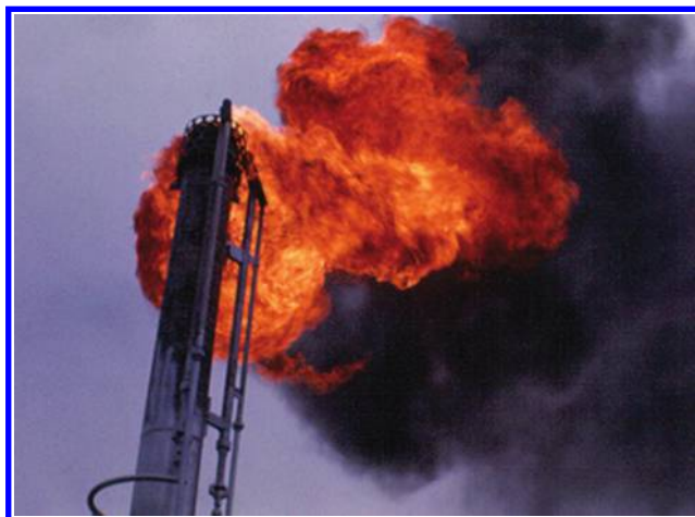
FIGURE 11.21 Typical nonassisted flare.
