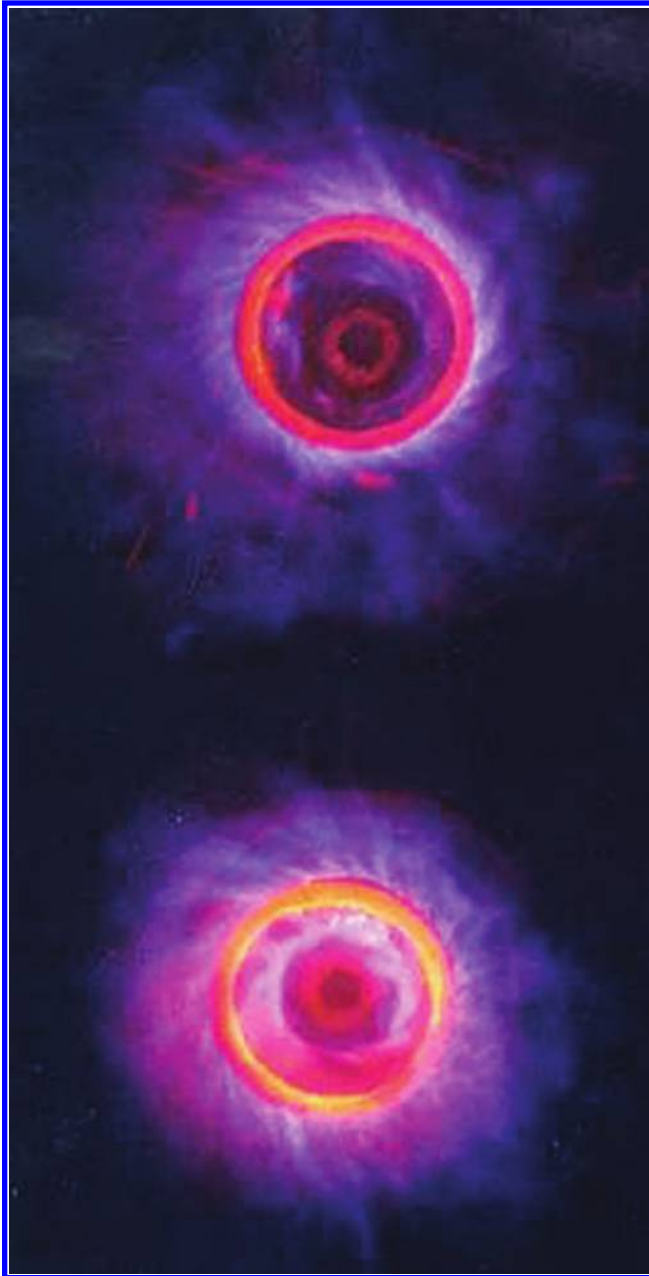
FIGURE 3.16 Enhanced images of the gas-fired RMB flame.
