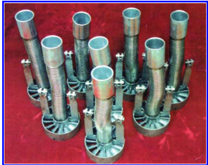
FIGURE 3.39 Spinners for tilting burners.
