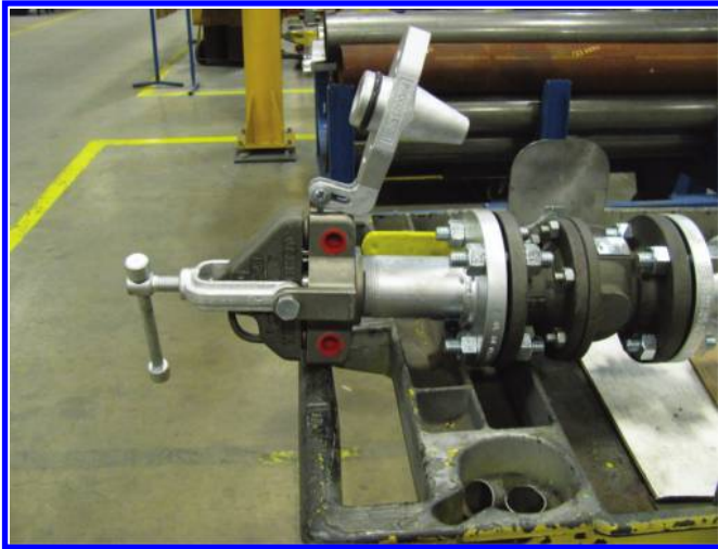
FIGURE 2.20 Oil gun insert and oil body receiver (with red caps).
