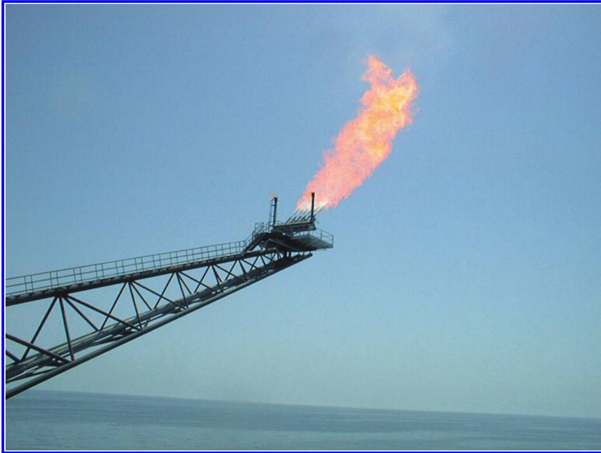
FIGURE 11.37 Poseidon flare: water-assisted Hydra.
