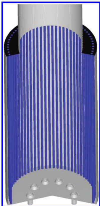
FIGURE 6.2 Vertical cylindrical furnace arrangement.
