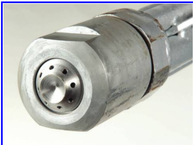
FIGURE 5.3 Heavy fuel-oil sprayer and twin-fluid Y-jet atomizer.
