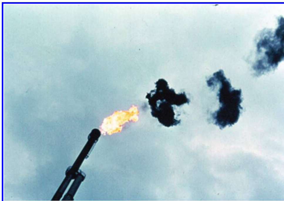
FIGURE 11.41 “Smoke signals” from a surging liquid seal.
