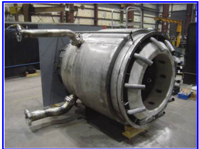
FIGURE 3.24 Modified Coen LCF burner for simultaneous low-NOx firing of multiple fuels of variable composition.
