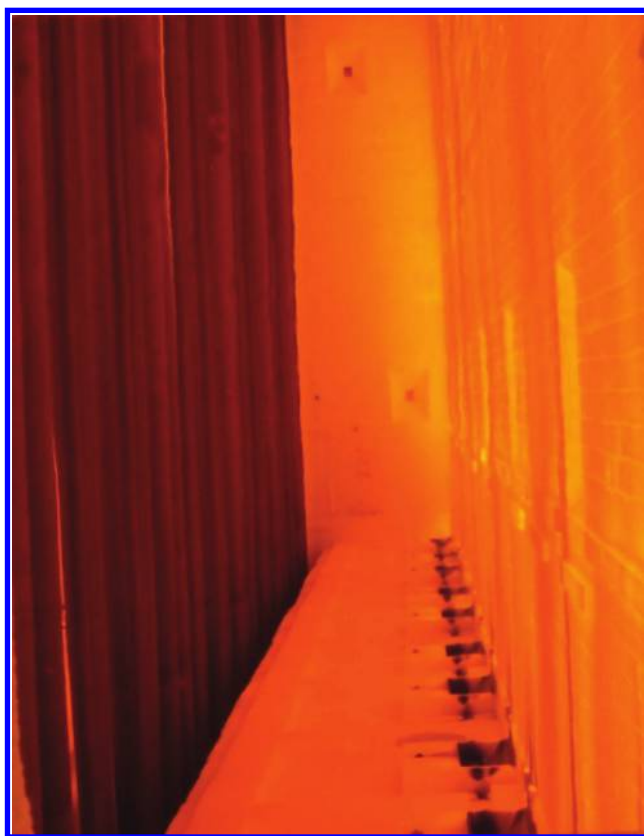
FIGURE 6.16 Large heat release floor burners.
