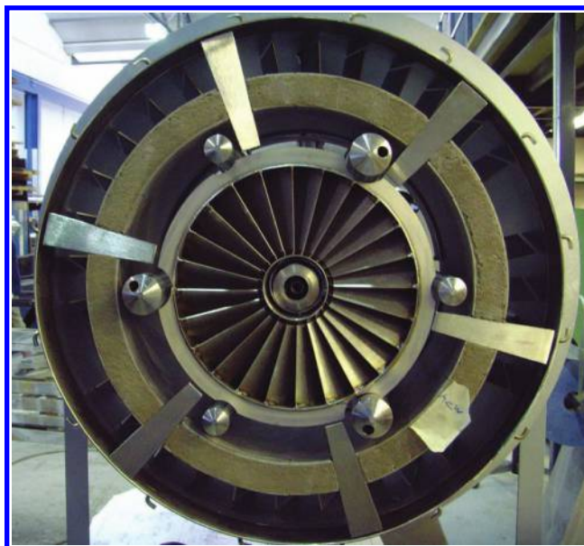
FIGURE 5.14 Hamworthy Combustion's DFL low- \text{NO}_x register burner.
