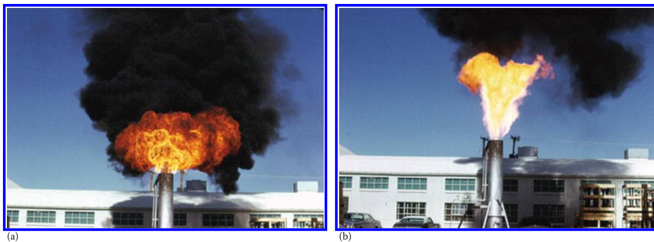
FIGURE 11.19 Effectiveness of air in smoke suppression: (a) no blower air and (b) start blower.
