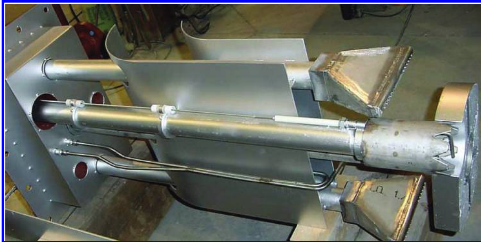
FIGURE 3.38 Main components of a fixed geometry burner for a gas and oil T-fired boiler.
