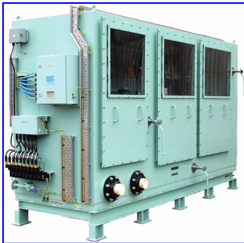
FIGURE 5.10 Fuel-gas valve enclosure for FPSO engine room boiler.
