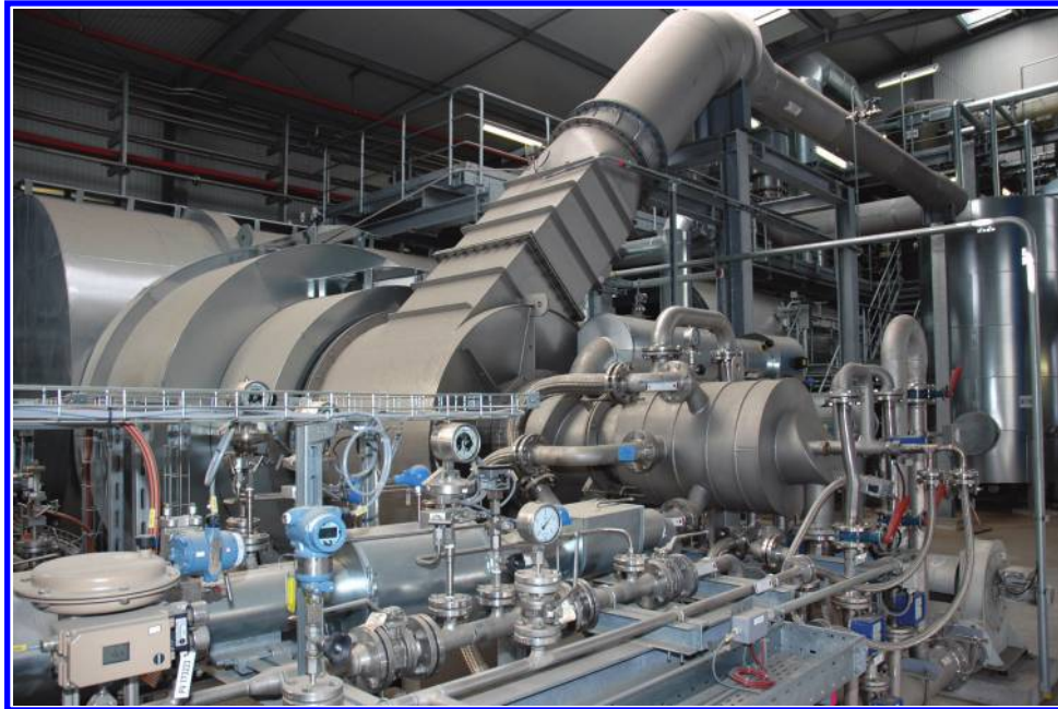
FIGURE 9.15 Combustor with a waste gas organ for explosive waste gas.
