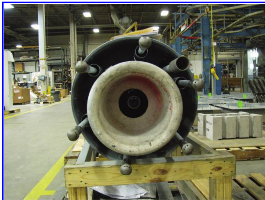
FIGURE 2.13 Regen oil tile with an oil gun in the center (secondary tile not shown).
