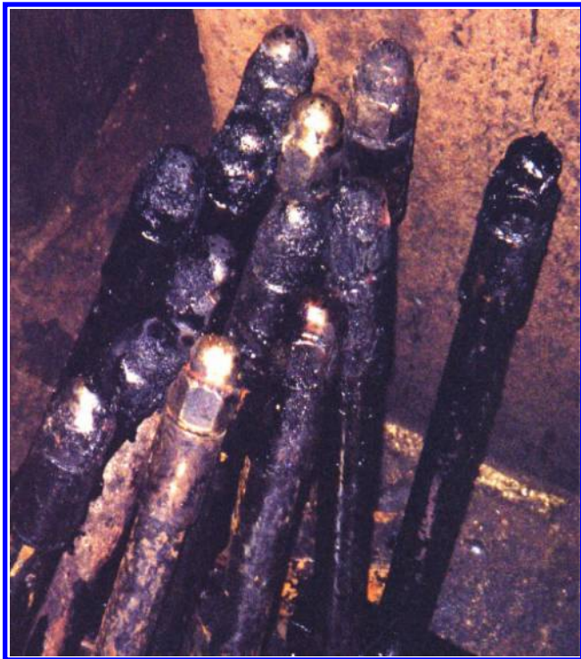
FIGURE 2.28 Fouled oil guns.
