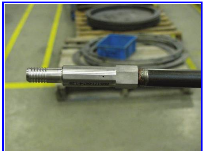
FIGURE 2.25 Atomizer with labyrinth seals and steam ports.
