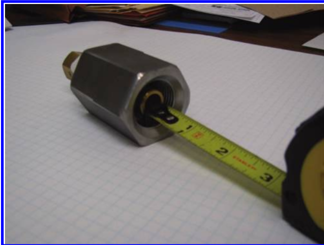
FIGURE 2.26 Checking atomizer location in the sleeve.
