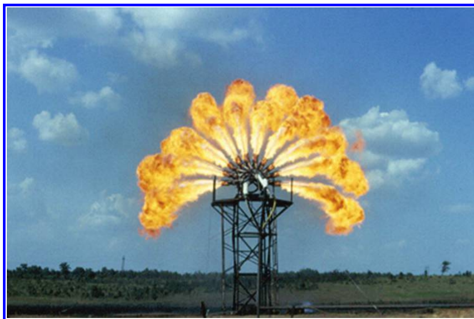
FIGURE 11.35 OWB liquid flare test firing 150 gpm (570 L/min).
