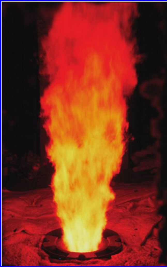
FIGURE 2.6 Round burner tile provides round oil flame.
