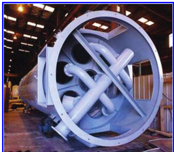
FIGURE 13.8 Enclosed flare gas manifold.
