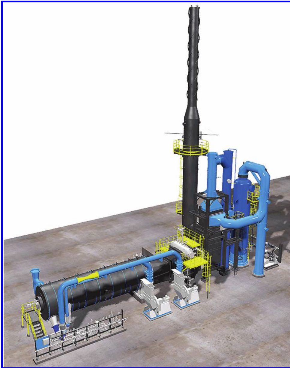
FIGURE 8.1 Example of a comprehensive thermal oxidizer system.
