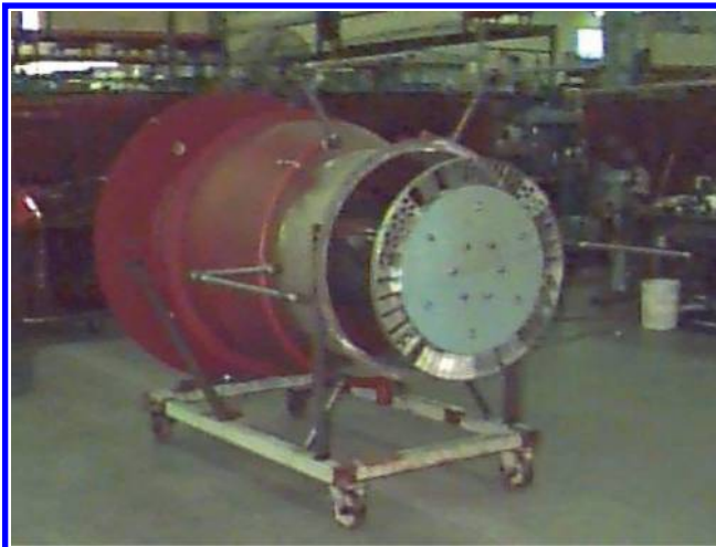
FIGURE 3.21 Assembled Coen QLA burner (front).
