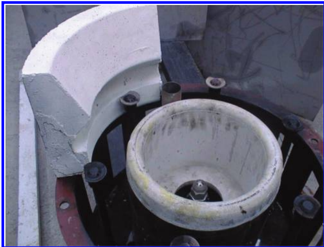
FIGURE 2.12 Regen tile and one section of secondary tile.
