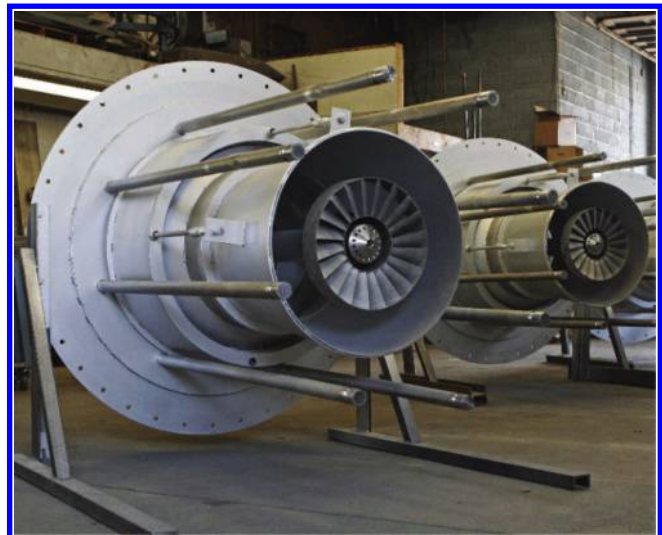
FIGURE 3.10 ECOjet ® gas-only burners.
