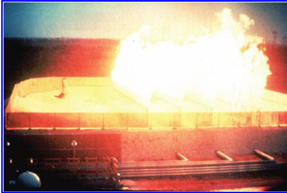
FIGURE 11.32 (continued) LRGO staging sequence during a flaring event from inception (a) to full load (g).
