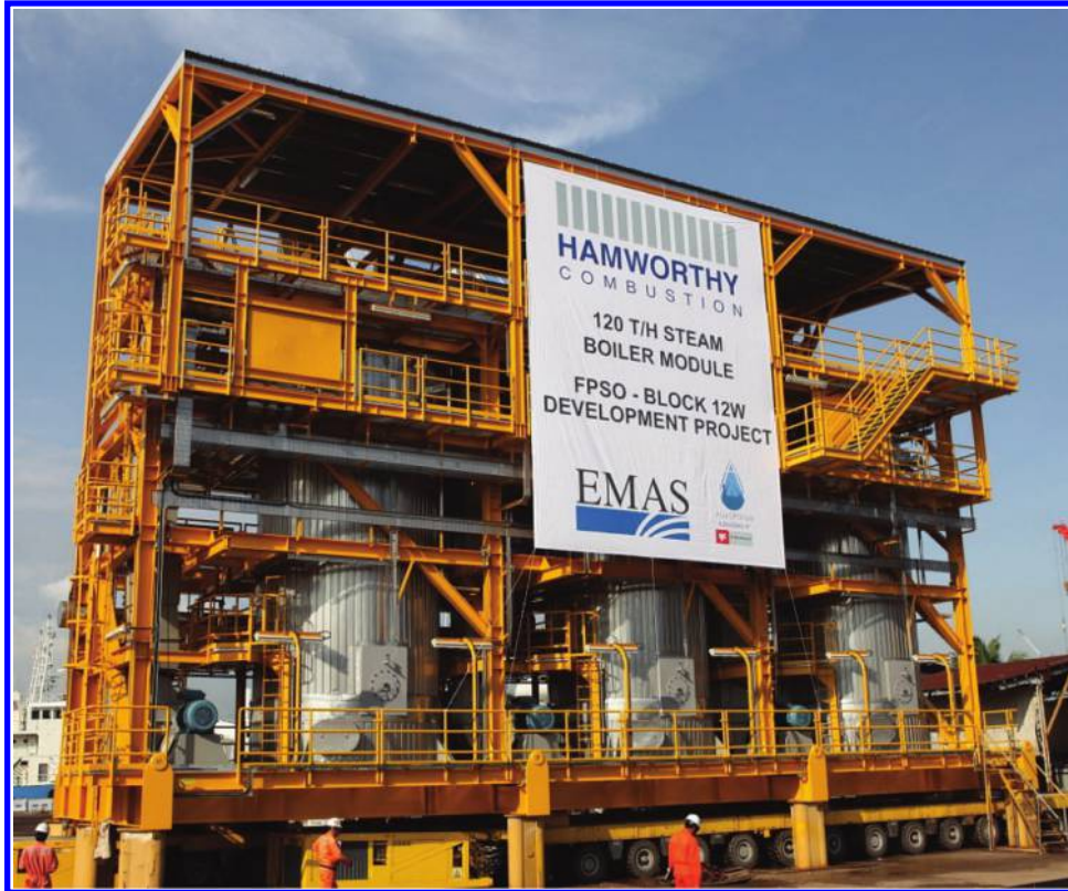
FIGURE 5.11 Hamworthy Combustion's triple 120 metric-ton/h (132 U.S. ton/h) steam boiler module for FPSO.
