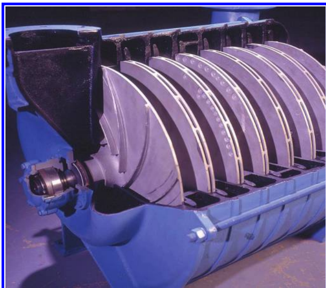
FIGURE 13.20 A cutaway of a multistage blower showing eight impellers. This blower is an eight-stage machine.
