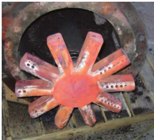
FIGURE 11.70 Spider with severe oxidation from overheating.
