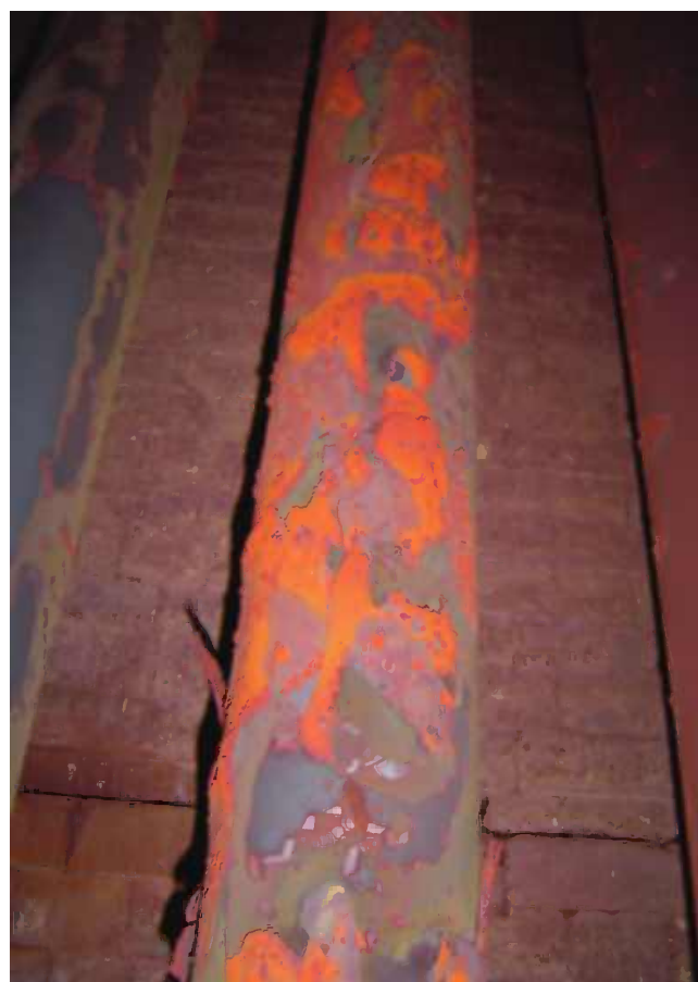
FIGURE 12.29 Tube scale due to flame impingement.
