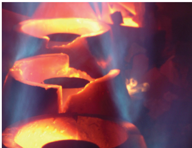
FIGURE 11.77 Burner tile with large broken pieces.
