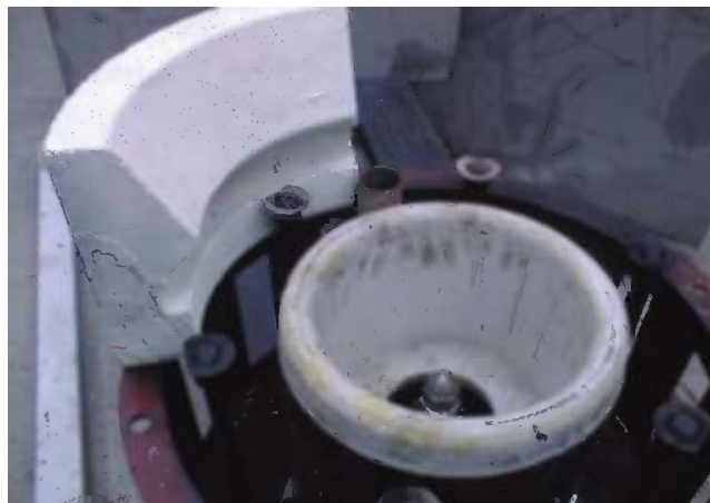
FIGURE 13.56 Oil gun in center of Regen (oil) tile (burner partially assembled).
