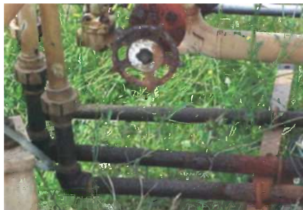
FIGURE 4.8 Corrosion of carbon steel process equipment located along the Texas coastline.
