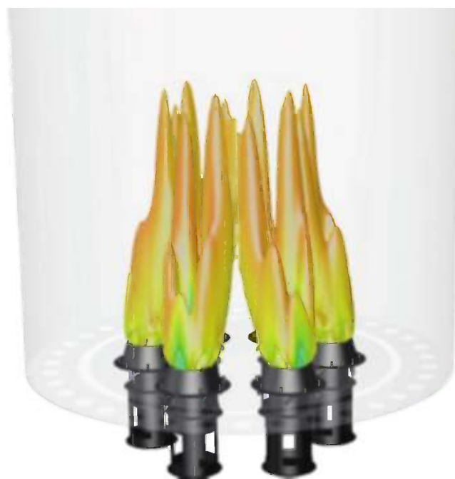
FIGURE 13.41 CFD model shows flames merging as a result of a tight spacing.
