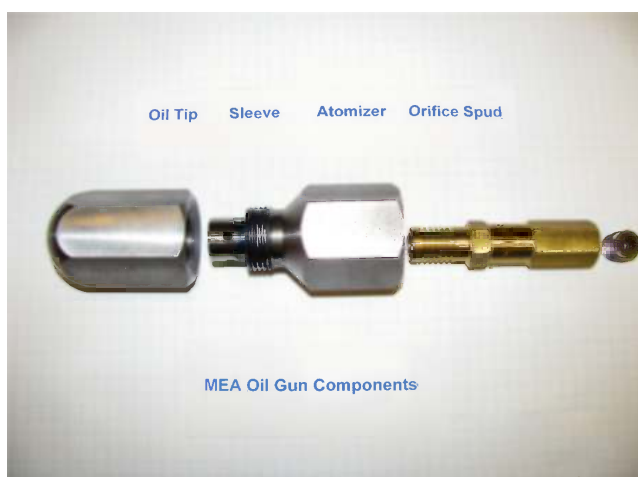
FIGURE 11.122 MEA oil gun parts.
