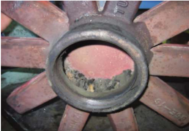
FIGURE 11.71 HEVD spider with internal fouling.
