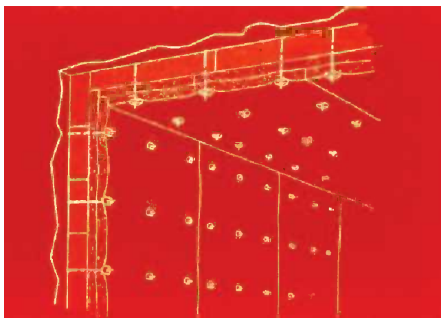
FIGURE 5.16 Illustration of anchors penetrating through refractory.
