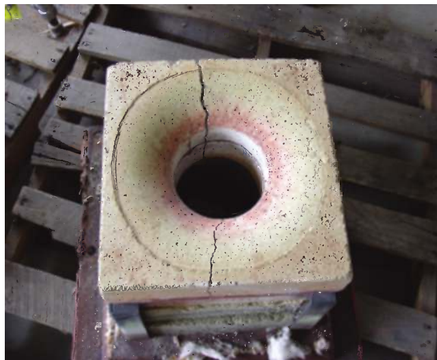
FIGURE 11.80 Radiant wall burner tile that should be replaced.
