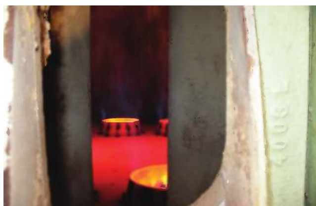
FIGURE 12.34 Uniform flames and refractory color.
