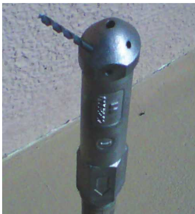
FIGURE 11.58 Checking ports with correct sized drill bit.
