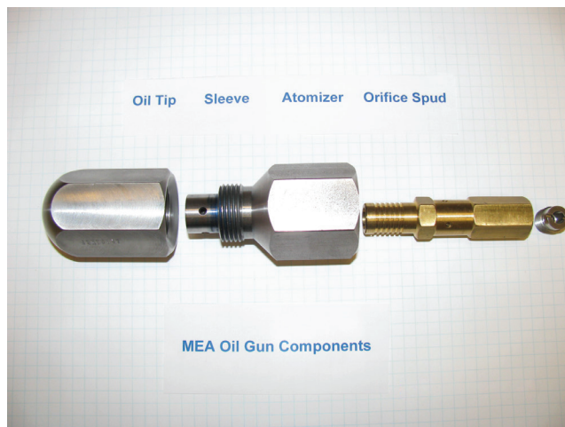
FIGURE 13.61 Typical oil gun components.
