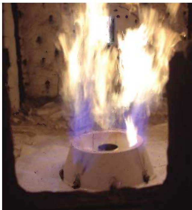
FIGURE 13.51 Poor mixing due to low fuel pressure.
