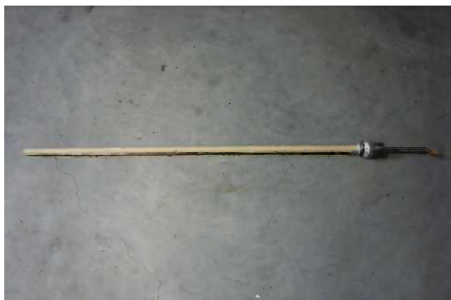
FIGURE 10.13 Ceramic-sheathed thermocouple. A stainless steel type K thermocouple is sheathed with a ceramic thermowell. This is the most common instrument for measuring temperature in a thermal oxidizer.
