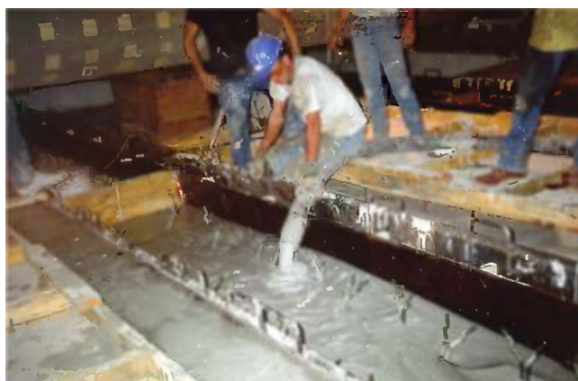
FIGURE 5.38 Example of poured refractory in a mold.
