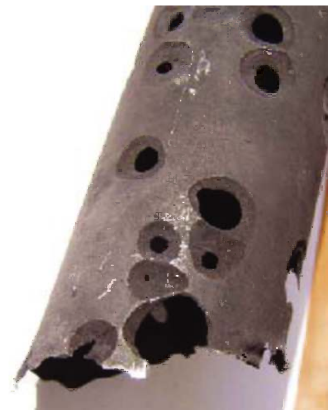
FIGURE 4.9 Metal dusting on an inlet tube of a heat exchanger unit. The material is alloy 800. (From Hrivnak, I. et al., Kovove Materialy , 43, 290, 2005.)
