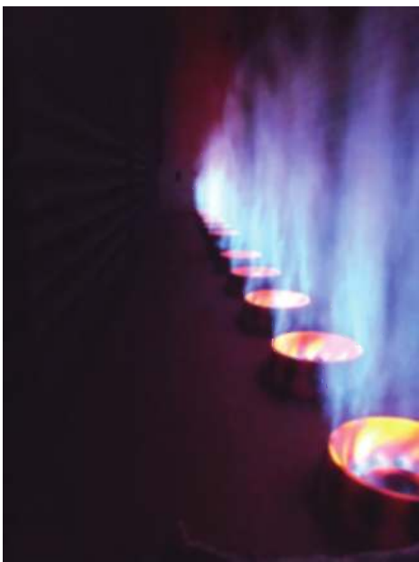
FIGURE 13.44 Cold firebox operation (floor and walls are darker in color).
