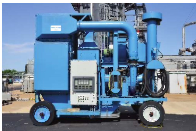
FIGURE 8.5 Self-contained, portable combustion air heater and blower used for testing forced draft, preheated air burner designs.
