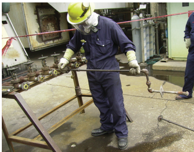
FIGURE 11.56 Using steam to blow out the gas riser/tip assembly.
