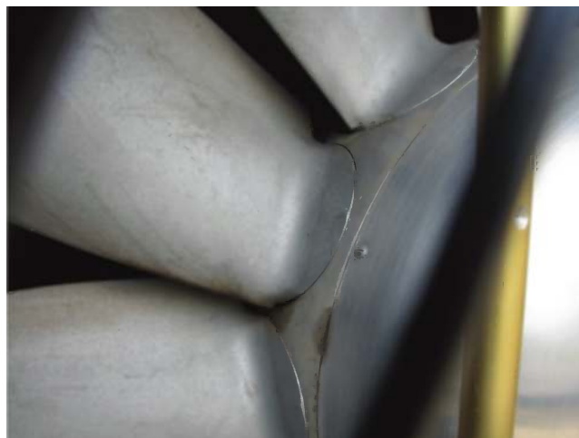
FIGURE 3.20 Close-up of variable pitch blades on a vane axial fan.
