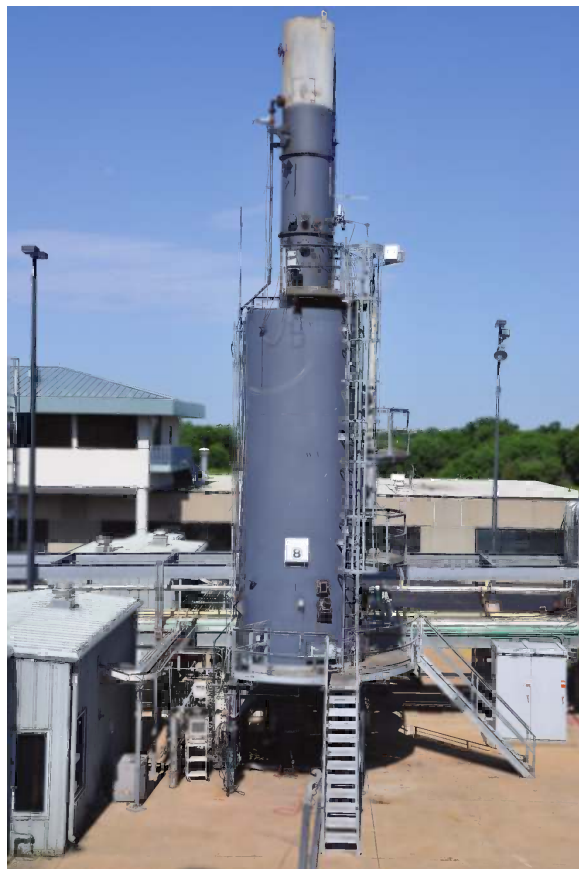
FIGURE 8.4 Vertical cylindrical furnace for freestanding, upfired burner tests.
