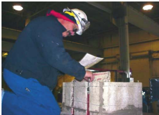
FIGURE 11.87 Checking gas tip orientation.
