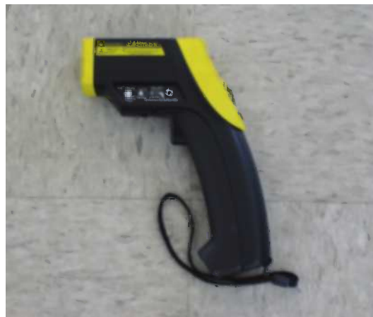
FIGURE 10.14 Handheld radiometer. This radiometer is equipped with the HeNe laser used for sighting. The radiometer quantifies the temperature of the sight point. Note that the emissivity of the material at the sight point must be known.
