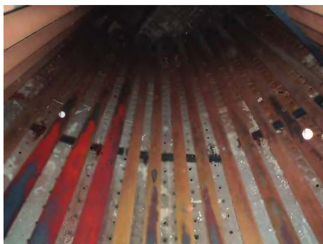
FIGURE 12.27 Process tube fouling due to flame impingement.
