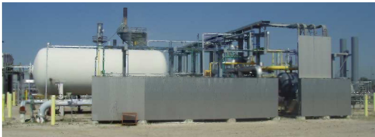
FIGURE 1.6 Stainless steel fence shielding flow control equipment from thermal radiation during flare testing. (From Baukal, C., Testing safety, in Industrial Combustion Testing , C.E. Baukal, ed., Chapter 2, Fig. 2.5, CRC Press, Boca Raton, FL, 2011.)
