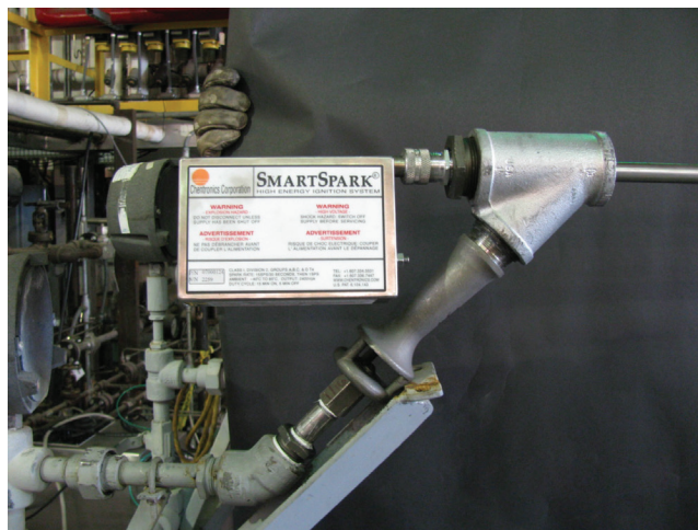
FIGURE 11.144 New pilot with an internal high-energy igniter system.
