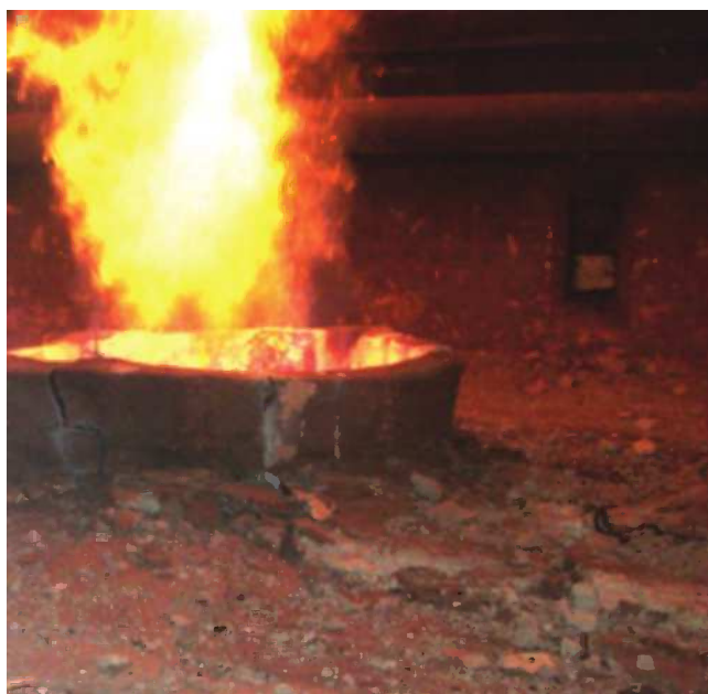
FIGURE 11.79 Tile crumbling and coming apart.
