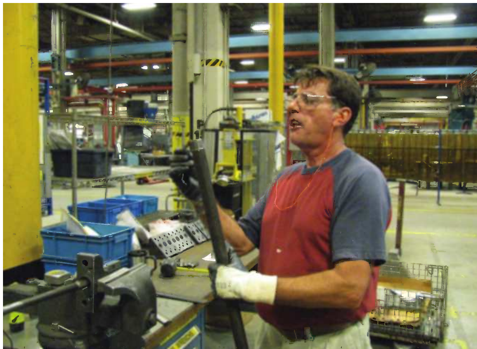
FIGURE 11.127 Applying high-temperature anti-seize to oil gun threads.
