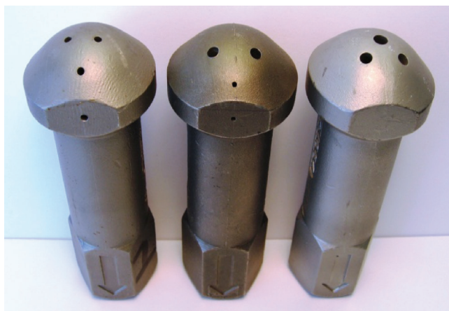
FIGURE 11.3 Gas tips with different drill patterns.
