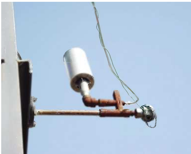
FIGURE 1.20 Cylindrical muffler on a suction pyrometer. (From Baukal, C.E., Industrial Combustion Pollution and Control , Fig. 10.25, Marcel Dekker, New York, 2004.)
