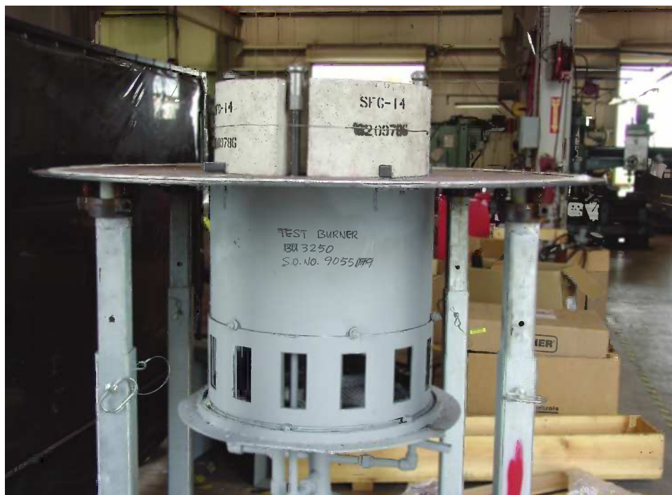
FIGURE 11.20 Burner designed to be mounted in a common plenum.
