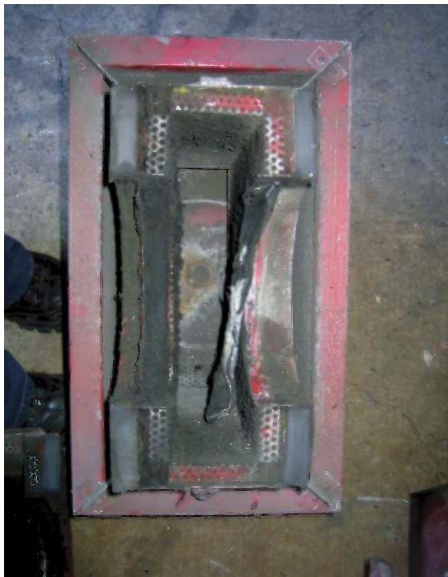
FIGURE 11.75 Worn gasket and dirty insulation.
