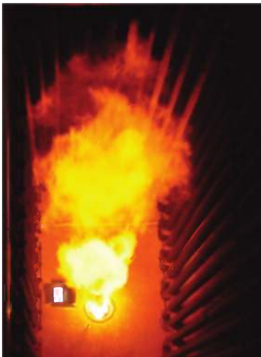
FIGURE 13.26 Flames short of air.
