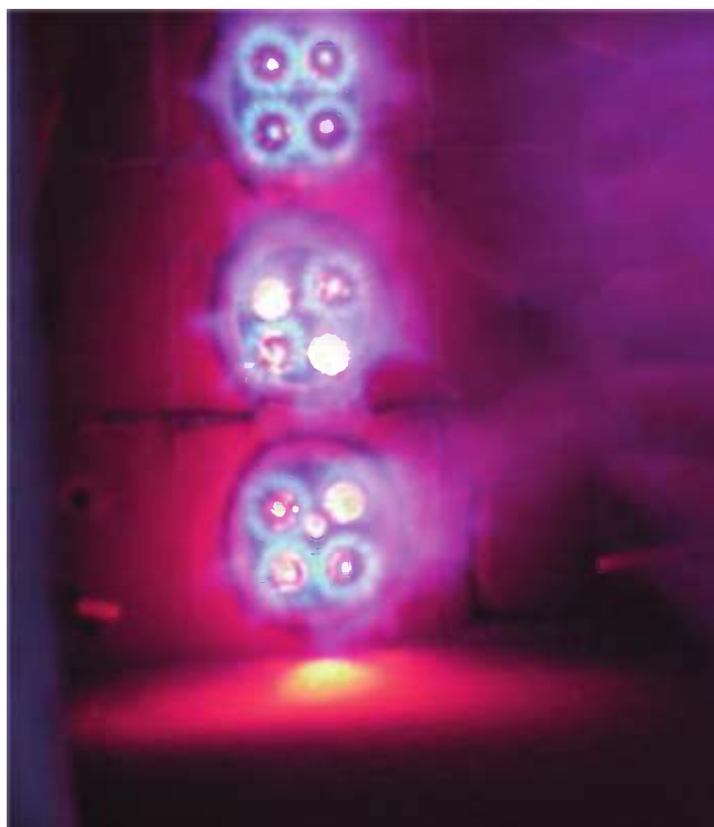
FIGURE 13.30 Gas tips glowing due to flashback.
