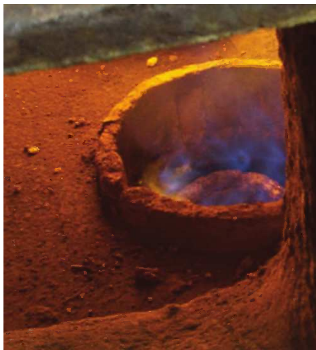
FIGURE 11.81 Vanadium attack on burner tile.
