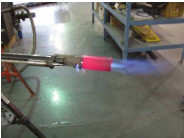
FIGURE 11.141 New-style pilot with no exposed insulators.
