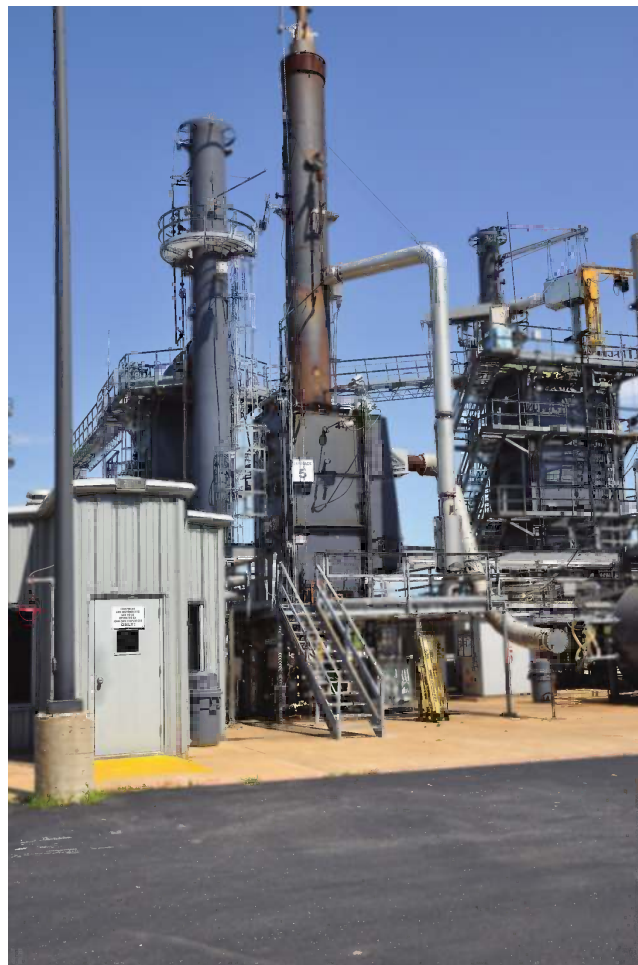
FIGURE 8.3 Test furnace capable of simulating terrace wall-fired heaters.
