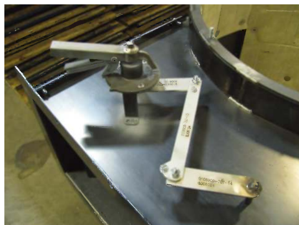
FIGURE 11.103 Damper linkage for dual-bladed opposed motion design.
