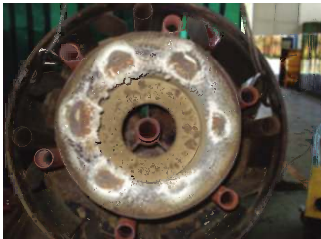
FIGURE 13.62 Vanadium attack on burner tile.
