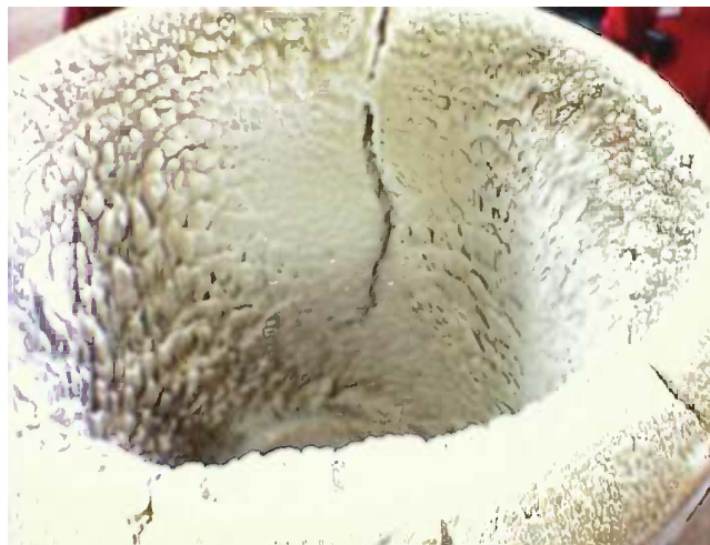
FIGURE 13.63 Catalyst buildup on oil tile.
