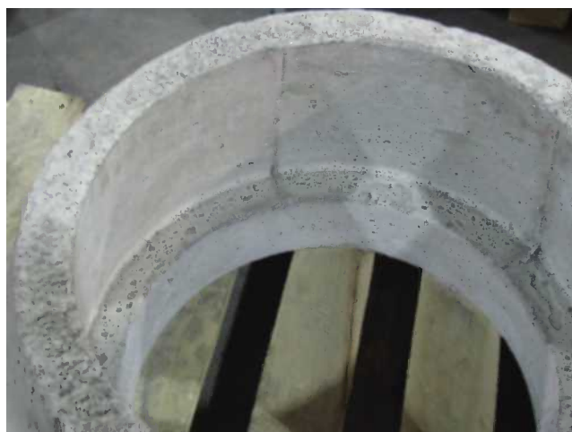
FIGURE 11.91 Burner tile ledge used to stabilize the flame.
