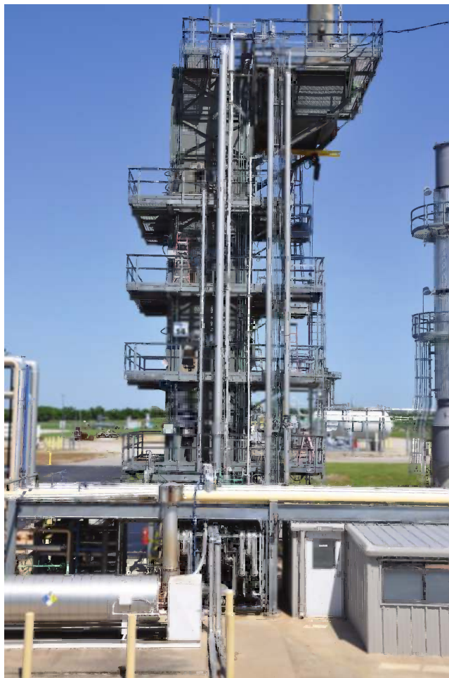
FIGURE 8.2 Test furnace used primarily for ethylene applications.
