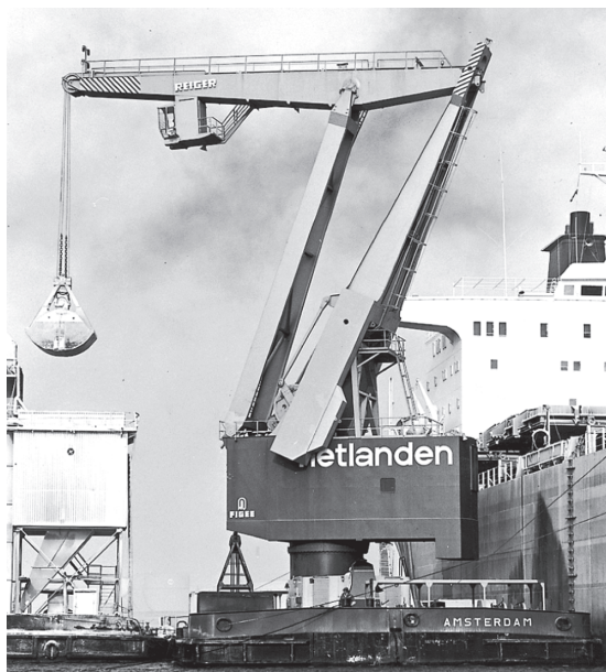
Figure P11.13 (a) Photograph; (b) R_{AO_2} = 14.7 m, R_{BA} = 6.5 m, R_{BO_4} = 19.3 m, R_{CA} = 22.3 m, R_{CB} = 16 m, and R_{O_2O_4} = -6.4\hat{i} + 5.3\hat{j} m. (Courtesy of B.V. Machinefabriek Figeo, Haarlem, Holland).
