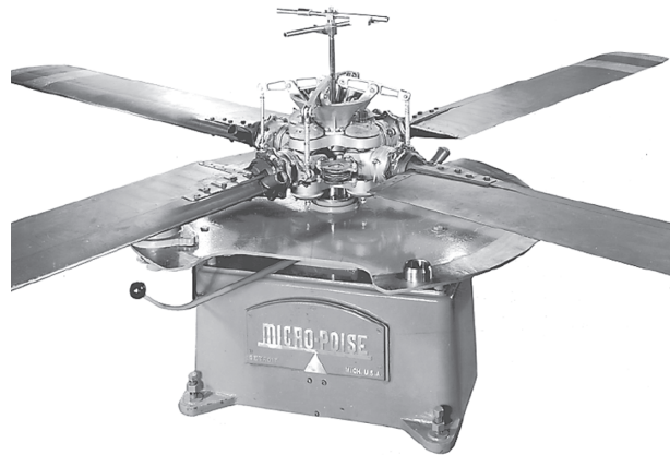
Figure 15.4 Aircraft propeller assembly balancer. (Courtesy of Schenck Ro Tec Corporation, Auburn Hills, MI.)
