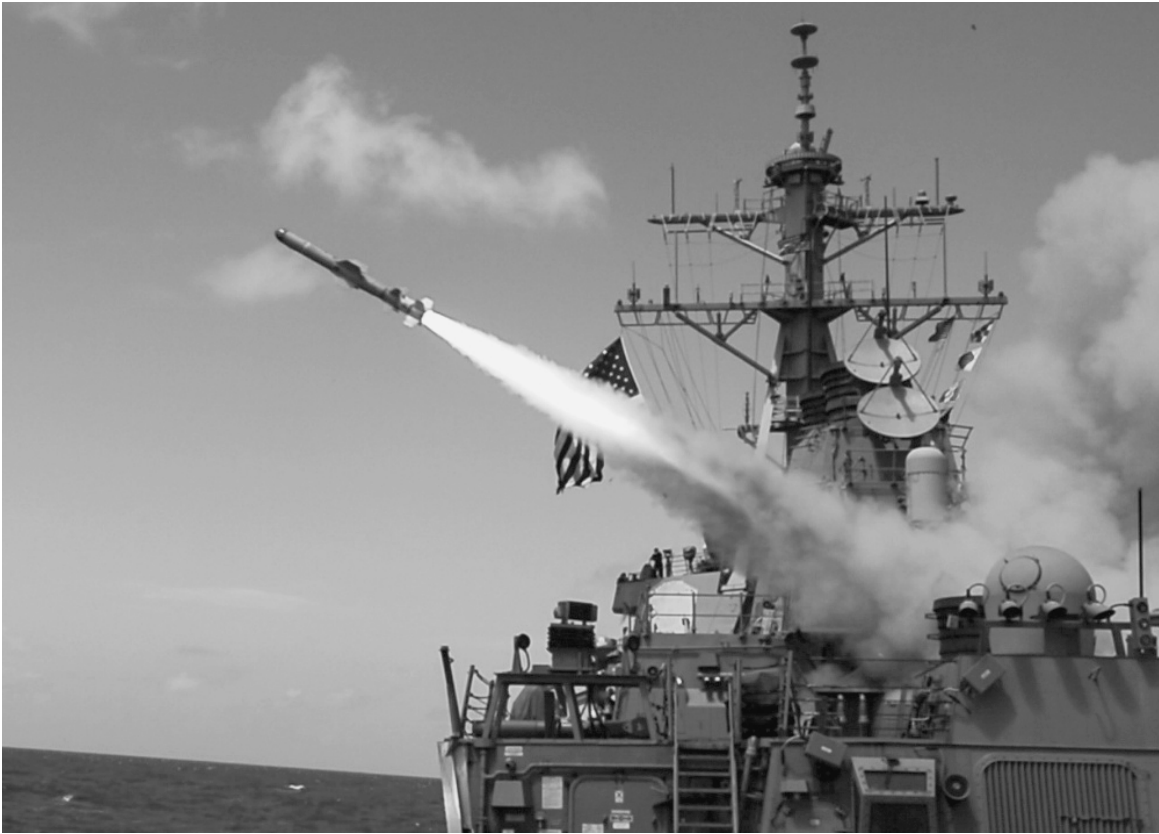
The destroyer USS Fitzgerald fires a Harpoon missile during a joint training exercise with Japan, 2016. The Harpoon is a fire-and-forget semiautonomous anti-ship missile. The human chooses the enemy ship to be destroyed and the missile uses automation to avoid other nearby ships. Missiles of this type are in widespread use around the world and have been used for decades.
