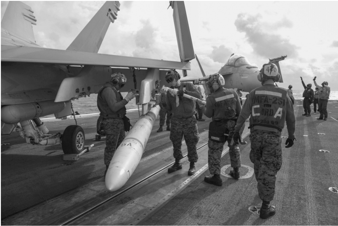
U.S. Marines remove a training AGM-88 High-Speed Anti-Radiation Missile (HARM) from an F/A-18C Hornet on the deck of the USS Theodore Roosevelt aircraft carrier, 2015. The HARM is a fire-and-forget semiautonomous homing missile used to destroy enemy radars.
