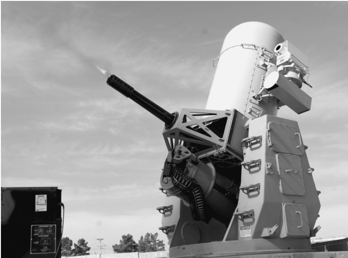
A Counter Rocket, Artillery, and Mortar (C-RAM) system from the 2nd Battalion, 44th Air Defense Artillery Regiment at Bagram Airfield in Afghanistan. The C-RAM, which has a high degree of automation but also retains a human in the loop, is an example of the kind of “centaur” human-machine teaming that Bob Work has advocated for.
