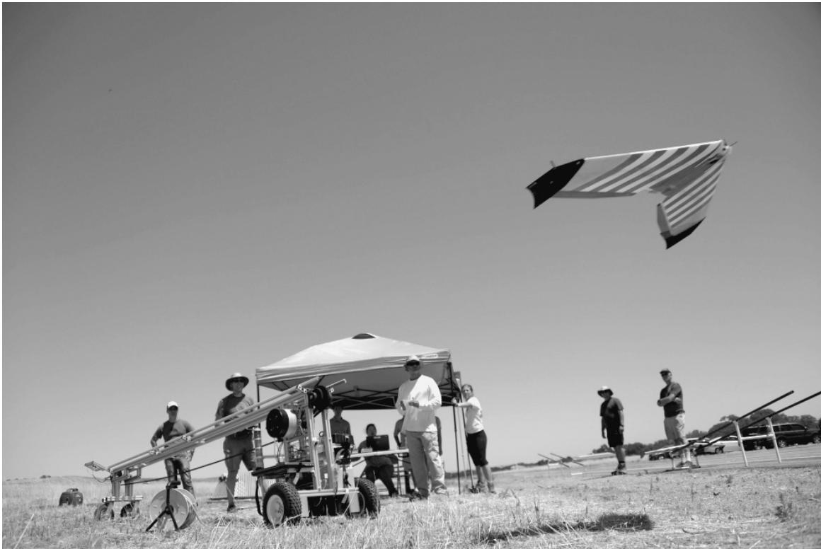
Researchers from the Naval Postgraduate School (NPS) launch a small drone as part of a thirty-drone swarm at Camp Roberts, California, 2015. Researchers at NPS are experimenting with swarm versus swarm combat, exploring new tactics for how to control friendly swarms and how to defeat enemy swarms.
