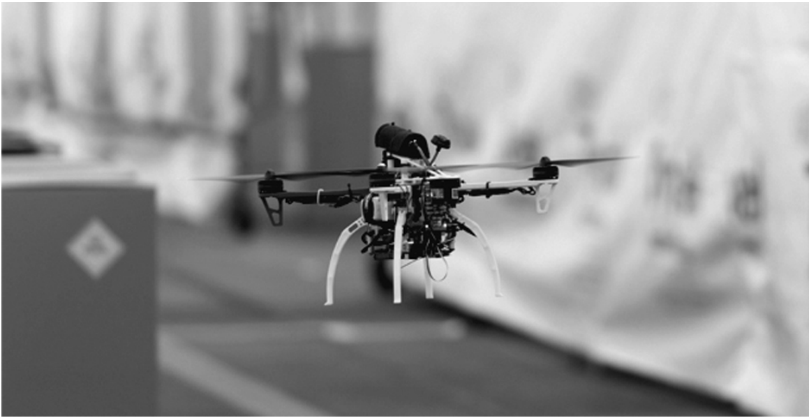
A modified quadcopter autonomously navigates through a warehouse as part of DARPA's Fast Lightweight Autonomy (FLA) program, 2016. FLA quadcopters use onboard sensors to detect the surrounding environment and autonomously navigate through cluttered terrain.
