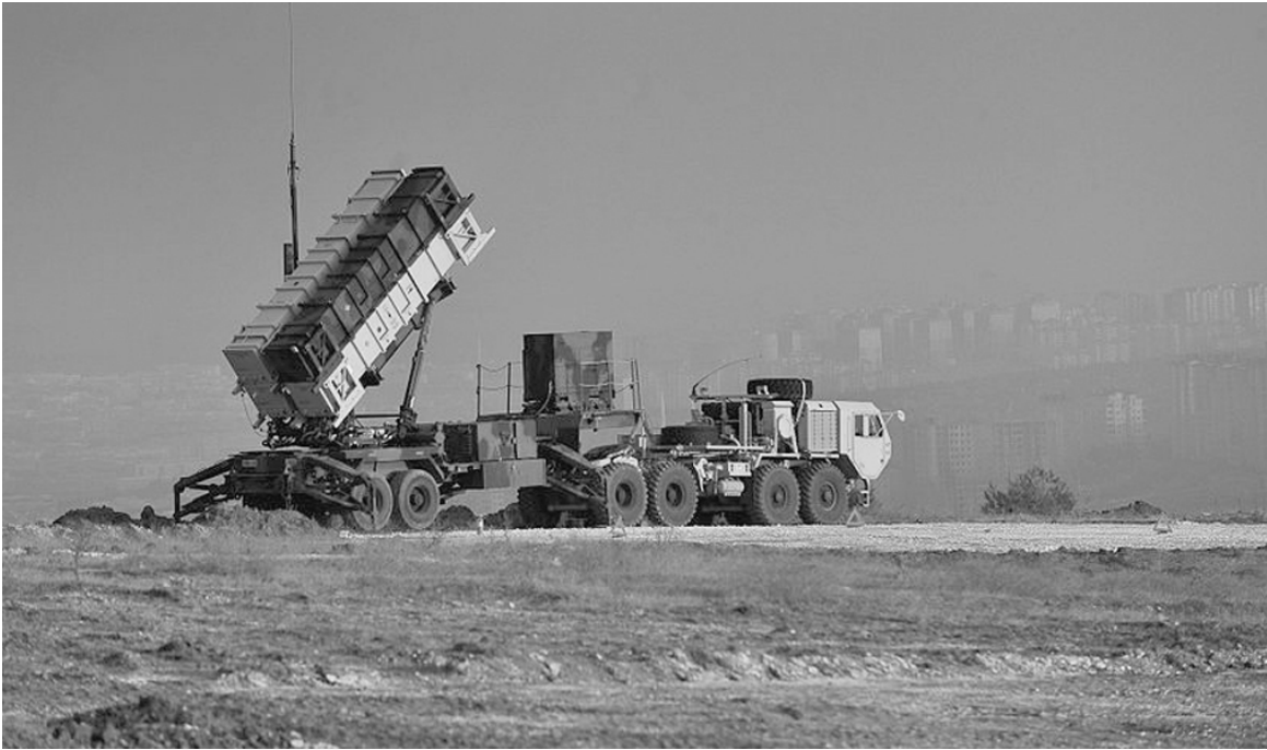
A U.S. Army Patriot battery along the Turkey-Syria border, 2013. U.S. Patriot batteries were deployed to Turkey to aid in defending Turkey during the Syrian civil war. The Patriot, a land-based supervised autonomous air and missile defense system, was involved in two fratricide incidents in 2003 that highlighted some of the dangers of automation in weapon systems.
