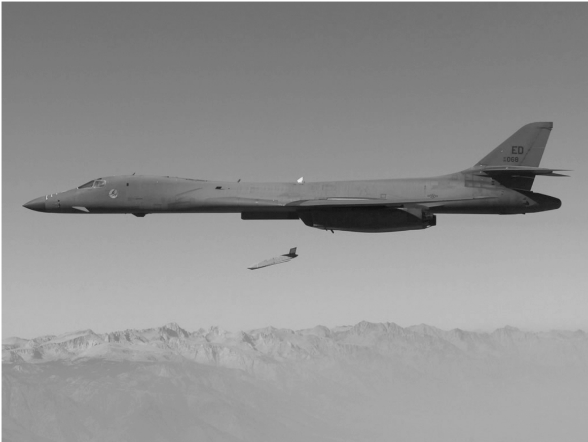
A B-1B bomber launches a Long-Range Anti-Ship Missile (LRASM) in a flight demonstration, 2013. The semiautonomous LRASM incorporates a number of advanced autonomous guidance features that allow it to avoid pop-up threats while en route to its human-designated target.
