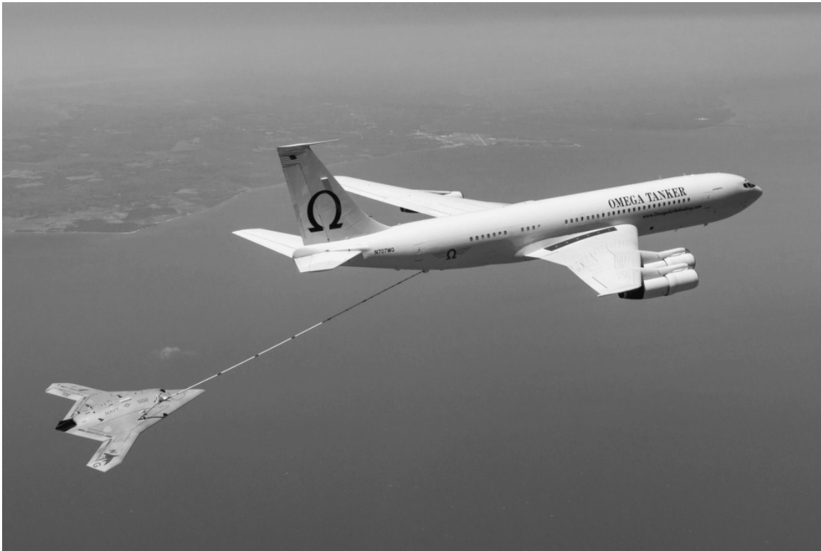
The X-47B autonomously refuels from a K-707 tanker over the Chesapeake Bay, 2015, demonstrating the first aerial refueling of an uninhabited aircraft. Autonomous aerial refueling is an important enabler for making uninhabited combat aircraft operationally relevant.
