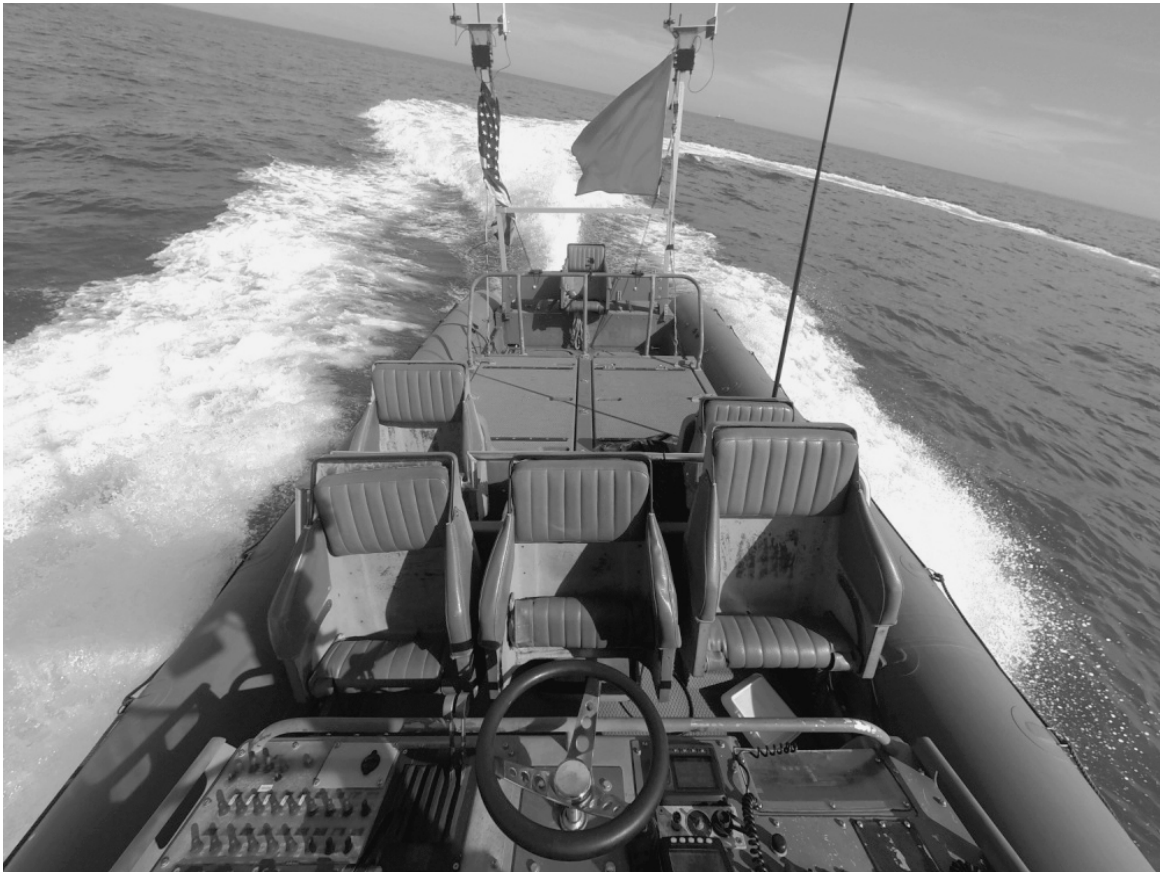
An uninhabited, autonomous boat near Virginia Beach as part of a U.S. Navy demonstration of swarming boats, 2016. Swarms are the next evolution in autonomous systems, allowing one human to control many uninhabited vehicles simultaneously, which autonomously cooperate to achieve a human-directed goal.
