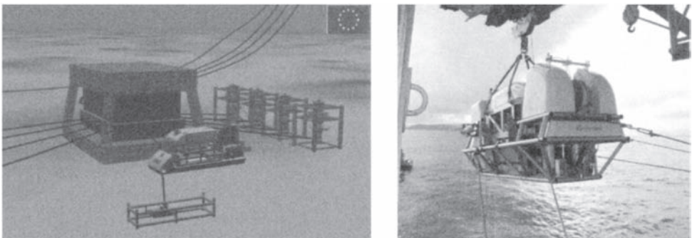
Figure 1.11 Left: Illustration of the SWIMMER concept—an autonomous deployment vehicle for Workclass ROVs. Right: The SWIMMER AUV and payload ROV being recovered after autonomous docking on seabed docking station.
