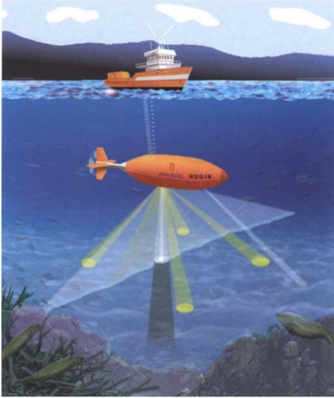
Color Plate 11 Illustration of HUGIN 3000 operating scenario in UUV mode. See Figure 11.2.
