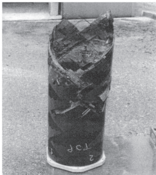
Figure 5.5 Collapsed carbon fibre pressure hull, the cross over of the fibre tows is seen in the lower section, the fracture follows the \pm 55^\circ wind angle.
