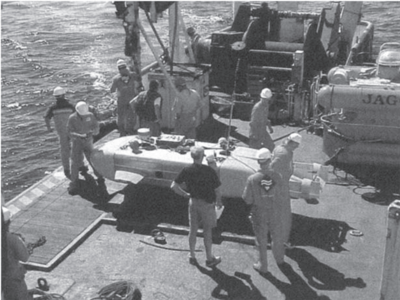
Figure 12.3 'MARTIN' during preparation for launch offshore Namibia 1999. The vehicle was equipped with a Tritech side scan sonar (Photo by courtesy of De Beers Marine Pty).
