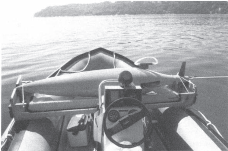
Figure 3.4 A Seaglider recovered aboard an inflatable boat after one month in Possession Sound. An un-pumped Sea Bird Electronics conductivity cell (with plastic tubing connected) is mounted above the wing. The antenna at the end of the trailing mast is not in view.
