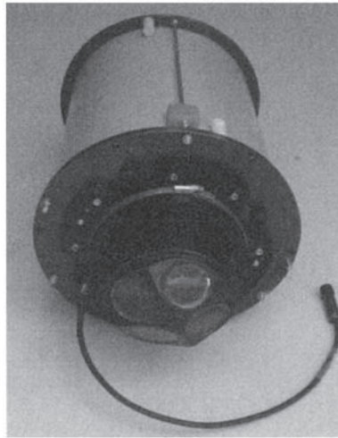
Figure 12.2 Doppler-inertial navigation instrument (MARPOS®) including the RDI DVL fixed to a pressure compartment housing the Kearfott optical gyro and the navigation computer. Diameter 37 cm, length 67 cm including the DVL.
