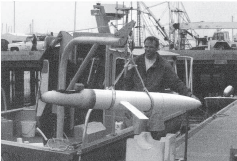
Figure 3.3 Spray being loaded onto a small boat in preparation for deployment. The aft flooded bay has been uncovered, exposing the hydraulic bladders. Above and forward of this a small protective covering obscures view of the Precision Measurement Engineering CTD.
