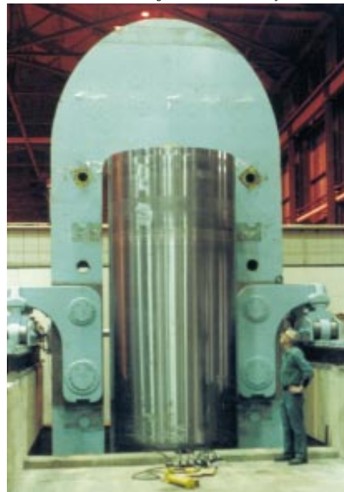
Figure 7-4: Side view of a large isostatic press.
