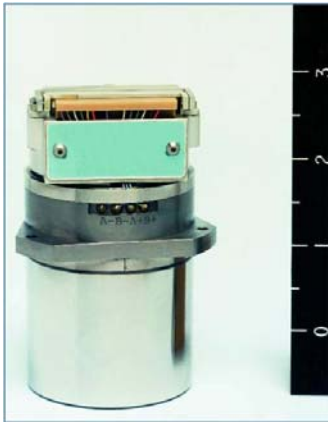
A pendulous integrating gyro
