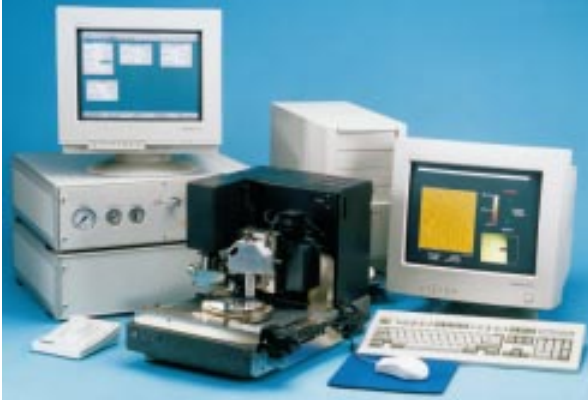
Figure 9-18: A profilometer system used for measuring mirrors.
