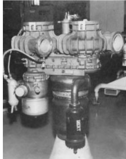
Figure 3-36: A multi-shaft turbopump assembly.
