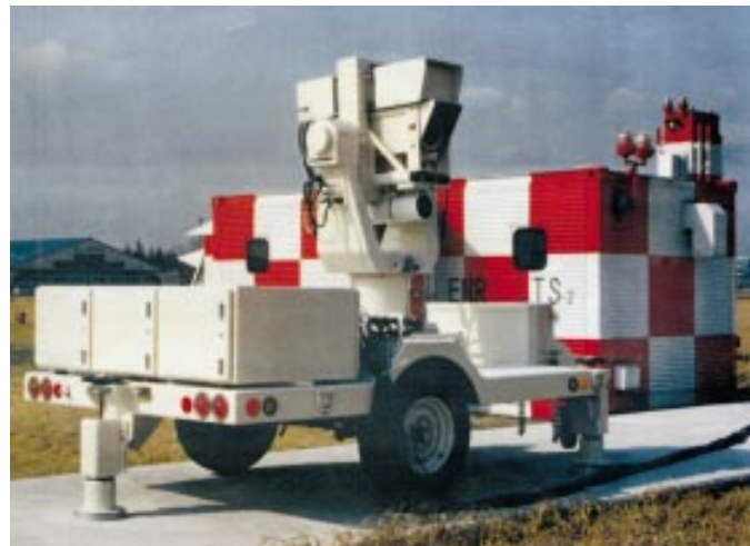
Figure 12-31: A mobile laser missile tracking system.
