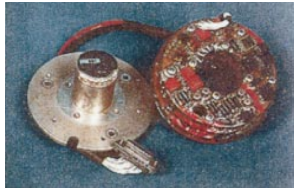
Figure 2-36: An RV SAFF system accelerometer with its associated electronics.
