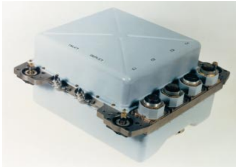
Figure 13-4: A radiation-hardened electronics assembly with liquid cooling.
