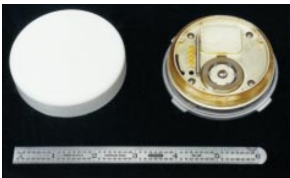
Figure 9-10: A fiber optic gyro with its top removed.
