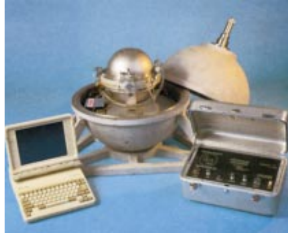
Figure 12-15: A non-MTCR-controlled gravity meter lowered by a ship or submarine.
