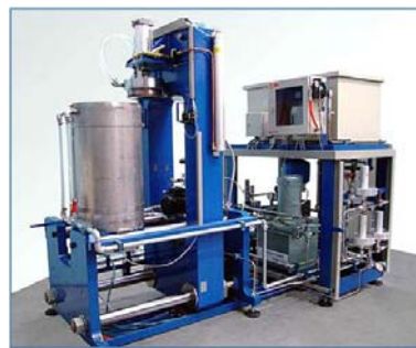
Left: A laboratory sized isostatic press. (ESPI) Right: A laboratory sized hot isostatic press. (Abra Fluid AG)
