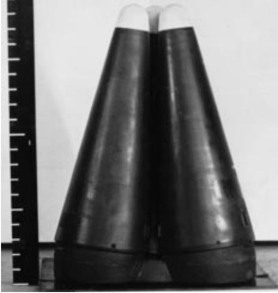
Figure 2-8: Three modern RVs attached to their mounting flange. The small fins at the aft end spin-stabilize the RV as it reenters the atmosphere.
