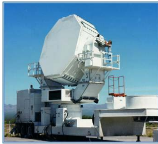
A mobile phased-array missile tracking radar. (MTCR Equipment, Software and Technology Annex
