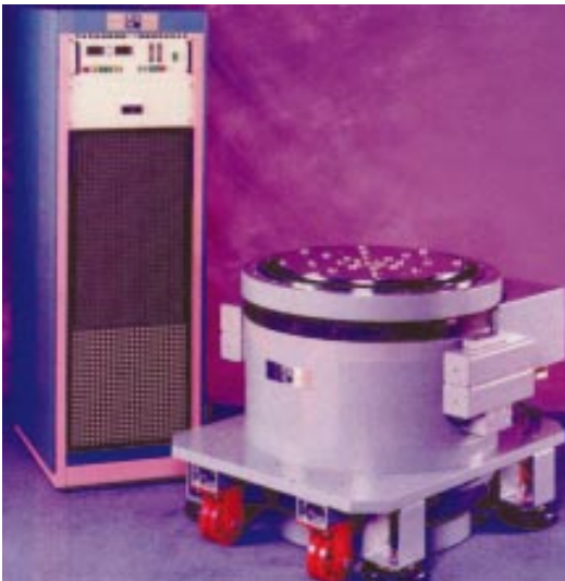
Figure 15-6: A power amplifier and its associated thruster.
