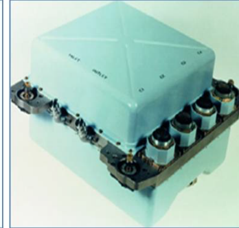
A radiation-hardened electronics assembly with liquid cooling. (The Charles Stark Draper Laboratory, Inc.)
