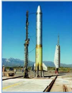
Minimal launch pad with a gantry and connections to a complete rocket system. (MTCR Equipment, Software)
