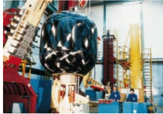
Figure 3-17: A large filament-wound solid rocket motor case.
