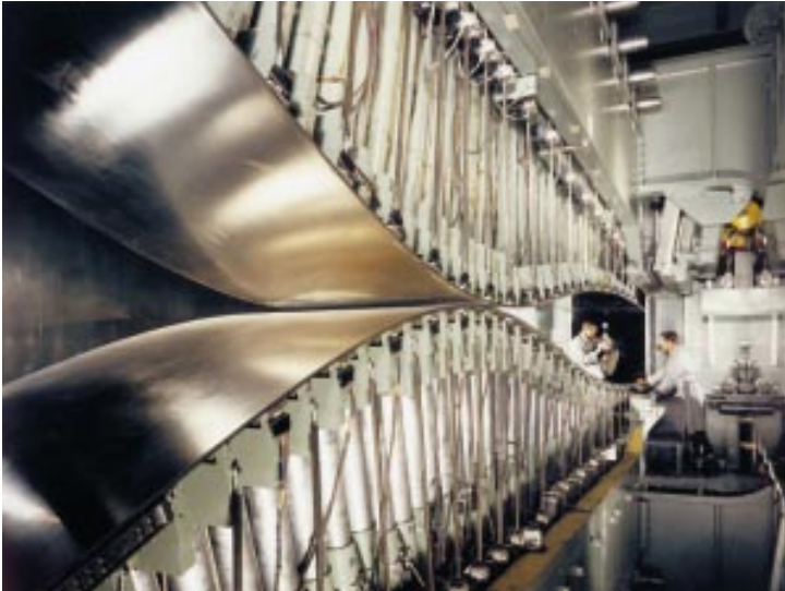
Figure 15-8: Exposed adjustable nozzle section of wind tunnel.
