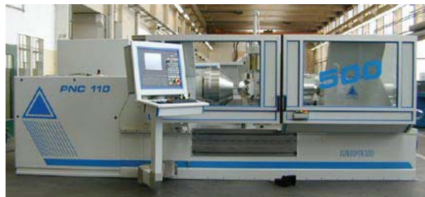
(ROK Doc: Item 44) Flow Forming Machine for Pressure Vessel Fabrication
