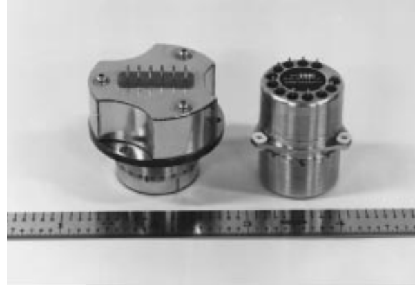
Figure 9-5: Two force rebalance accelerometers that can be built with any of a wide range of performance capabilities.
