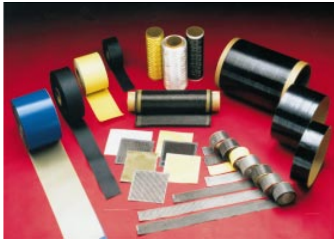
Figure 8-2: Examples of fabrics, tapes, and yarns.
