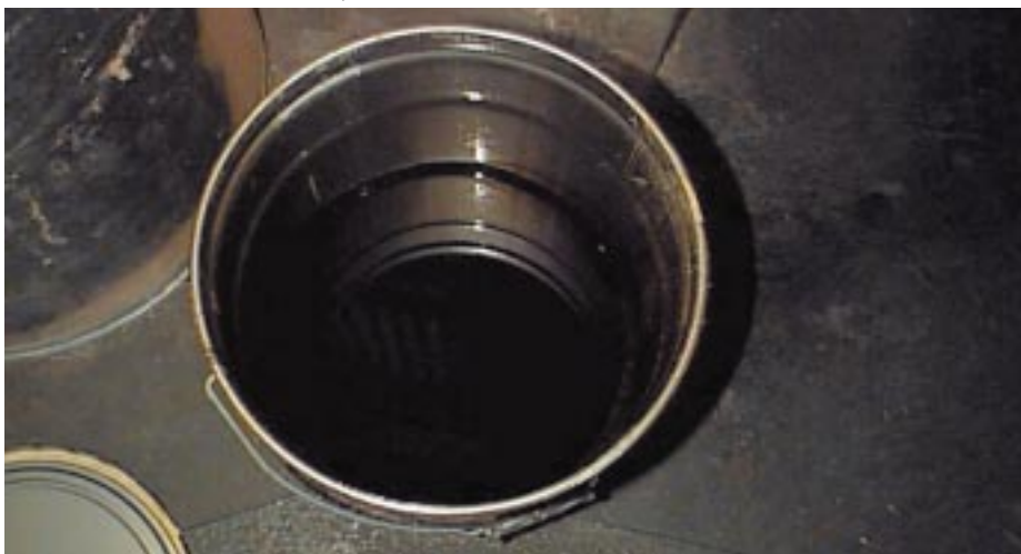
Figure 4-4: Top view of PBAN in a shipping drum.
