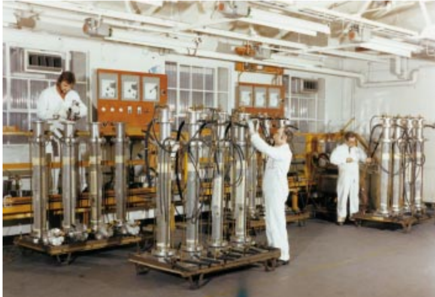
Figure 5-1: Tactical motors with cast-cure tooling attached.
