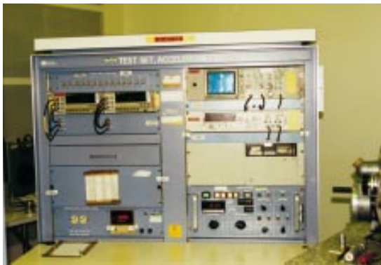
Figure 9-24: PIGA accelerometer alignment station control electronics.
