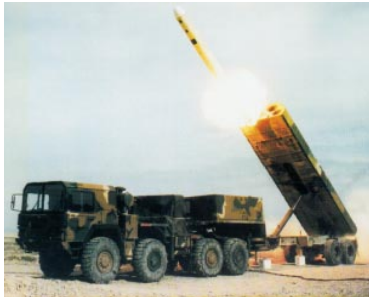
Figure 12-8: A transporter erector launcher used to transport and launch cruise missiles.
