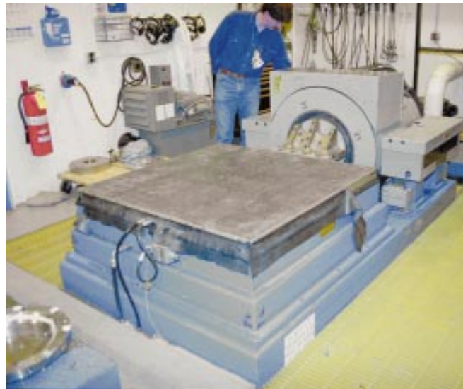
Figure 15-5: Thruster (in rear) connected to a slip table on common base.
