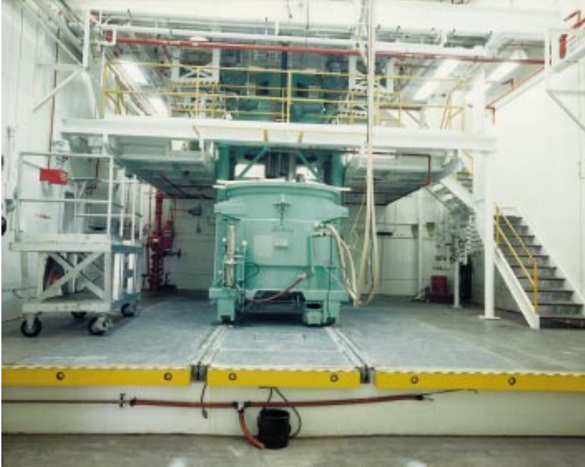
Figure 5-5: A 420-gallon propellant mixing bowl.
