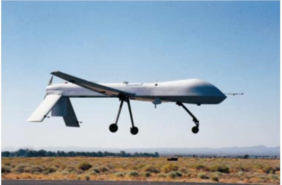
Figure 19-2: A typical unmanned air vehicle design normally used for reconnaissance missions.
