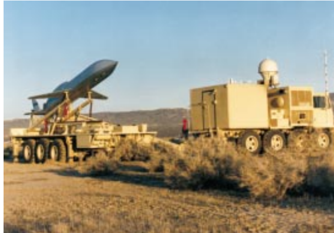
Figure 12-7: Rocket-assisted unmanned air vehicle erector launcher and its associated command-and-control van.
