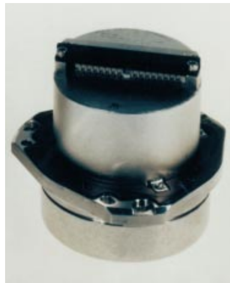
Figure 9-7: A DTG dynamically tuned spinning mass gyro.
