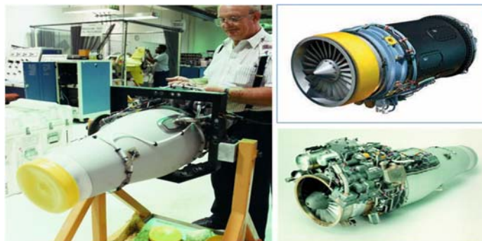
(May 2005) Figure 1: Left: A small turbofan engine for a cruise missile on its checkout stand. (MTCR Equipment, Software, and Technology Annex Handbook, Third Edition (May 2005) Top right: A turbofan used to power a HALE UAV. (Rolls Royce Group, plc) Bottom right: A small turbofan engine for a cruise missile. (Williams International)
