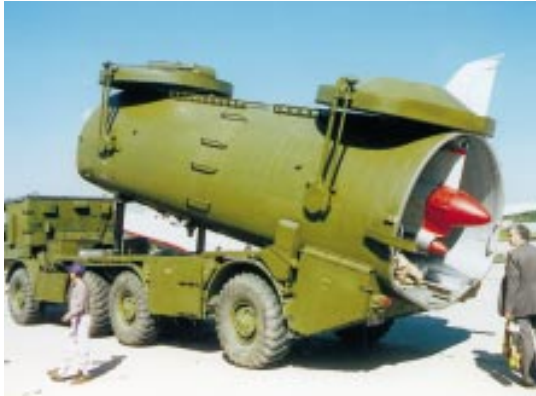
Figure 12-6: A transporter erector launcher for a large, Category II cruise missile.
