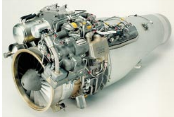
Figure 3-2: A small turbofan engine for a cruise missile.
