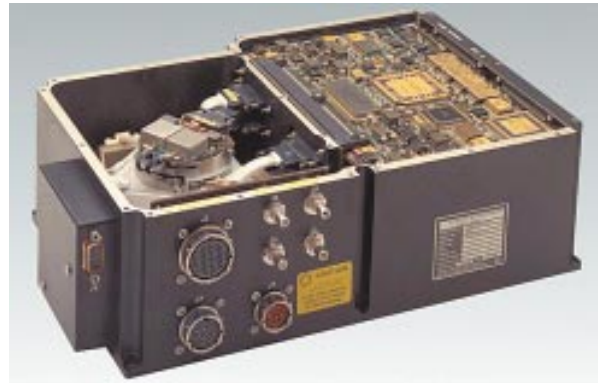
Figure 2-24: A guidance set using hemispheric resonating gyros.
