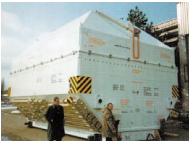
Figure 2-4: Shipping container for a liquid-fuel upper stage.
