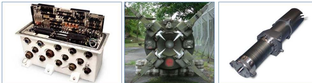
Figure 11: Left: A thrust vector control electronics box for use in large launch vehicle applications. (Moog, Inc.) Center: Four jet vanes mounted in the rear of a ballistic missile. (Russian military) Right: A fine positioning linear actuator designed for use in space applications. (Moog, Inc)
