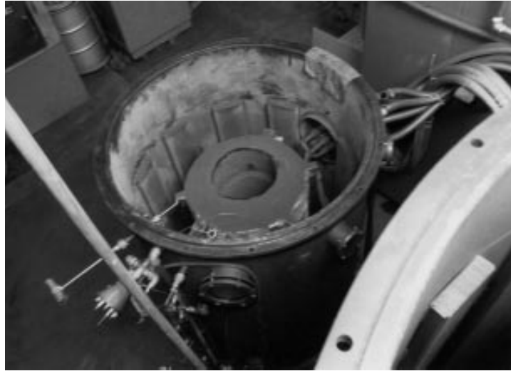
Figure 7-10: Inside of a small CVD furnace showing the retort, heaters, and insulation.
