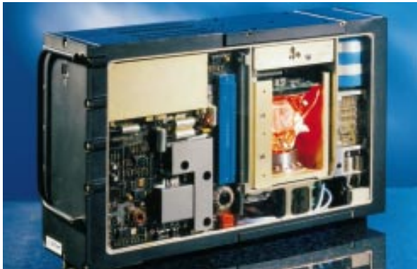
Figure 2-23: A guidance set using ring laser gyros.
