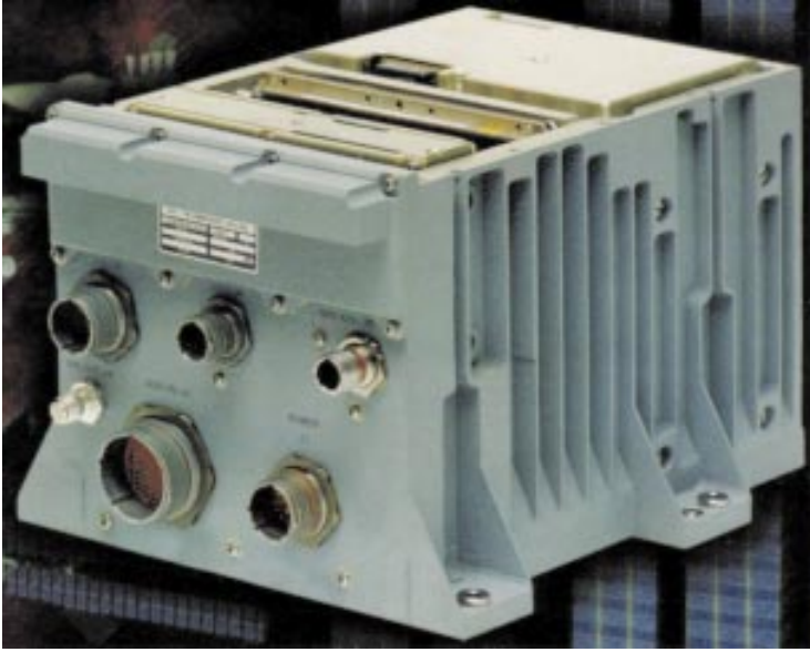
Figure 13-1: A global positioning system (GPS) aided inertial navigation system with integral guidance computer.
