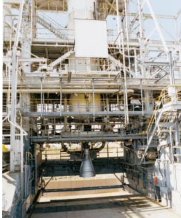
Figure 15-15: Close-up of the missile testing bay in Figure 15-14 showing the engine, feed lines, and run tanks.
