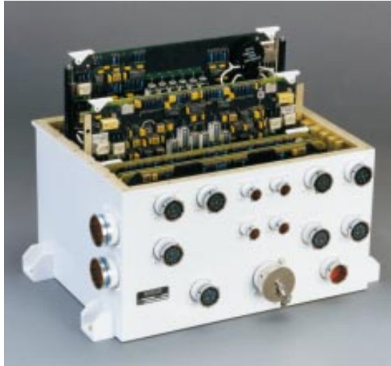
Figure 2-29: A thrust vector control electronics box for a large liquid rocket engine.
