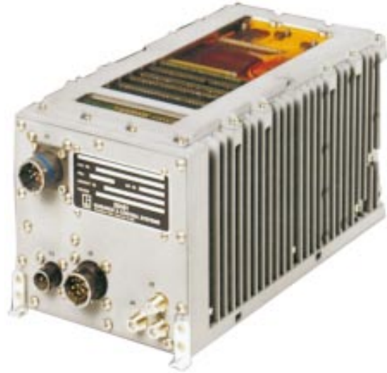
Figure 11-4: A complete guidance package based upon Global Positioning System receivers.
