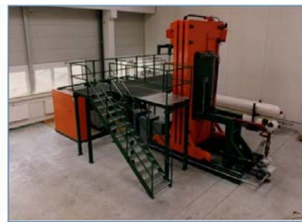
Left: A laboratory sized isostatic press. (ESPI) Right: A laboratory sized hot isostatic press. (Abra Fluid AG)
