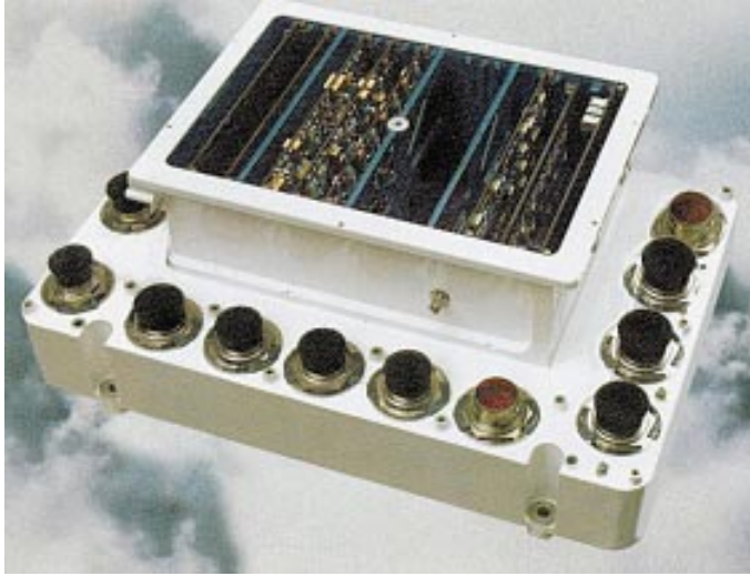
Figure 13-3: A radiation-hardened digital signal processor.
