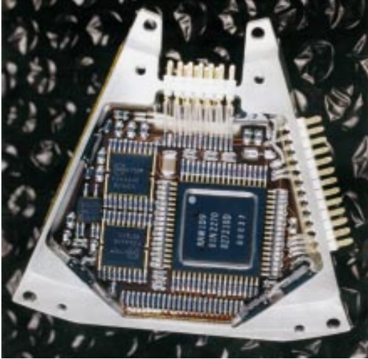
Figure 18-1: A circuit board populated with microcircuits hardened against nuclear effects.
