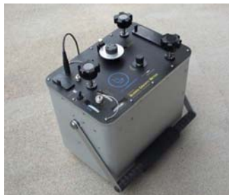
This automated gravity meter is one of the most precise, rugged and lightweight gravity meters. Under normal conditions, it can be leveled for mGal readings within 30 seconds, and has a drift rate of less than 0.5 mGals per month when mature. (ZLS Corporation)
