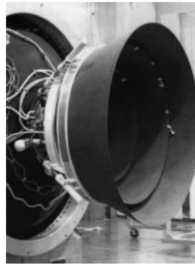
Figure 3-23: A modern extendable rocket nozzle skirt showing the actuators that increase its length after staging.
