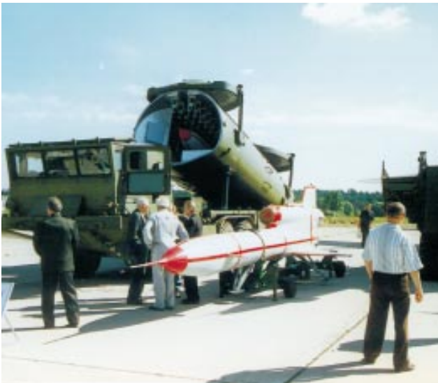
Figure 19-1: A jet-powered Category II unmanned air vehicle in front of its transporter erector launcher.
