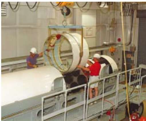
Figure 3-30: An interstage being positioned for attachment.
