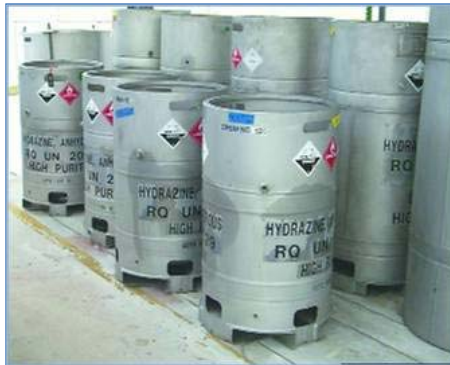
Figure 9: 34-gallon anhydrous hydrazine shipping containers made of 300-series stainless steel. (MTCR Equipment, Software and Technology Annex Handbook, Third Edition (May 2005))
