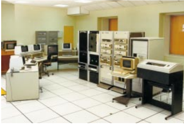
Figure 12-18: Representative ground-site telemetry receiving and processing equipment.
