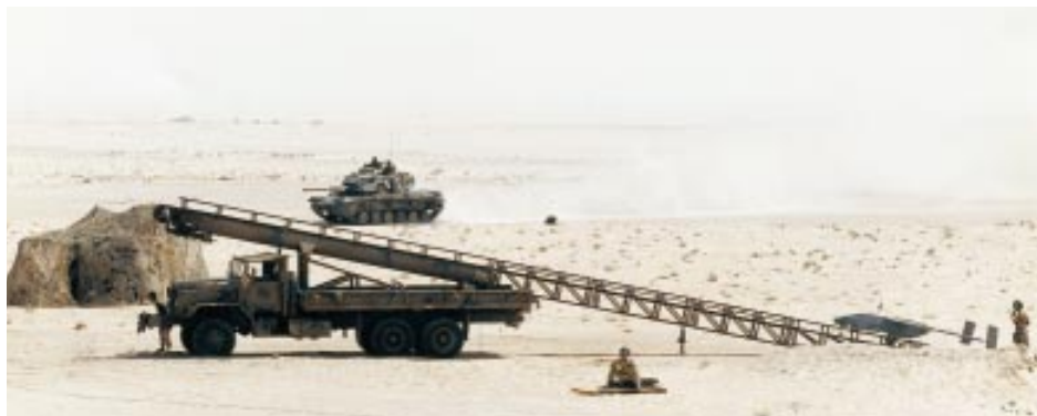
Figure 12-9: A pneumatic unmanned air vehicle launcher.
