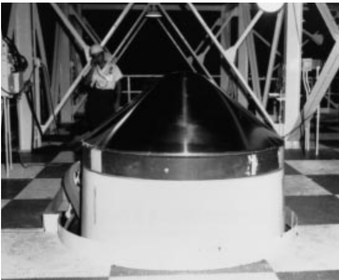
Figure 2-11: Another view of a beryllium-copper heat sink.
