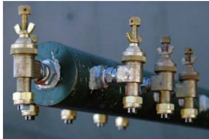
A Modular Aerial Spray System, used for pesticide application, can use a setting called ultra-low volume and specialized spray boom nozzles such as those shown here to spread one half to an ounce of chemical over an acre. (U.S. Air Force)
