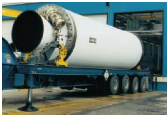
Figure 2-1: A completed stage for a solid propellant missile.
