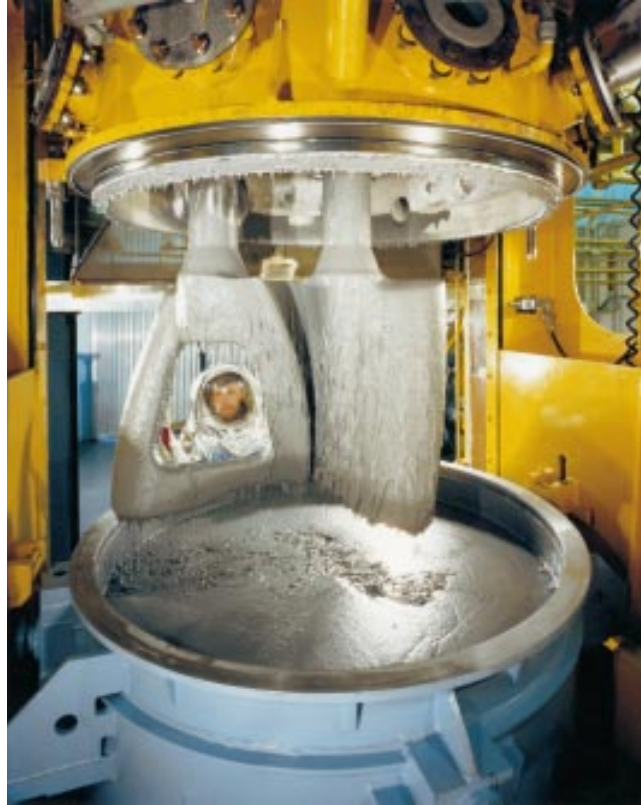
Figure 5-6: Open-blade configuration of a batch mixer.
