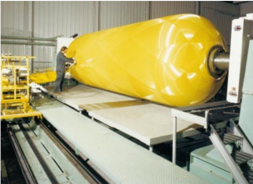
Figure 6-2: A large multi spindle filament winding machine.
