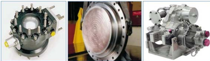
Left: A modern liquid propellant control valve. (Allied Signal Aerospace) Center: A liquid propellant injector plate. (Boeing) Right: A turbopump assembly for a space launch vehicle. (Hamilton Sundstrand)
