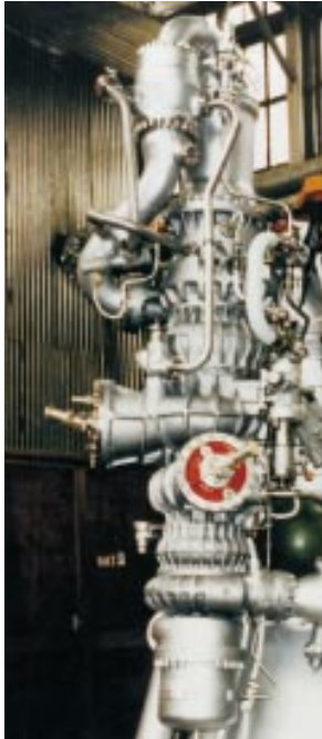
Figure 3-35: A single-shaft turbopump.
