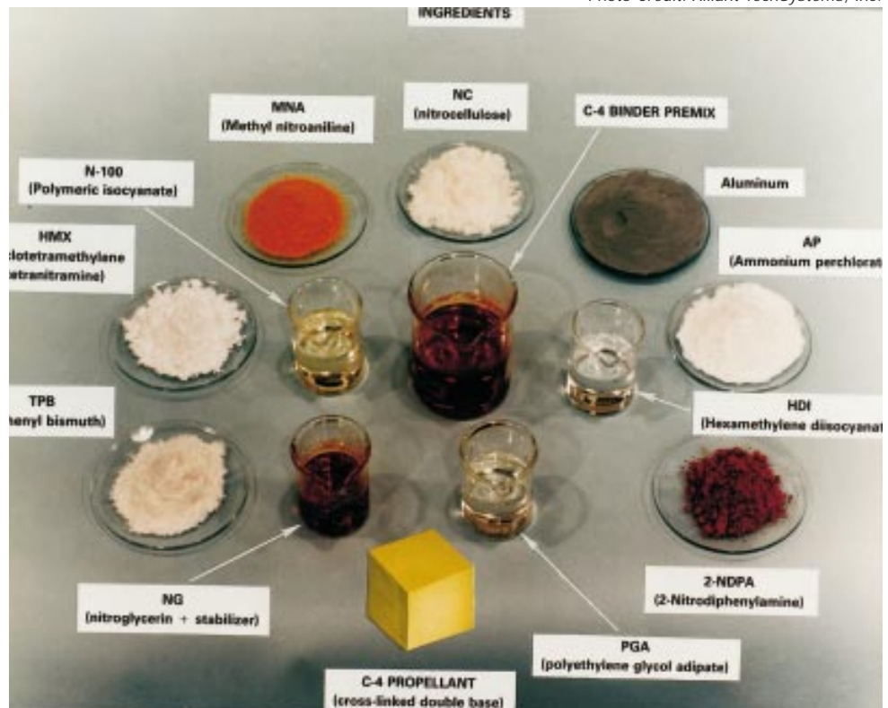
Figure 4-2: Composite-modified double-base propellant and samples of its constituent chemicals.
