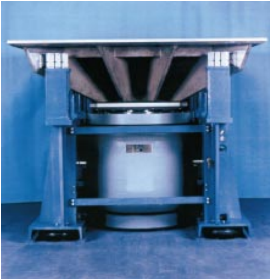
Figure 15-4: A thruster with an expanded head.
