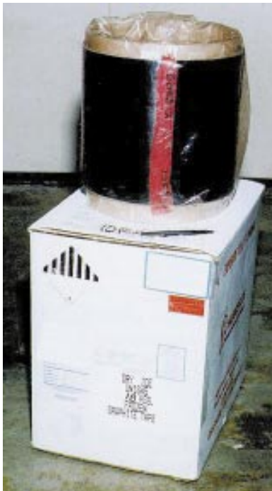
Figure 8-4: Special cardboard container for holding dry ice packing around a carbon fiber prepreg tape spool during shipping. The dry ice is normally contained in a plastic bag packed around the spool.
