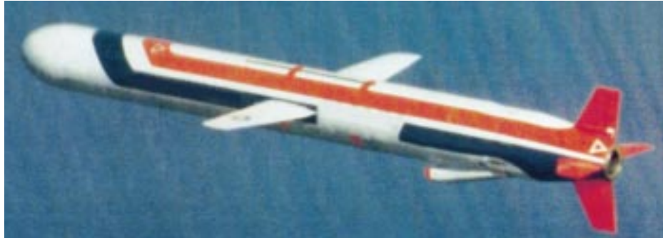
Figure 1-8: A land attack cruise missile in flight showing its entire control surfaces and engine inlet.
