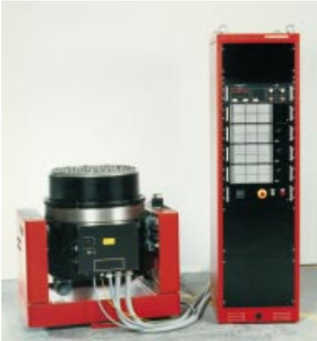
Figure 15-21: A thruster table and its power supply.
