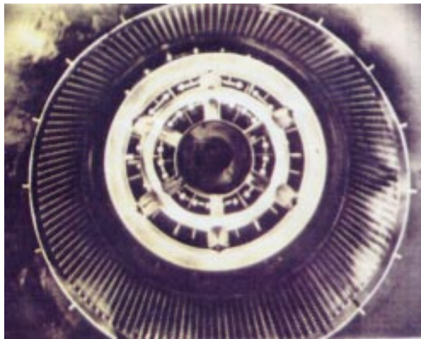
Figure 3-15: A baffle-type flameholder installed in a ramjet engine.
