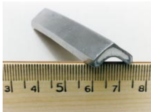
Figure 3-28: Short section of flexible linear-shaped charge (on a centimeter scale) designed to cut through a missile stage.
