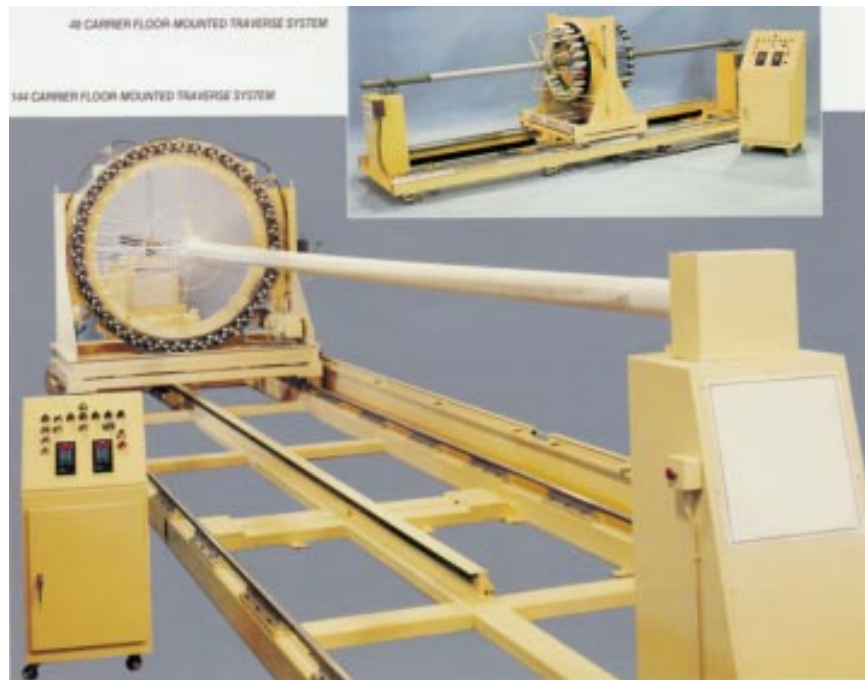
Figure 6-7: A 144 carrier floor-mounted traverse braiding machine.
