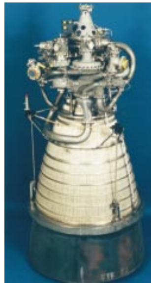
Figure 3-24: An engine with a large, regeneratively cooled nozzle.
