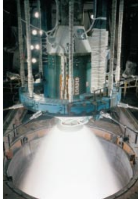
Figure 15-17: A solid rocket motor being tested at simulated altitude.
