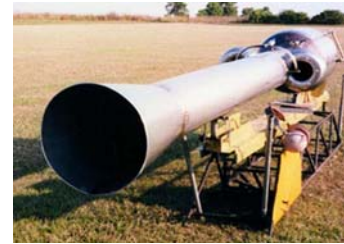
A modern pulsejet engine with a rearward facing intake. (Thermojet)
