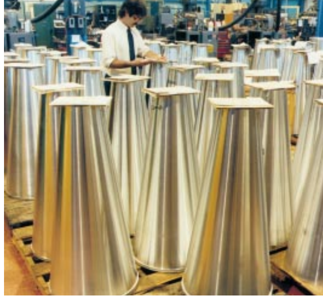
Figure 2-9: Modern RV mid-sections during manufacture.
