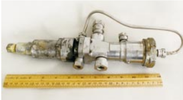
Figure 3-31: A servo valve from a Scud missile.
