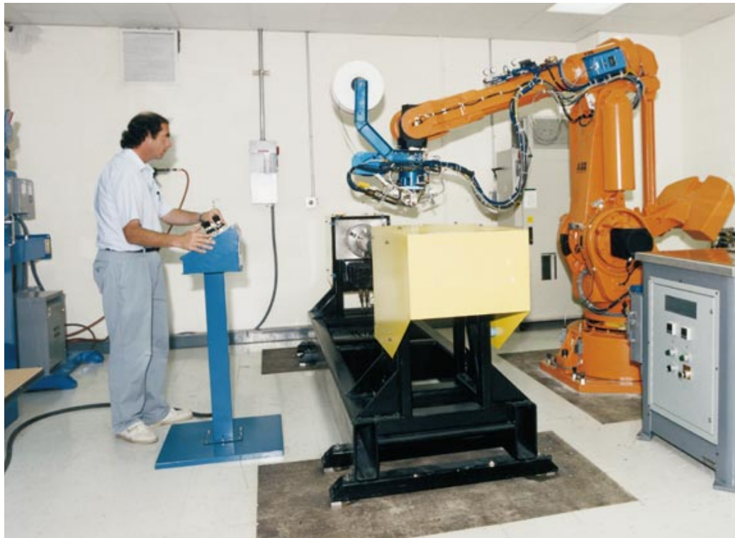
Figure 6-5: A modern, multi-axis numerically controlled tape laying machine.
