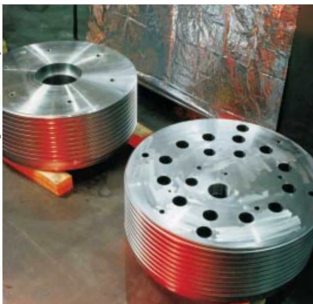
Figure 7-2: Two removable high-pressure closures, showing holes for hoses or pipes.
