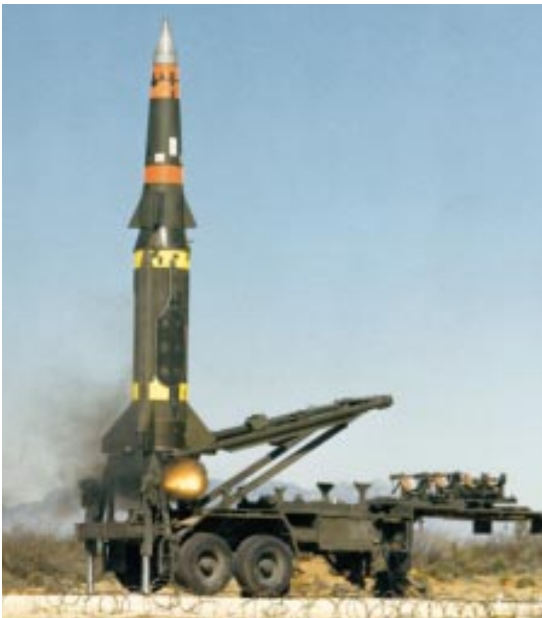
Figure 12-4: An erector launcher detached from its prime mover.
