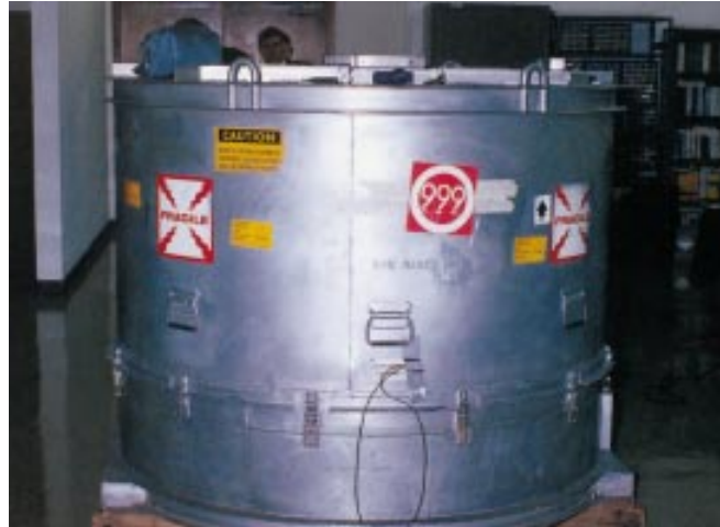
Figure 2-27: A shipping container for an ICBM guidance system.
