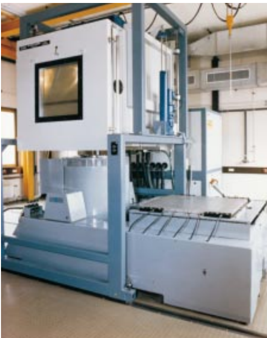
Figure 15-23: Another vibration and environmental test apparatus configuration.
