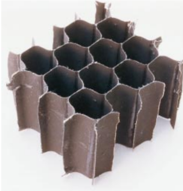
Figure 17-4: A sample of radar absorbing honeycomb material.
