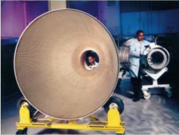
Figure 3-26: End views of regeneratively cooled nozzles.
