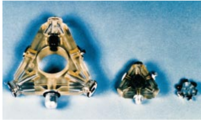
Figure 9-9: Three exposed ring laser gyros without their associated electronics.
