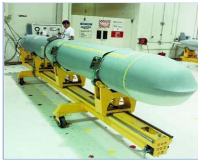
Figure 7: An operational cruise missile on its checkout stand, showing its nose cone modified to lower radar returns and enhance aerodynamic performance. (MTCR Equipment, Software and Technology Handbook, Third edition (May 2005))
