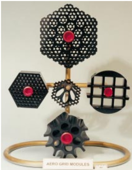
Figure 3-11: Various aerodynamic grids used to straighten the flow of air into a ramjet engine.
