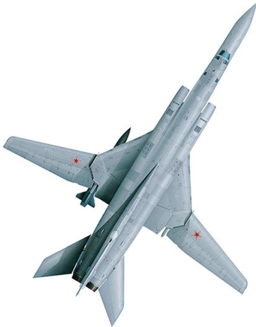
**The Tu-22M is not fitted with ailerons. Instead, control is provided using three sections of spoilers/lift dumpers on the outer wing panels and differential deflection of the elevators.**
