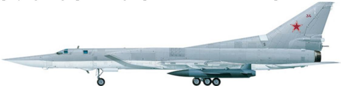
**A Tu-22M-3 armed with a Kh-22 missile underwing. This delta-wing missile is made of welded titanium and steel alloys, and powered by a twin-chamber liquid-fuel rocket motor.**
