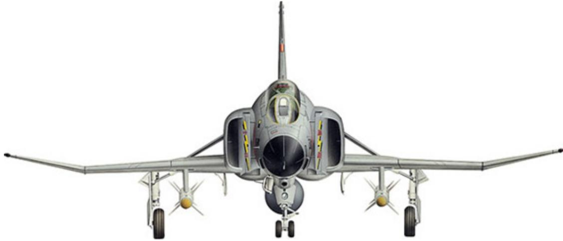
For anti-shipping work, the F-4EJ Kai can be equipped with the ASM-2 missile, seen here underwing. This turbojet-powered weapon uses infra-red guidance for terminal accuracy.
