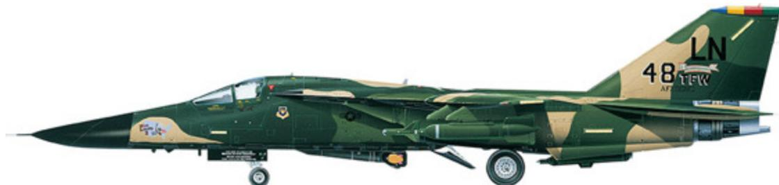
**F-111Fs of the 48th TFW were employed almost exclusively to drop laser-guided bombs during Desert Storm, in this case 907kg (2000lb) GBU-24 Paveway IIIs with penetrator warheads.**
