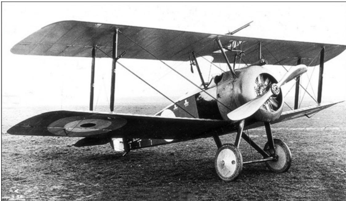
**The navalized 2F.1 variant differed from the basic Camel in its armament of a single Vickers gun in the port position, supplemented by a Lewis gun above the wing centre section.**
