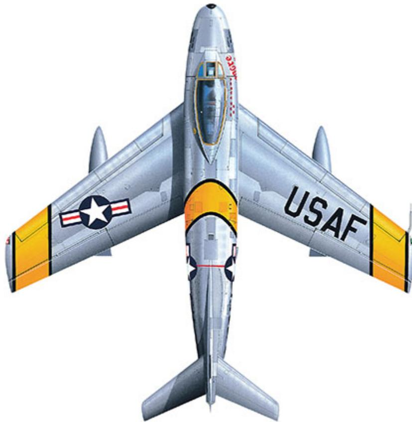
Last of the fighter line from North American production was a dedicated fighter-bomber, the F-86H, with a more powerful J73 engine contained within a much-redesigned fuselage, additional fuel capacity and nuclear-weapons capability. A total of 477 were built.
