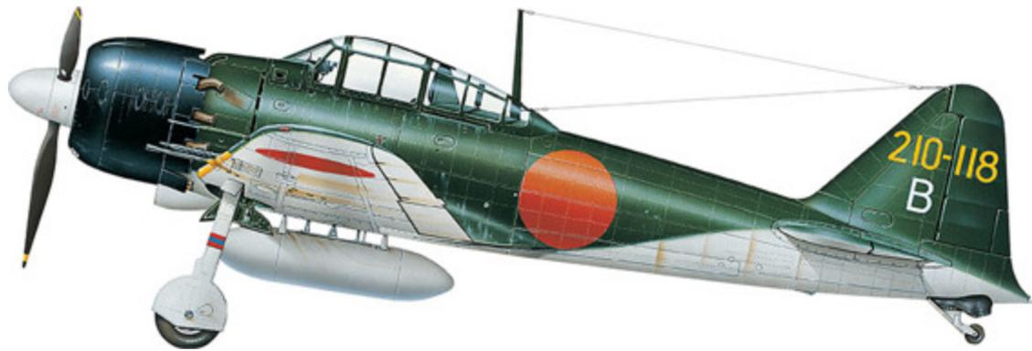
**The A6M5c sub-variant (93 built) featured improved armament in the form of an additional pair of 13.2mm (0.52in) machine guns fitted outboard of the standard wing cannon.**
