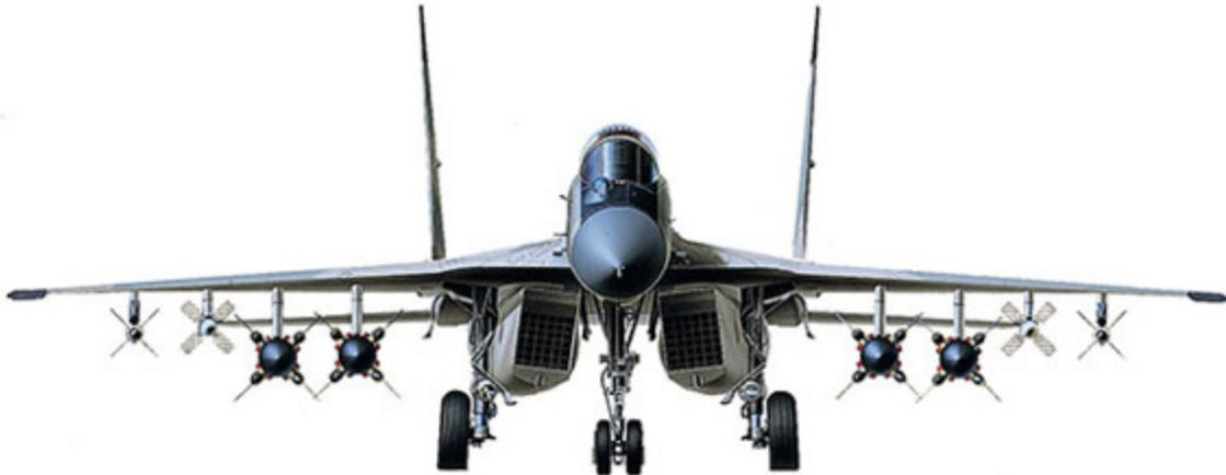
**The original MiG-29M launched efforts to create a genuine second-generation 'Fulcrum', including flyby-wire flight controls, advanced structure, improved powerplant, avionics and weapons systems. The 9.15 yielded five prototypes.**
