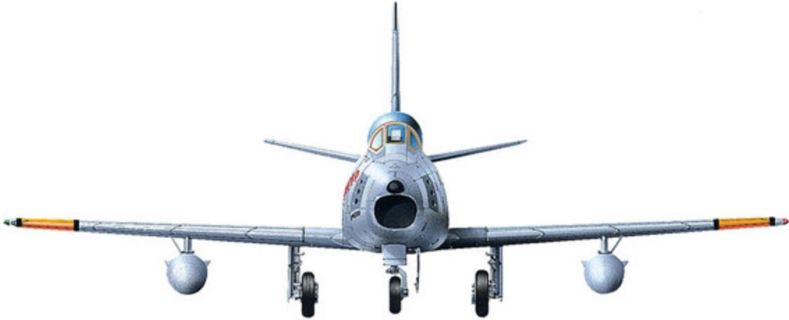
**In the neat undercarriage of the Sabre, the nosewheel unit retracted backwards to lie in the forward fuselage, while the mainwheels retracted inwards to lie in the fuselage.**
