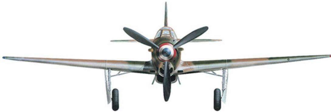
**A frontal view of the Yak-9D. The fighter utilized a lightweight armament comprising a single 20mm (0.79in) ShVAK firing through the spinner and one 12.7mm (0.5in) UBS machine gun.**
