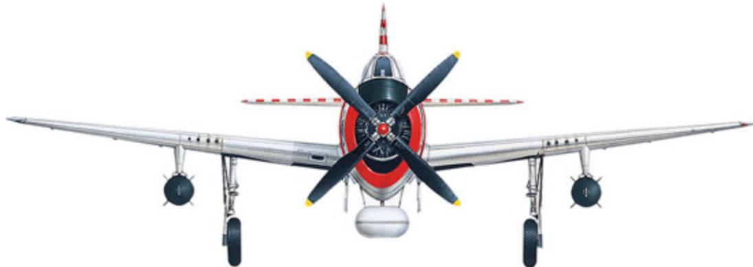
**A frontal view of the 527th FS P-47D reveals the external stores, comprising 1000lb (454kg) bombs underwing and one of the nine different types of drop tank, carried on the centreline.**
