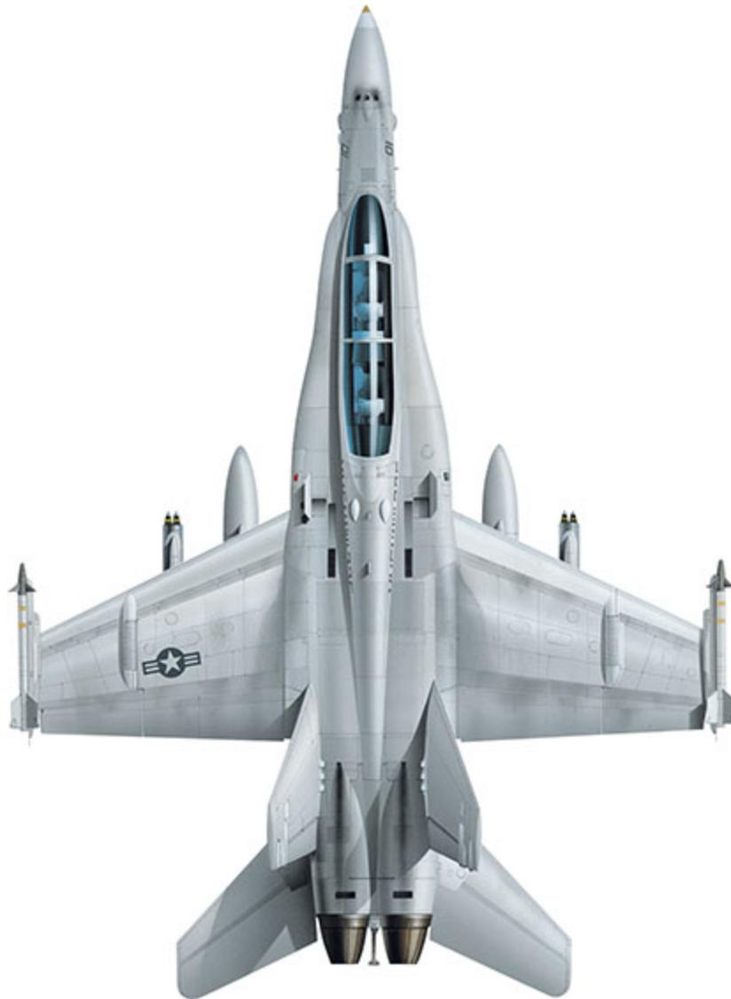
A two-seat version of the Hornet was developed alongside the F/A-18A, and produced the F/A-18B, which, apart from the addition of a second crew position, was basically unchanged from the A-model. A total of 40 aircraft were completed for the U.S. Navy and Marine Corps.
