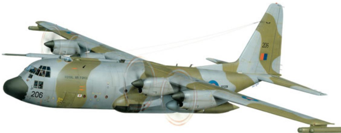
**The C-130K version was built specifically for British use on the basis of the C-130H, and entered RAF service as the Hercules C.Mk 1, seen here on strength with the Hercules Wing at RAF Lyneham in 1990. This is a C.Mk 1P sub-variant with an inflight refuelling probe above the cockpit.**
