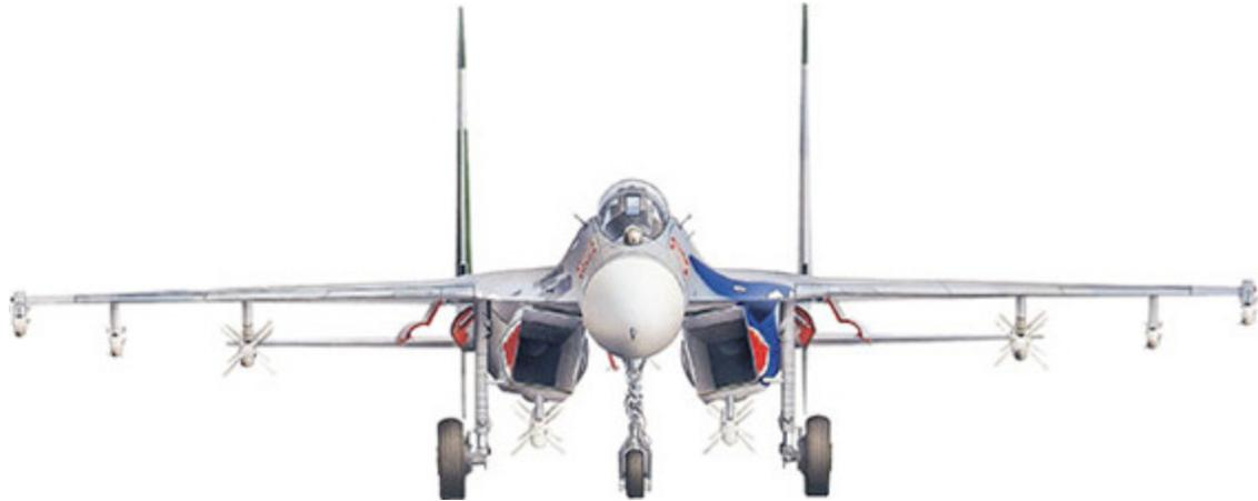
**The original 'Flanker-B/C' production models can carry weapons on a total of 10 external hardpoints: one on each wingtip, two under each wing, one under each engine nacelle and two in tandem on the fuselage centreline.**
