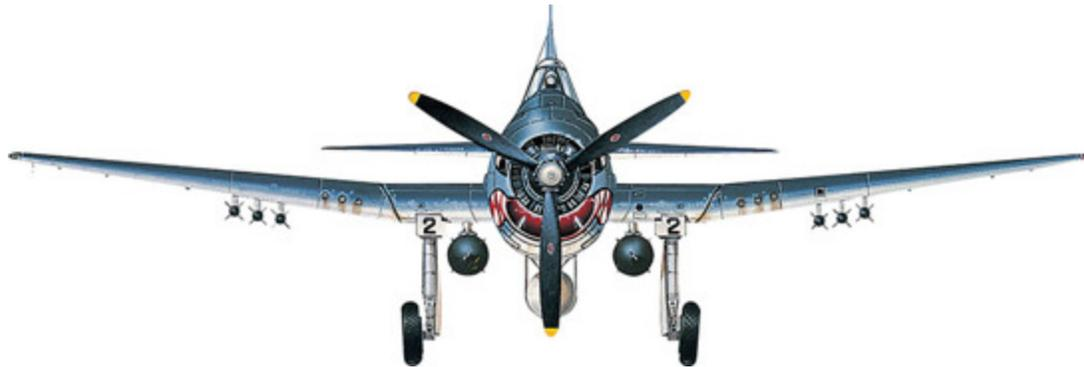
**A frontal view of the fully armed VF-27 F6F-5 reveals details of its weaponry, including machine guns in the wing, bombs on the inner underwing stations and rocket projectiles outboard.**
