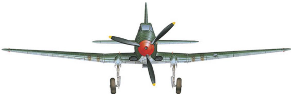
**A frontal view of the Il-10. Powered by a Mikulin AM-42 driving a three-bladed propeller, the Il-10 demonstrated greatly enhanced performance compared to the Il-2.**
