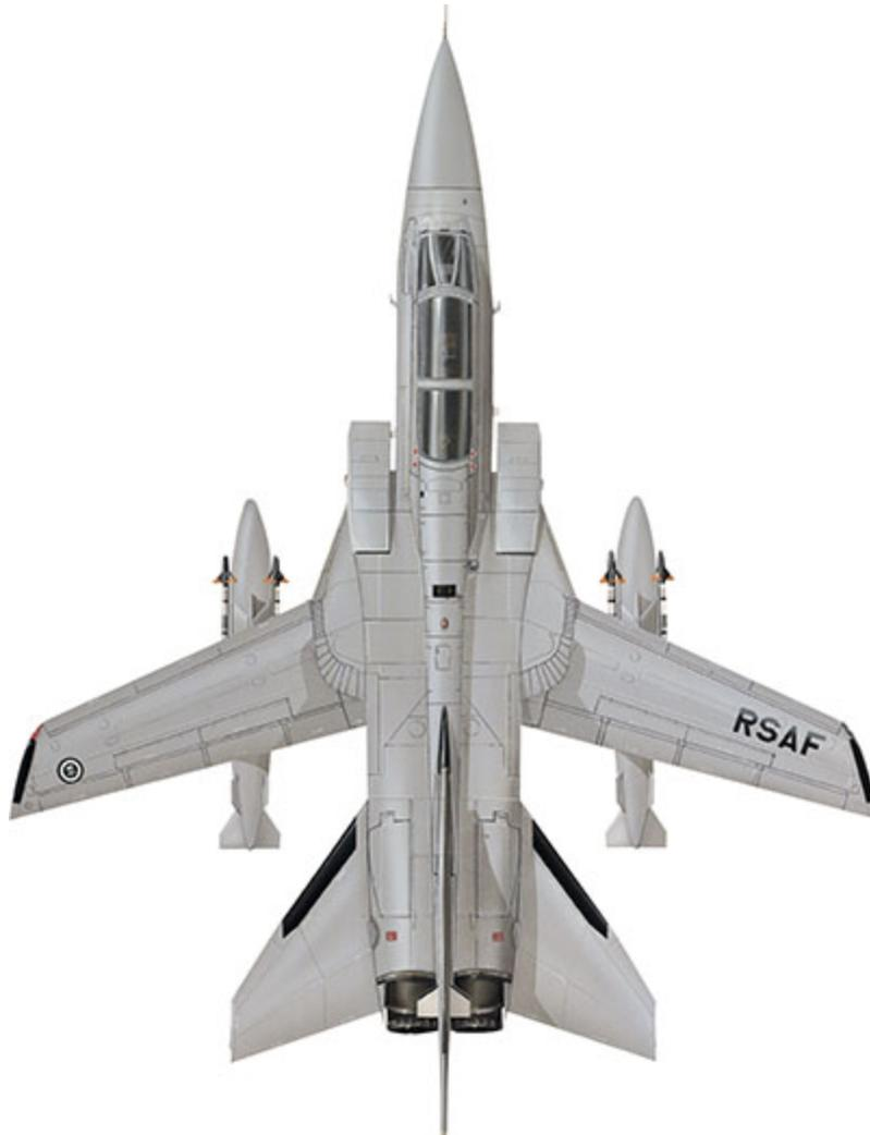
**The RSAF's Tornado ADVs were equivalent to the RAF's F.Mk 3, and were delivered with the Sky Flash semi-active radar-homing AAM. The Saudi Tornado ADVs were retired in 2007.**
