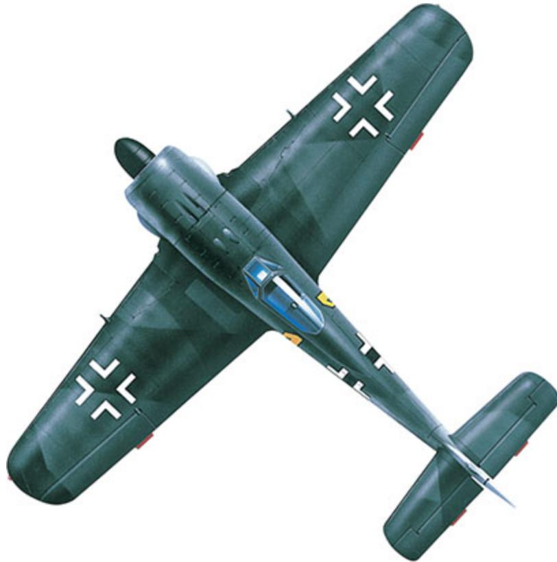
**A plan view of Schneider's Fw 190A-1 demonstrates the excellent view provided by the one-piece, rear-sliding canopy. Powerplant for the A-1 was the 1193kW (1600hp) BMW 801C-1.**
