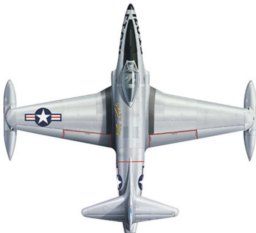
After 240 F-80Bs had been completed, production switched to the F-80C that was the definitive Shooting Star model. The F-80C had a further increase in power, and improved armament, and a total of 670 were completed by the end of 1950. The initial powerplant for the C-model was an Allison J33-A-23 rated at 20.46kN (4600lb) thrust, but this gave way in later production machines to a J33-A-35 developing 24.01kN (5400lb) of thrust. Provision was also added for underwing rockets.
