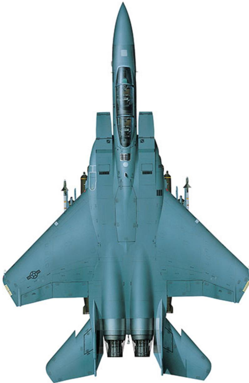
**The F-15E carries conformal fuel tanks on the sides of the fuselage. Each holds 2737 litres (723 U.S. gal) of fuel, and is fitted with three stub pylons for attaching weapons.**
