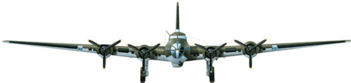
**A frontal view of a B-17C, 39 examples of which were ordered in 1939. These aircraft were heavier than their predecessors, on account of increased armour, heavier defensive armament and additional equipment. However, 895kW (1200hp) engines ensured this was the fastest Flying Fortress version.**
