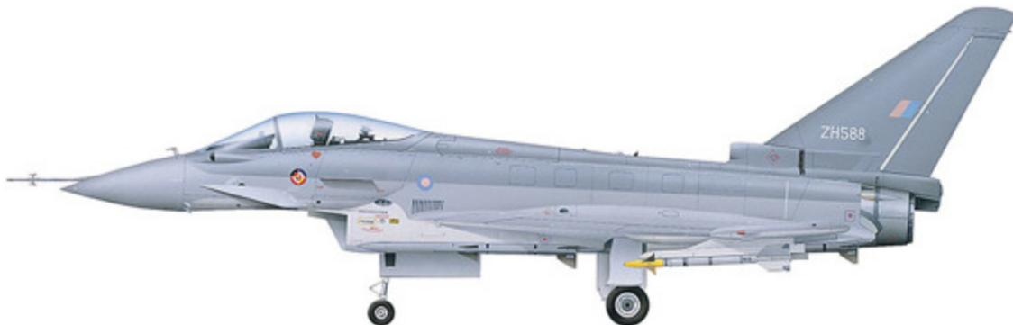
**DA.2, serial ZH588, was the first British prototype, and is seen armed with AIM-9L Sidewinder missiles. The aircraft was first flown at Warton in April 1994 and is now at the RAF Museum.**
