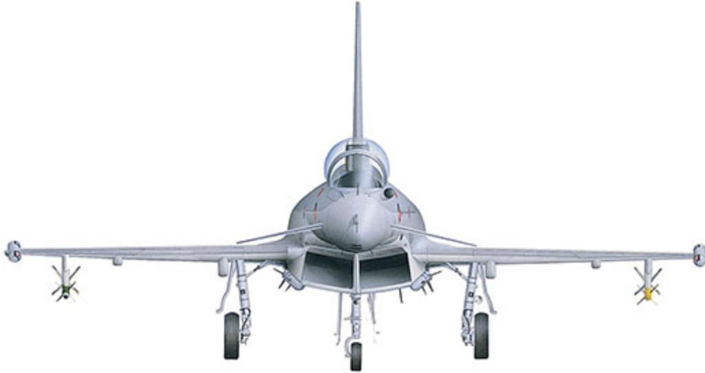
**The twin ‘chin’ engine intakes have a hinged lower lip (‘varicowl’) to ensure good performance at all speeds and angles of attack. An ogival splitter plate removes boundary layer airflow and feeds the engines with clean, fast-moving air.**
