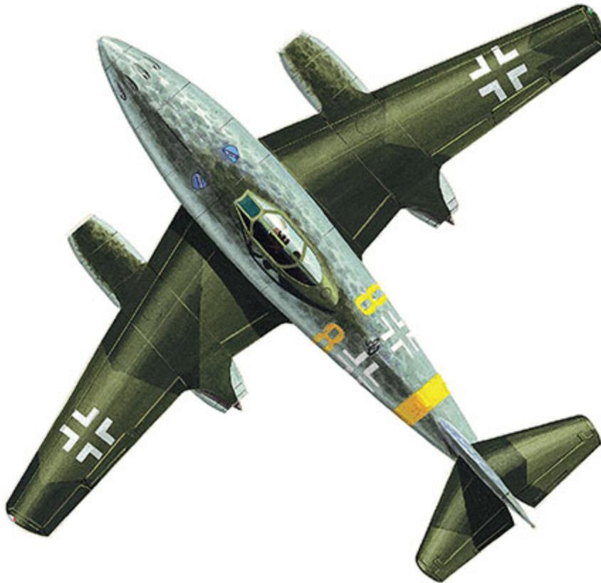
The Me 262A-2a was equipped to carry up to 500kg (1102lb) of bombs in addition to the basic four-cannon armament and was also developed as a two-seater, the Me 262A-2a/U, with a bomb-aimer in a glazed nose.
