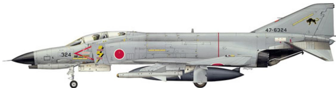
**Three views of an upgraded F-4EJ Kai of the Japan Air Self-Defense Force's 8 Hikotai based at Misawa. The unit had a dual-role ground attack and anti-shipping assignment.**
