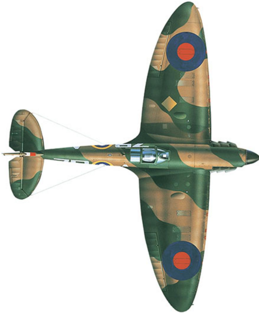
**An aerial view of this Battle of Britain Spitfire Mk IA reveals the classic tapered wing of the type, as well as the yellow gas detection patch applied on the port wing in summer 1940.**
