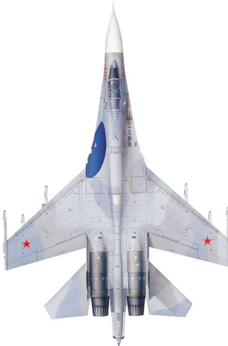
**The Su-27 features a prominent leading edge root extension (LERX) that provides additional lift, helping destabilize the heavy radar nose. The starboard wing root contains a 30mm (1.18in) cannon.**
