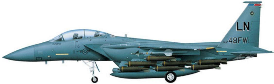
**An F-15E as flown by the commander of the 48th Fighter Wing at RAF Lakenheath. The aircraft is armed for a close support mission, with 14 SUU-30H/B cluster bombs, plus AIM-9s.**
