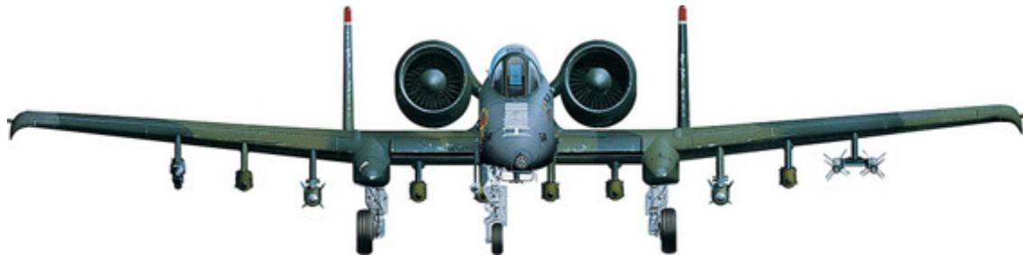
**This A-10A carries a typical Desert Storm mixed weapons load of Mk 20 Rockeye cluster bombs, AGM-65D Mavericks, twin Sidewinders and AN/ALQ-119 electronic countermeasures pod.**
