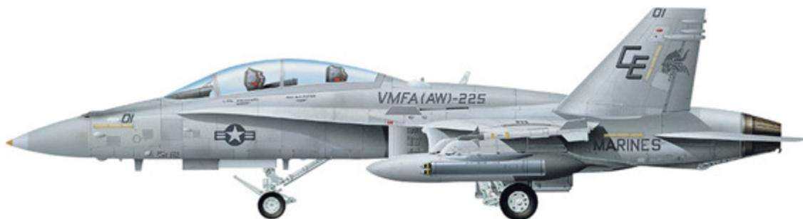
**An F/A-18D of the U.S. Marine Corps’ VMFA(AW)-225 armed with 127mm (5in) Zuni unguided rockets underwing, used for target-marking purposes in the forward air controller (airborne) role.**
