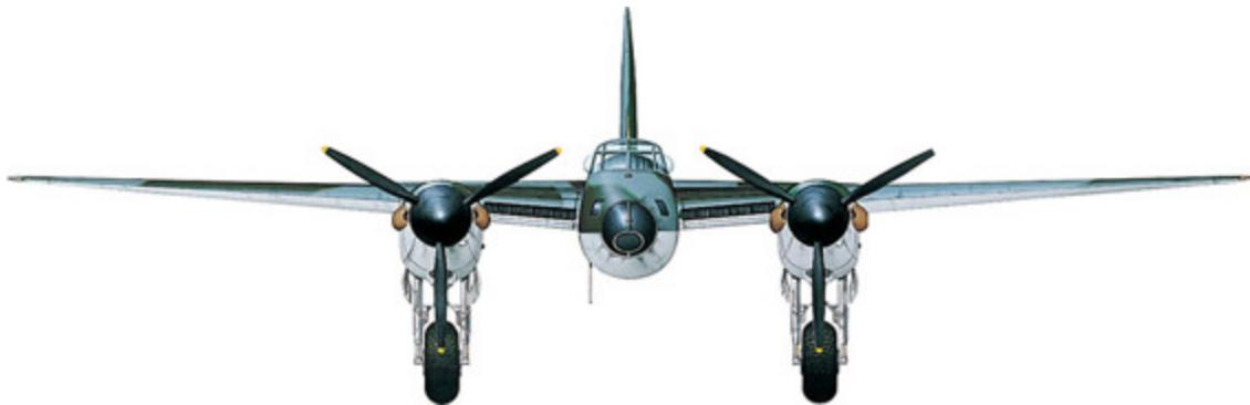
**Frontal view of a Mosquito B.Mk IV Series II light bomber, which introduced various refinements including extended nacelles, enlarged tailplane and flame dampeners on the exhausts.**
