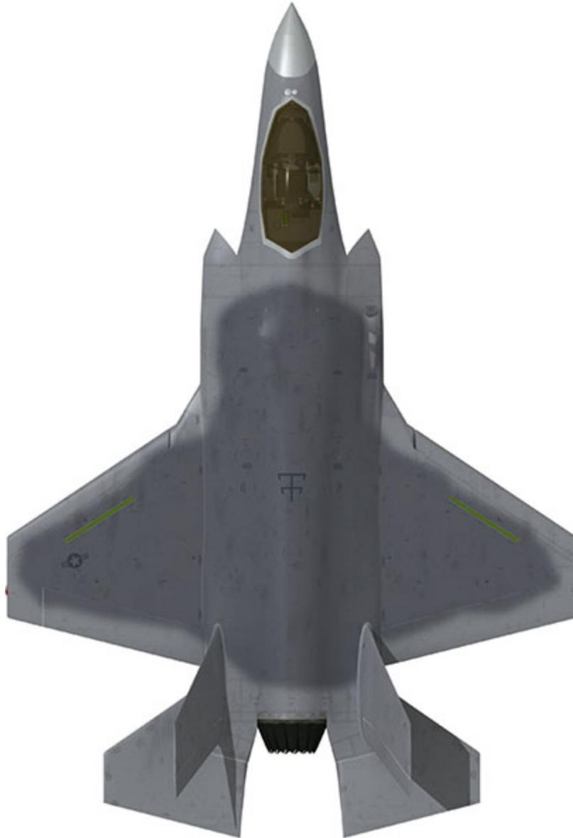
The F-35B, which is replacing the AV-8B and F/A-18 with the USMC, is capable of STOVL operation thanks to its shaft-driven Rolls-Royce LiftFan propulsion system and an engine that can swivel 90 degrees when in short take-off/vertical landing mode. The F-35B has a smaller internal
