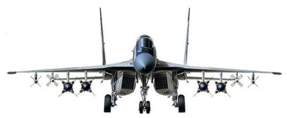
The original MiG-29M launched efforts to create a genuine second-generation 'Fulcrum', including flyby-wire flight controls, advanced structure, improved powerplant, avionics and weapons systems. The 9.15 yielded five prototypes.
