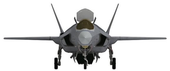
Compared to the Harrier, STOVL operations in the F-35B are much simplified for the pilot. Converting from conventional flight to STOVL mode is no more complicated than pushing a button. The F-35A is the only version to carry an internal cannon – the 25mm (0.98in) GAU-22/A – and will be the most prolific model, replacing the A-10 and F-16 with the USAF and serving with the majority of allied air forces to fly the Lightning II.
