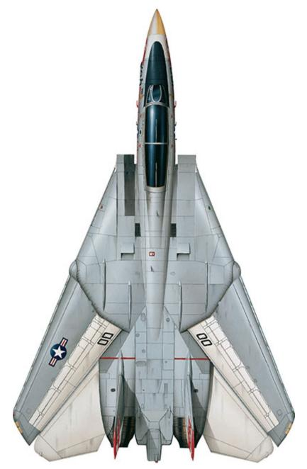
The Tomcat's variable-geometry outer wings are equipped with full-span leading edge slats and almost full-span trailing edge flaps. Front-section spoilers provide roll control.
