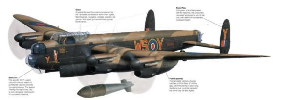
A Lancaster B.Mk I (Special) of No.9 Squadron, based at RAF Bardney in 1945. The aircraft is seen here dropping a Tallboy weapon, as used to attack the U-boat pens at Bergen, Norway.
