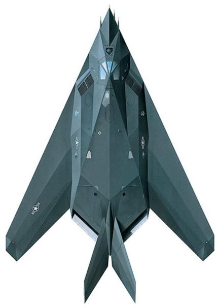
A straight line running from nose to wingtip (swept at 67.5 degrees) and similar sweepback on the tailfins served to dissipate radar energy away from its source.
