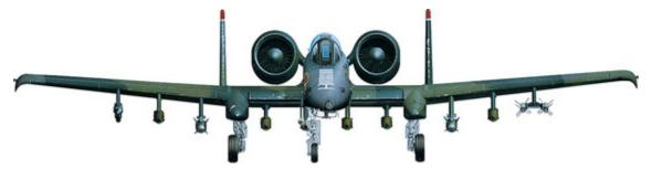
This A-10A carries a typical Desert Storm mixed weapons load of Mk 20 Rockeye cluster bombs, AGM-65D Mavericks, twin Sidewinders and AN/ALQ-119 electronic countermeasures pod.
