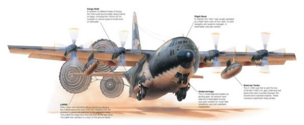
A USAF C-130E operating in Vietnam in 1966. The aircraft is conducting a low-altitude parachute extraction cargo drop, as employed in the defence of Khe Sanh in 1968, when C-130s accounted for 90 per cent of supplies used by troops defending the base from a North Vietnamese siege.
