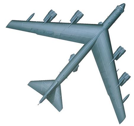
Built in five sections, the huge wing of the B-52 uses the entire interspar area for fuel carriage. The wing is highly flexible to absorb different loads depending on weights and aerodynamics.
