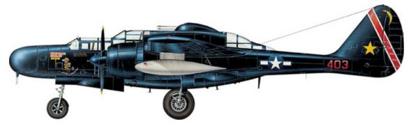
Two views of P-61B serial 42-39403 was fitted with the dorsal gun barbette. Other features of the B-model included a longer nose, Curtiss Electric propellers and four external pylons.
