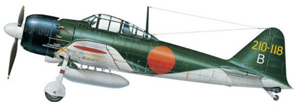
The A6M5c sub-variant (93 built) featured improved armament in the form of an additional pair of 13.2mm (0.52in) machine guns fitted outboard of the standard wing cannon.
