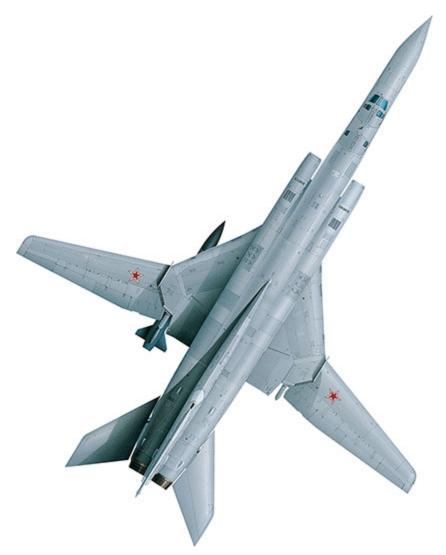
The Tu-22M is not fitted with ailerons. Instead, control is provided using three sections of spoilers/lift dumpers on the outer wing panels and differential deflection of the elevators.
