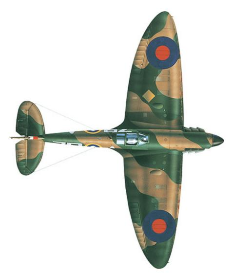
An aerial view of this Battle of Britain Spitfire Mk IA reveals the classic tapered wing of the type, as well as the yellow gas detection patch applied on the port wing in summer 1940.
