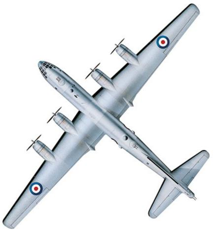
A top view of the Washington B.Mk 1 reveals the slender wing, designed to withstand massive loading and maximise cruise performance. Fowler flaps generated extra lift at low speed.
