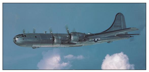
Renton-built B-29A-5-BN serial 42-93869 seen soon after leaving the production line. The huge Wright Duplex Cyclone engines drove 5.05m (16ft 7in) diameter four-bladed propellers.
