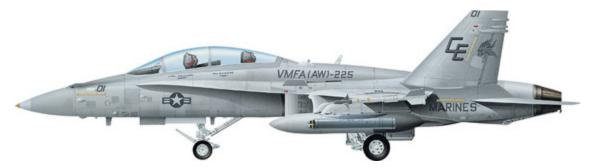
An F/A-18D of the U.S. Marine Corps' VMFA(AW)-225 armed with 127mm (5in) Zuni unguided rockets underwing, used for target-marking purposes in the forward air controller (airborne) role.
