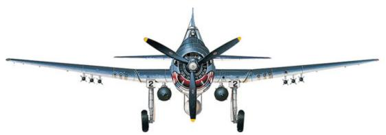
A frontal view of the fully armed VF-27 F6F-5 reveals details of its weaponry, including machine guns in the wing, bombs on the inner underwing stations and rocket projectiles outboard.
