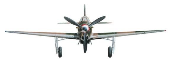
A frontal view of the Yak-9D. The fighter utilized a lightweight armament comprising a single 20mm (0.79in) ShVAk firing through the spinner and one 12.7mm (0.5in) UBS machine gun.
