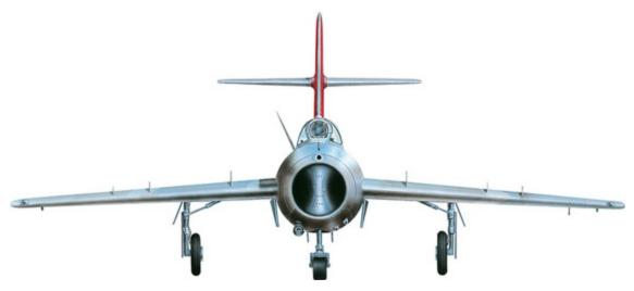
In its day-fighter versions, the MiG-17 packed a punch with a nose armament of one 37mm (1.45in) N-37D cannon to starboard, and single 23mm (0.9in) NS-23 cannon on the port side.
