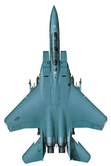
The F-15E carries conformal fuel tanks on the sides of the fuselage. Each holds 2737 litres (723 U.S. gal) of fuel, and is fitted with three stub pylons for attaching weapons.
