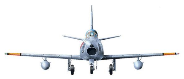
In the neat undercarriage of the Sabre, the nosewheel unit retracted backwards to lie in the forward fuselage, while the mainwheels retracted inwards to lie in the fuselage.
