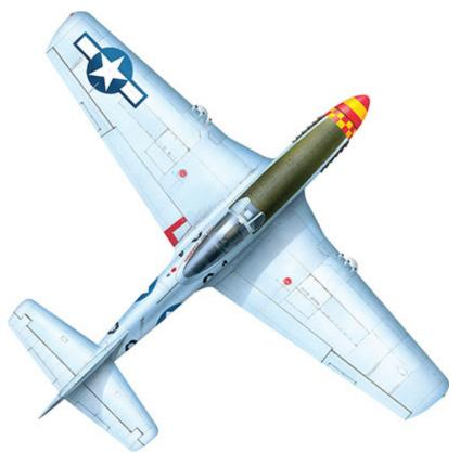
Although capable of a high rate of fire, with six 12.7mm Browning machine guns in the wing the P-51K was less heavily armed that the P-47, or the various cannon-armed fighters of the RAF.
