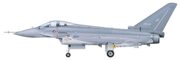
DA.2, serial ZH588, was the first British prototype, and is seen armed with AIM-9L Sidewinder missiles. The aircraft was first flown at Warton in April 1994 and is now at the RAF Museum.
