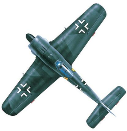
A plan view of Schneider's Fw 190A-1 demonstrates the excellent view provided by the onepiece, rear-sliding canopy. Powerplant for the A-1 was the 1193kW (1600hp) BMW 801C-1.
