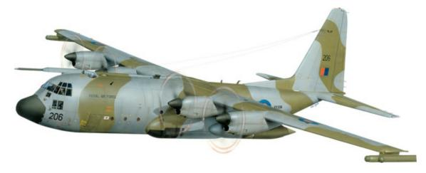
The C-130K version was built specifically for British use on the basis of the C-130H, and entered RAF service as the Hercules C.Mk 1, seen here on strength with the Hercules Wing at RAF Lyneham in 1990. This is a C.Mk 1P sub-variant with an inflight refuelling probe above the cockpit.
