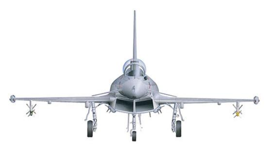
The twin 'chin' engine intakes have a hinged lower lip ('varicowl') to ensure good performance at all speeds and angles of attack. An ogival splitter plate removes boundary layer airflow and feeds the engines with clean, fast-moving air.
