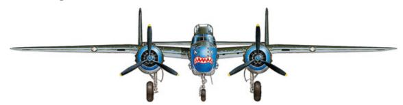
A front view of the B-25J from the 499th 'Bats Outa Hell'. The aircraft, which carried the individual name 'Betty's Dream', was fitted with a total of 18 guns, including 12 in the nose.
