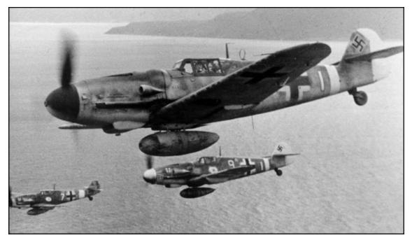
Operating from an airfield in Greece, Bf 109G-6s of 7./JG 27 patrol over the Adriatic Sea. The two aircraft to the rear are equipped with tropical filters and underwing cannon gondolas.
