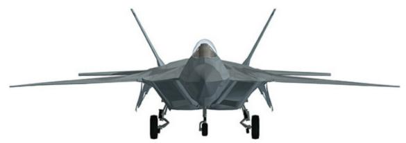
The Raptor's agility allows it to make very tight turns, and exploit post-stall manoeuvring capabilities, flying at sustained angles of attack of more than 60 degrees while retaining some roll control.
