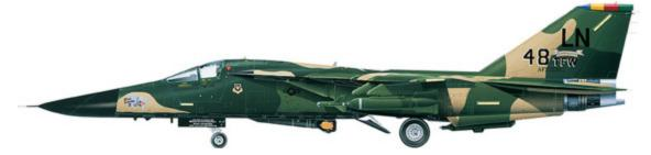
F-111Fs of the 48th TFW were employed almost exlusively to drop laser-guided bombs during Desert Storm, in this case 907kg (2000lb) GBU-24 Paveway IIIs with penetrator warheads.
