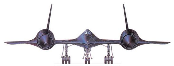
The frontal aspect of the SR-71A was dominated by its huge engine nacelles, blended into the wing leading edge, and the broad chines blending the fuselage into the leading edges.
