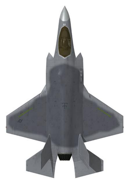
The F-35B, which is replacing the AV-8B and F/A-18 with the USMC, is capable of STOVL operation thanks to its shaft-driven Rolls-Royce LiftFan propulsion system and an engine that can swivel 90 degrees when in short take-off/vertical landing mode. The F-35B has a smaller internal
