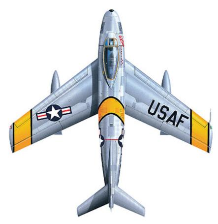
Last of the fighter line from North American production was a dedicated fighter-bomber, the F-86H, with a more powerful J73 engine contained within a much-redesigned fuselage, additional fuel capacity and nuclear-weapons capability. A total of 477 were built.
