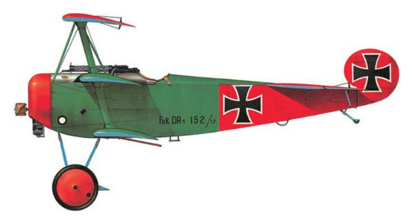
A side view of Dr.I 152/17 reveals the characteristic slab-sided fuselage, strut-braced tailplane and fixed landing gear. A key attribute of the *Dreidecker* was its simple, low-cost construction.
