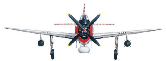
A frontal view of the 527th FS P-47D reveals the external stores, comprising 1000lb (454kg) bombs underwing and one of the nine different types of drop tank, carried on the centreline.
