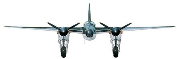
Frontal view of a Mosquito B.Mk IV Series II light bomber, which introduced various refinements including extended nacelles, enlarged tailplane and flame dampeners on the exhausts.
