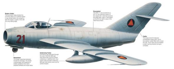
This non-afterburning MiG-17 was flown by Lt Bomba of the Mozambique Air Force when he defected to South Africa in 1980, where the fighter was tested before being returned to Mozambique.
