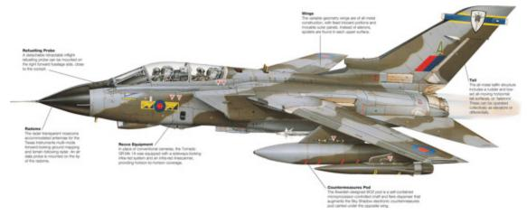
A Tornado GR.Mk 1A of the RAF's No.13 Squadron, based at Marham, Norfolk, in the 1990s. The GR.Mk 1A version retained virtually the full air-to-ground capability, although the twin cannon were deleted to make space for reconaissance equipment.
