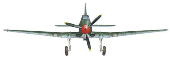
A frontal view of the II-10. Powered by a Mikulin AM-42 driving a three-bladed propeller, the II-10 demonstrated greatly enhanced performance compared to the II-2.
