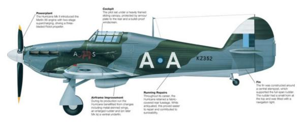
A total of 4711 Mk IICs had been completed when production came to an end in September 1944. Equipped with a four-cannon wing and bomb racks, it was the most widely deployed version.
