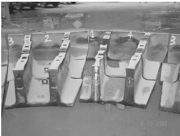
Fig. 6. Pulp lifter wear demonstrating slurry backflow.
