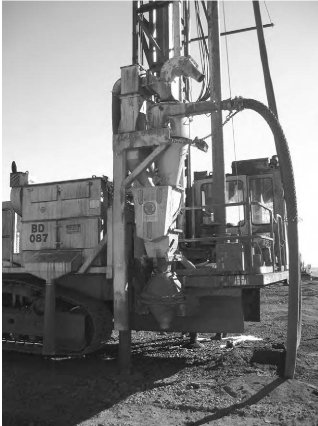
Fig. 4. Automatic sample extraction system mounted on a reverse-circulation blast-hole drill rig, which utilizes a cone divider for sample division.
