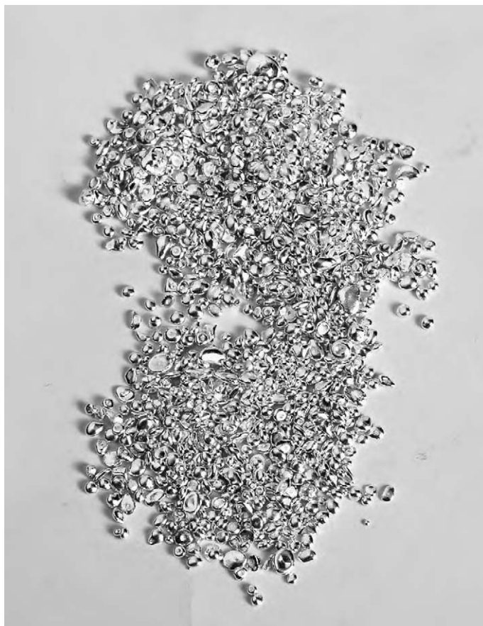
Fig. 5. Silver granules as used in the anode baskets of the HSSE plant.
