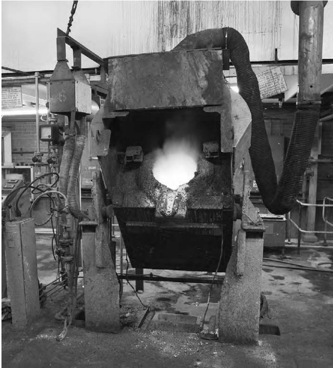
Fig. 2. Refining furnace in the Miller refining circuit.
