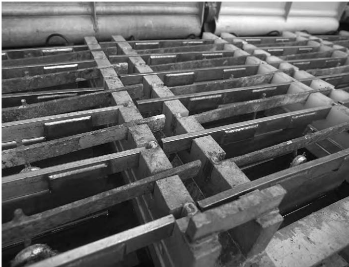
Fig. 10. Electrolytic cells showing the titanium cathode plates.
