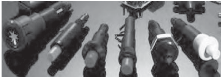
Figure 2-3 Piezoelectric PZT-based gas igniters. When the piezoelectric material is stressed (by applying a pressure) a voltage develops and a spark is created between the electrodes. (Courtesy of Morgan Electro Ceramics, Inc.)
