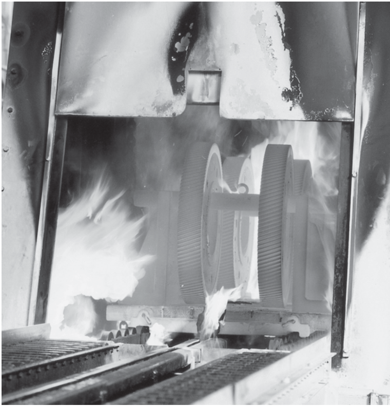
Figure 5-1 Furnace for heat treating steel using the carburization process. (Courtesy of Cincinnati Steel Treating.)
