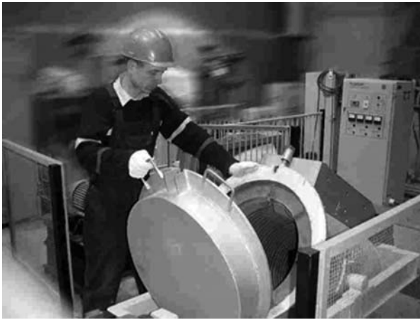
Figure 19.10 An installation for thermo-diffusion galvanizing (sherardizing): general view while container is being charged.
