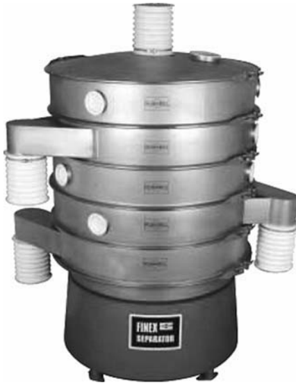
Figure 11.23 Tetradecks Russel Finex sifter. Courtesy of RusselFinex Inc.
