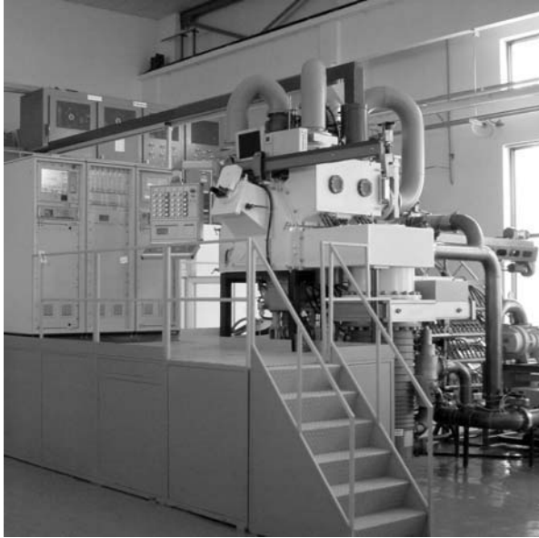
Figure 4.23 Installation UE-204 of the EO Paton Electric Welding Institute International center for electron beam technologies used for electron beam evaporation and following physical vapor deposition in a vacuum and the manufacture of various materials and components. Courtesy of Professor BA Movchan.
