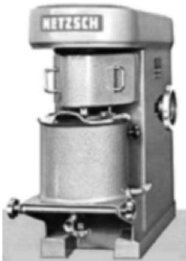
Figure 3.5 Laboratory batch NETZSCH attritor PE 5. Courtesy of NETZSCH Incorporated.
