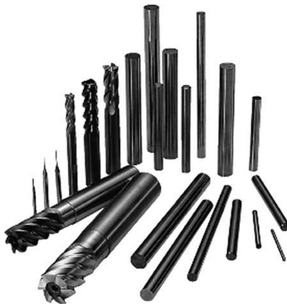
Figure 4.28 Selection of nanometric WC-Co solid carbide end mills, drills and rods. (Source: Ref 24)
