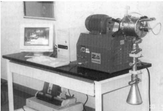
Figure 3.6 Laboratory Simoloyer CM01-051 attritor in horizontal performance. (Source: Ref 11)
