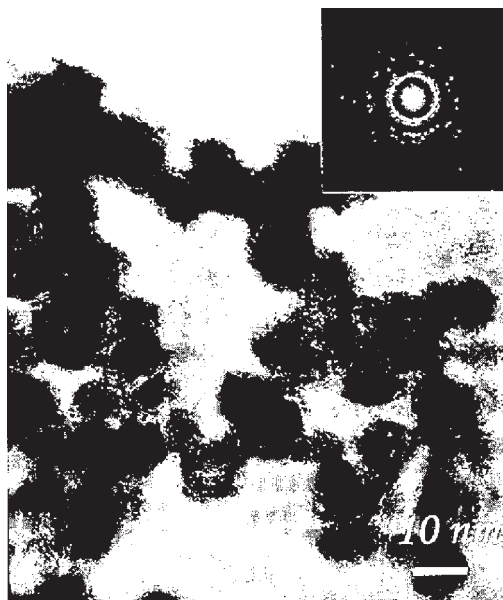
Figure 4.16 TEM image and selected area electron diffraction pattern of nickel particles produced with ethylene as photosensitizer. (Source: Ref 26)
