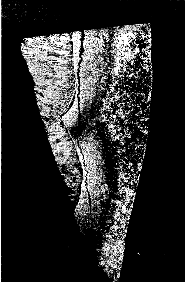
Fig. 21 Stress relief cracking initiating in coarse grained HAZ.
