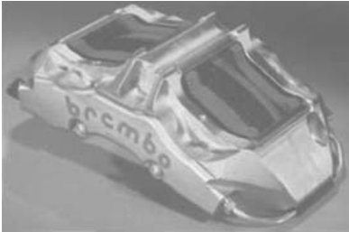
Figure 10.14 An Al-Be composite disk brake caliper for a Ferrari Formula 1 racing car (Marder, 1997).
