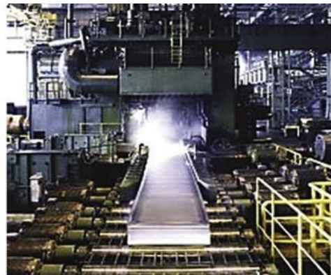
Elastic design, avoiding plasticity, ensures that the cabin of the car does not deform in a crash. Plasticity absorbs the energy of impact, and allows metals to be shaped and polymers to be moulded. (Image of crash testing courtesy AutoNews; image of hot rolling courtesy of Tanis Inc., Delafield, WI)
