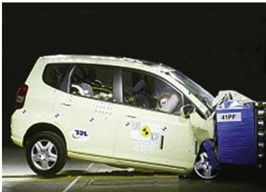
Elastic design, avoiding plasticity, ensures that the cabin of the car does not deform in a crash. Plasticity absorbs the energy of impact, and allows metals to be shaped and polymers to be moulded. (Image of crash testing courtesy AutoNews; image of hot rolling courtesy of Tanis Inc., Delafield, WI)
