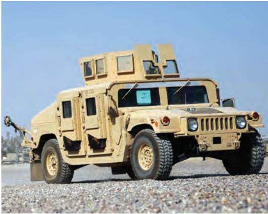
FIGURE 1-2 Up-armored high-mobility multipurpose wheeled vehicle (HMMWV, or Humvee). SOURCE: Available at <http://www.militaryfactory.com/armor/imgs/hmmwv-m1114uah.jpg>. Courtesy of U.S. DoD.
