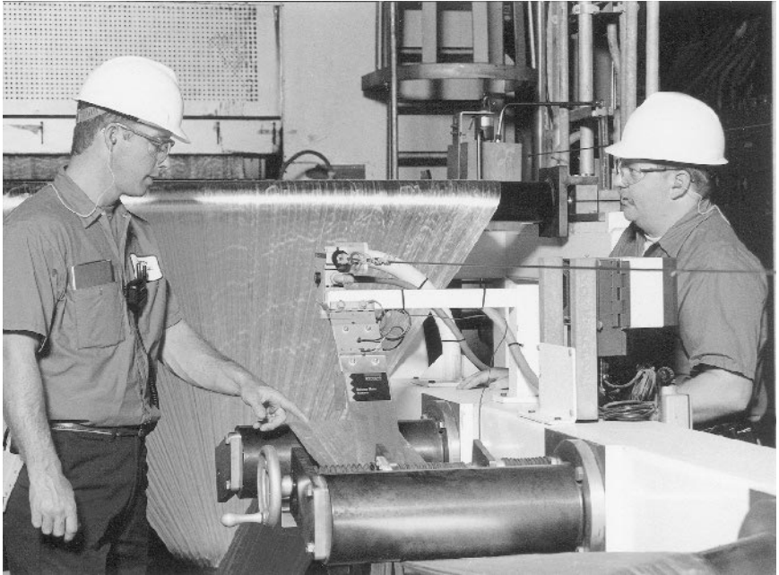
4.4 Inspecting lyocell tow as it is condensed after drying and prior to crimping. (Reproduced by courtesy of Acordis.)
