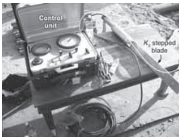
FIGURE 10.35 The K_0 stepped blade with control unit and other accessories (courtesy of Professor David White, Iowa State University).
