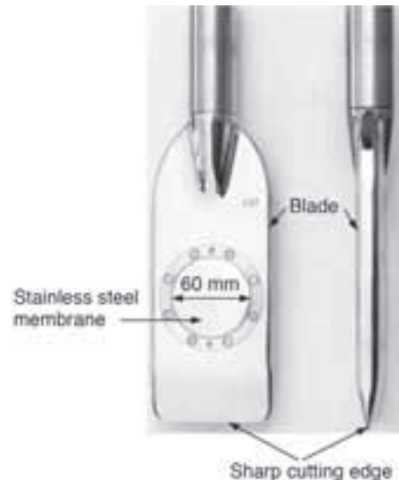
FIGURE 10.31 The flat dilatometer: front and side views (adapted from Marchetti et al. 2001).
