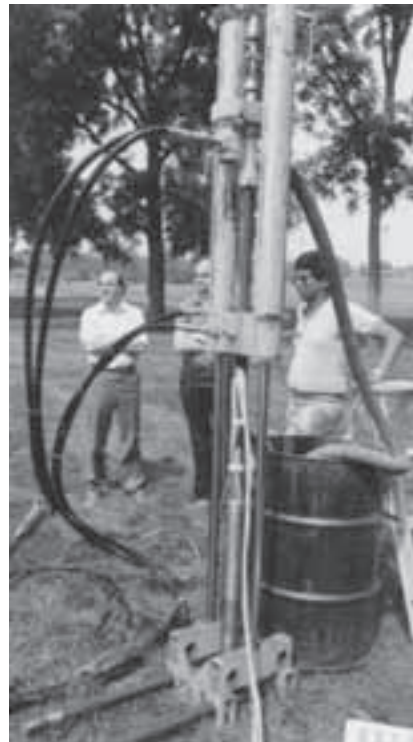
FIGURE 10.28 Pressuremeter test apparatus arrangement at the test site.
