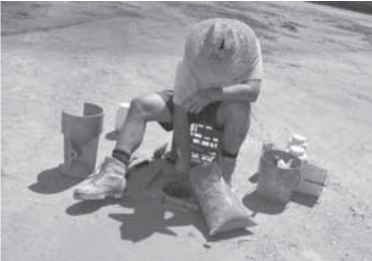
FIGURE 10.39 Determination of in situ unit weight by sand cone method.
