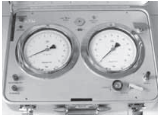
FIGURE 10.32 Control unit of the DMT (after Marchetti et al. 2001).
