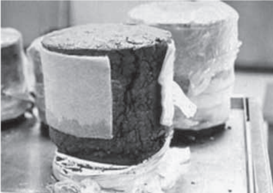
FIGURE 9.8 Three-dimensional swell test results in sulfate-laden, lime-treated soil.
