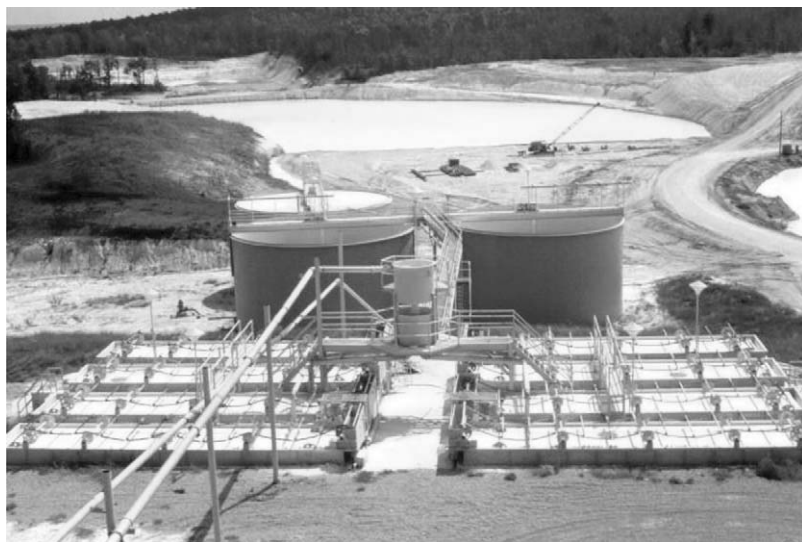
Fig. 10.1.12. Mining and degritting operation in a kaolin mine, Georgia USA.
