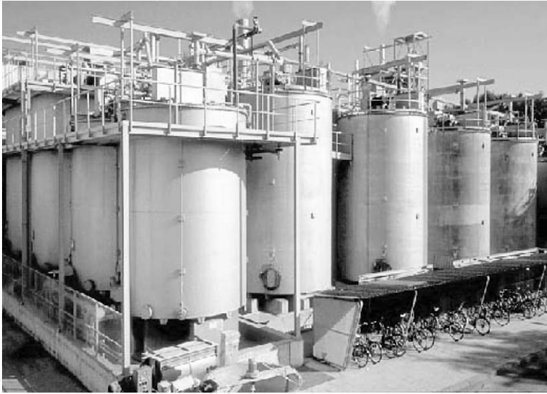
Fig. 10.1.21. Reaction vessels for acid-activation of bentonite (Courtesy N. Schall, Süd-Chemie AG, Germany).
