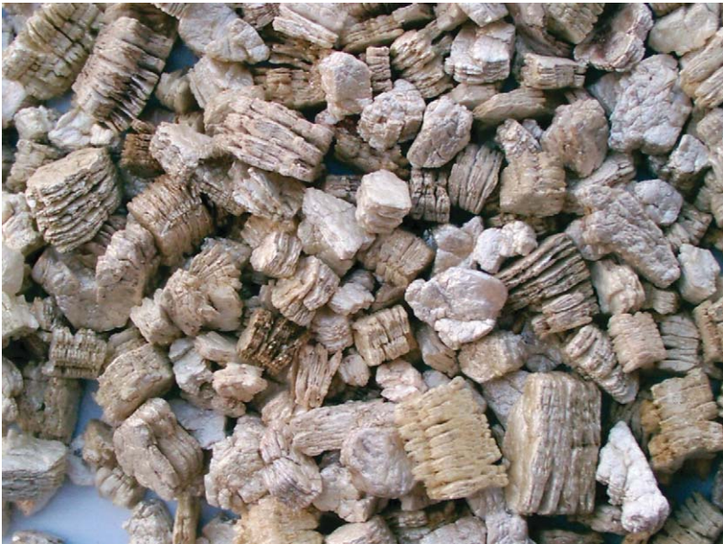
Fig. 10.1.9. Shock-heated expanded vermiculite flakes (Courtesy K. Beneke, University Kiel).
