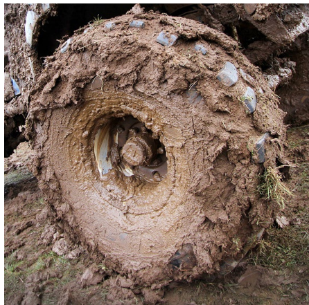
Figure 5A-24: Adhesion of Organic Soil to a Tire.
