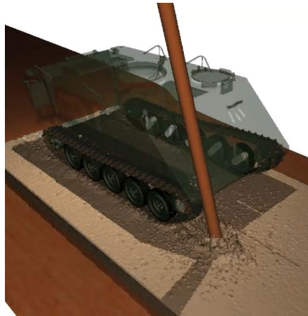
Figure 5A-30: Soil Embedded Large Tree Stem or Pole Interacting with the Vehicle and the Soil.
