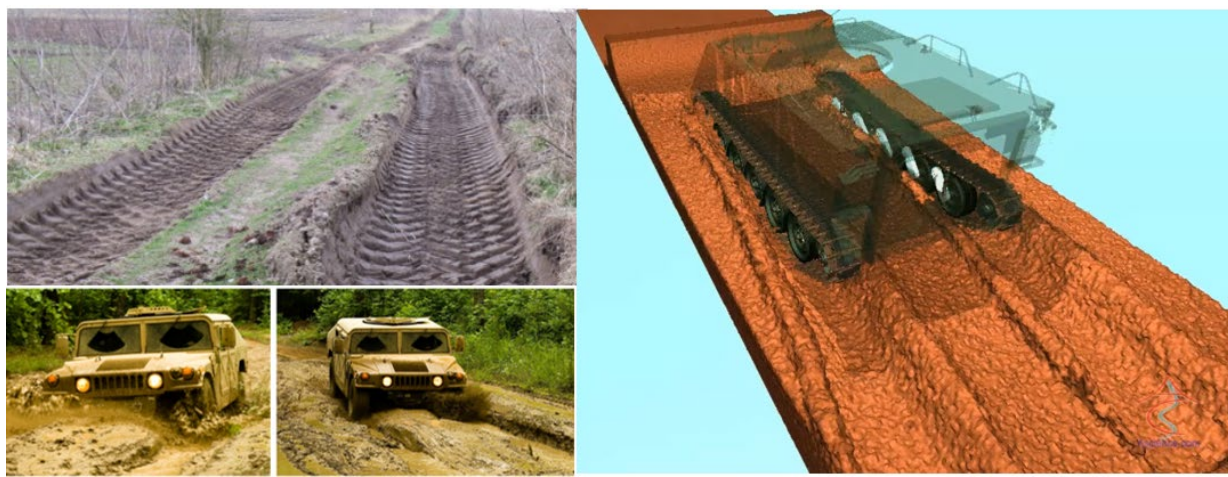
Figure 5A-12: Terrain Damage Caused by a Vehicle Measured by the Rut Depth, Width, Shape and Side Wall Height.
