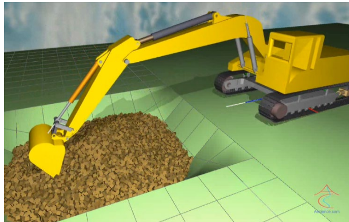
Figure 5B-60: Snapshot of a Backhoe Digging through Non-Cohesive Sand Type Soil Modeled Using Cubical Rigid Body DEM Particles.
