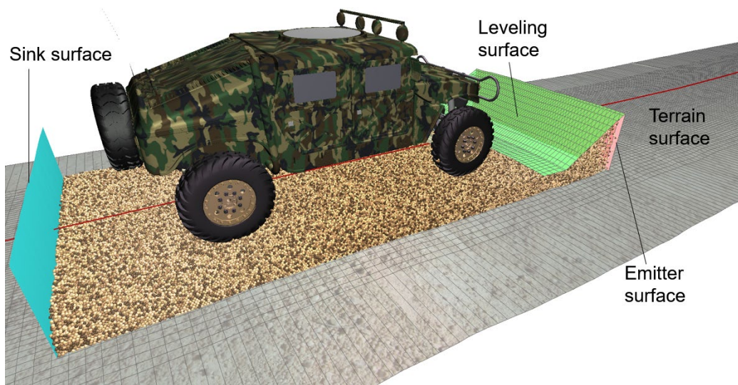
Figure 5B-32: Moving DEM Complex Topography Terrain Patch Modeled Using an I-J Ordered Quadrilateral Grid Representing the Terrain's Surface, an Emitter Surface, a Leveling Surface, and a Sink Surface.
