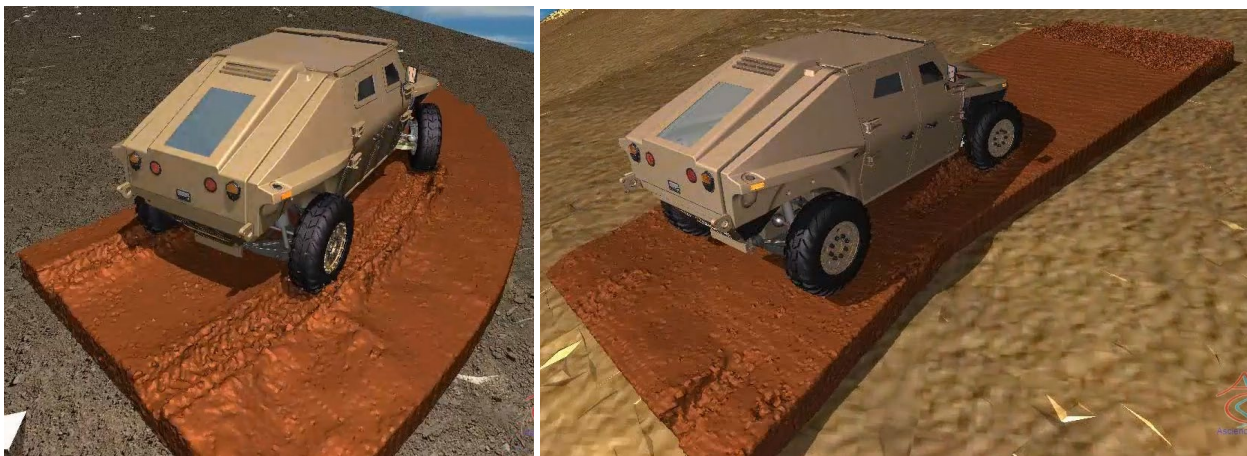
Figure 5B-33: Snapshots of the Moving DEM Complex Topography Terrain Patch in Typical Vehicle Mobility Simulations: 90° Turn (Left) And Going Down A Slope (Right) On Rough Soft Soil Terrains.
