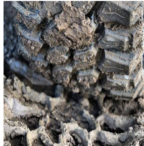
Figure 5A-6: Soil Adhesion to a Tire Caused by the Soil Particles-Rubber Forces.
