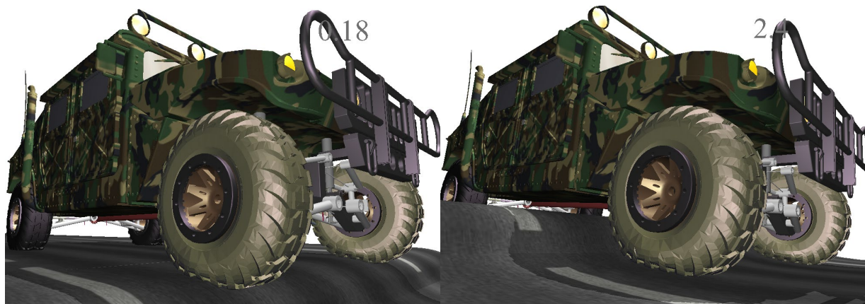
Figure 5B-44: Snapshots of the Multibody Vehicle Model with Finite Element Flexible Tires Displayed using the Tread Proxy Contact Surface. The Tire is Going over Hard Pavement.
